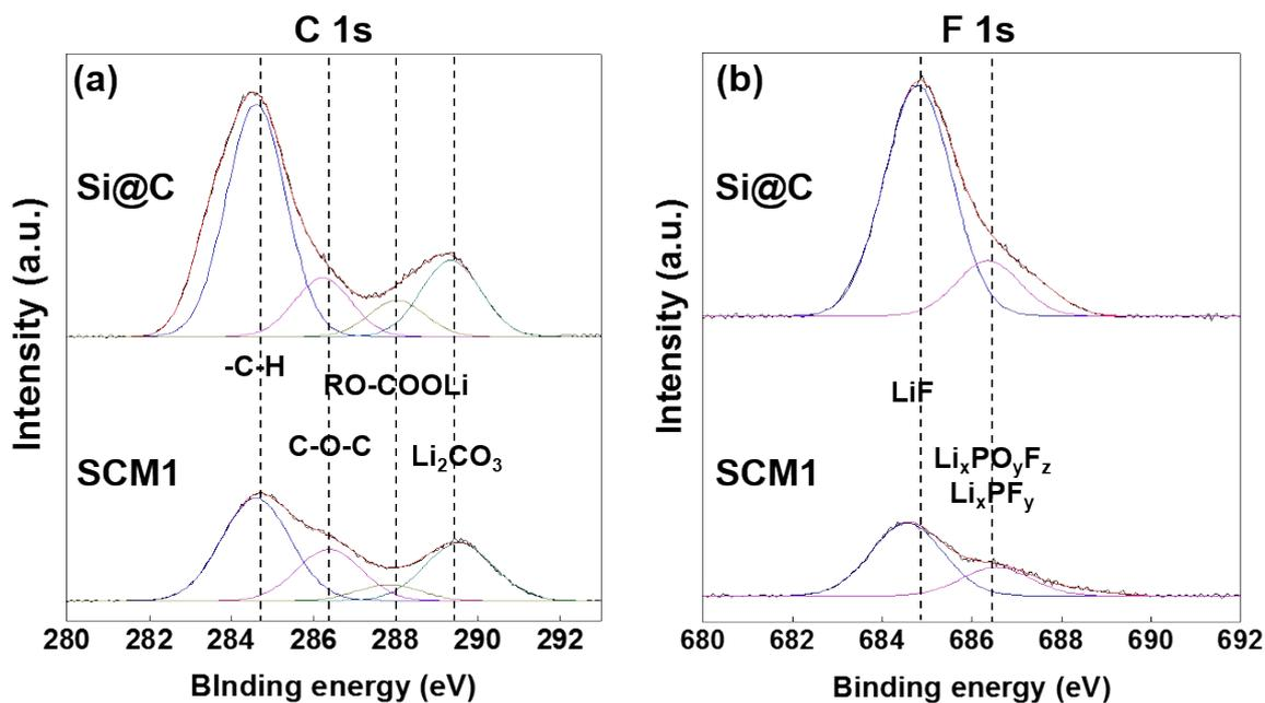
**Figure S11.** XPS spectra of Si@C and SCM1 electrodes of (a) C 1s (b) F 1s after 100 cycles based on various current densities: 1<sup>st</sup> = 100 mA/g, 2<sup>nd</sup> = 200 mA/g, and 3<sup>rd</sup> and following = 500 mA/g.
