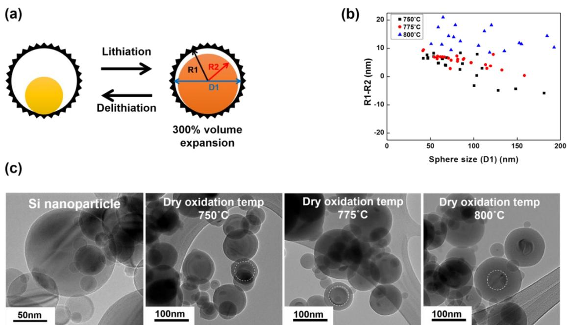
**Figure S1.** (a) Illustration of Si core volume expansion of SCM yolk-shell structure. (b) The Si volume expansion calculation scatter diagram for various dry oxidation temperatures. (c) HR-TEM image of Si nanoparticles and Si@SiO<sub>2</sub> nanoparticles for various the dry oxidation temperatures.
