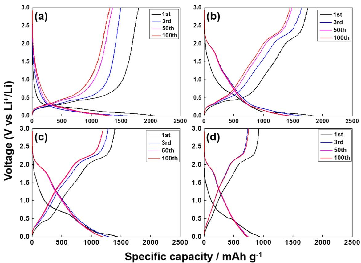
**Figure S8.** Charge-discharge profile of (a) Si@C, and SCM electrodes: (b) SCM1, (c) SCM3, and (d) SCM5.
