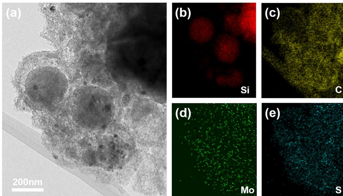
**Figure S12.** (a) TEM image of SCM1 electrodes after 100 cycles and its elemental mapping for (b) Si, (c) C, (d) Mo, and (e) S.
