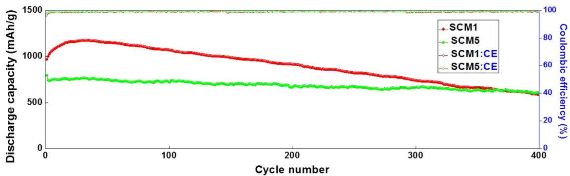
**Figure S5.** Long-term cyclic test of SCM1, SCM5 at a current density of 2000mA/g.
