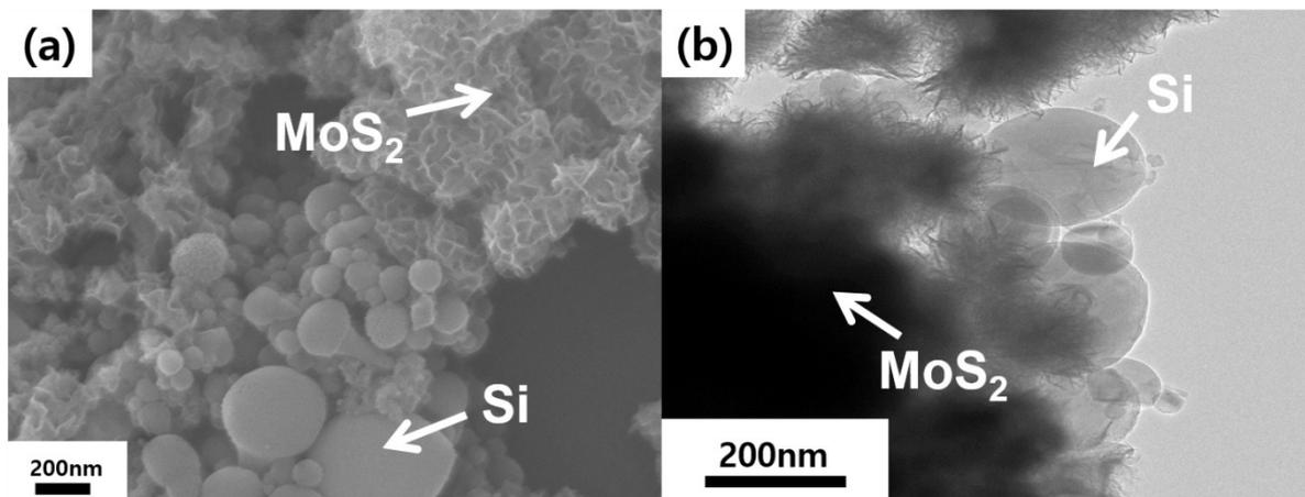
**Figure S2.** (a) FE-SEM image, (b) HR-TEM image of synthesized of Si/MoS<sub>2</sub> nanoparticles without a PDA coating on the Si@SiO<sub>2</sub> surface.
