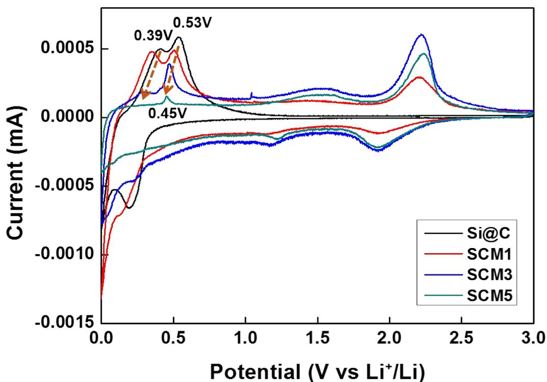
**Figure S7.** Cyclic voltammetry at 5<sup>th</sup> cycle of Si@C, SCM1, SCM3 and SCM5 at a scan rate of 0.1 mV/s.
