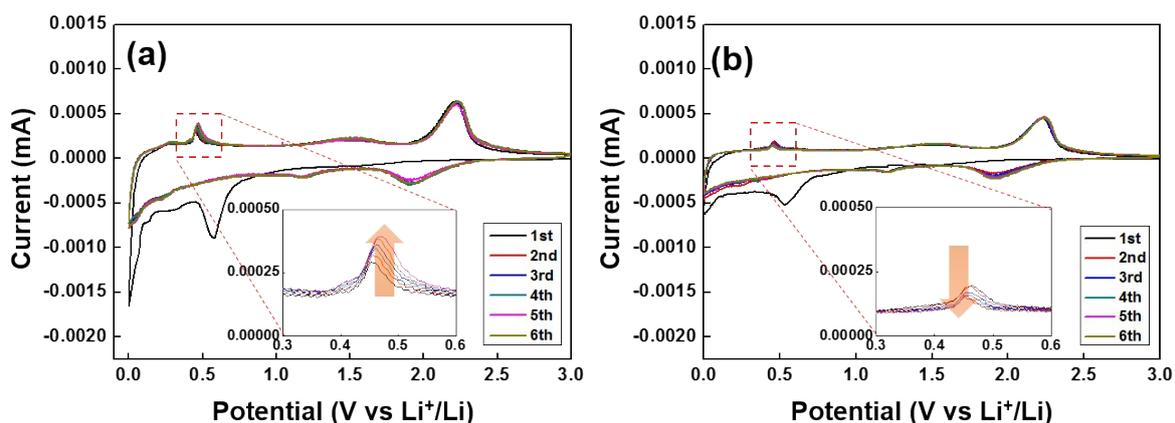
**Figure S6.** Cyclic voltammetry of (a) Si@C, (b) SCM1 at a scan rate of 0.1 mV/s.
