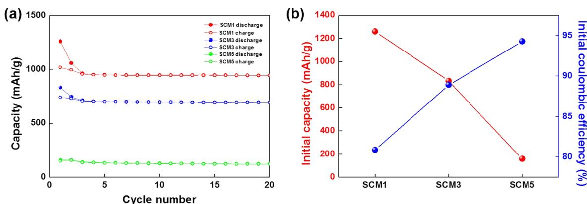
**Figure S9.** (a) Cycling performance and (b) initial coulombic efficiency of SCM1, SCM3 and SCM5 at 0.01 ~ 1.5V (Li/Li<sup>+</sup>) range based on various current densities: 1<sup>st</sup> = 100 mA/g, 2<sup>nd</sup> = 200 mA/g, and 3<sup>rd</sup> and following = 500 mA/g.
