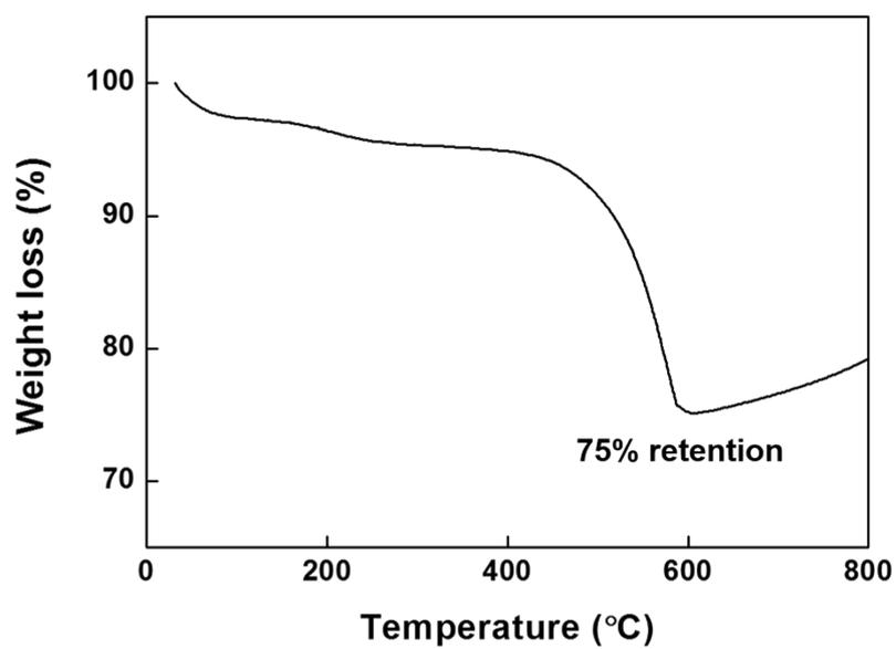
**Figure S3.** Thermogravimetric Analysis (TGA) results of the Si@C sample. The sample was heated under the air.
