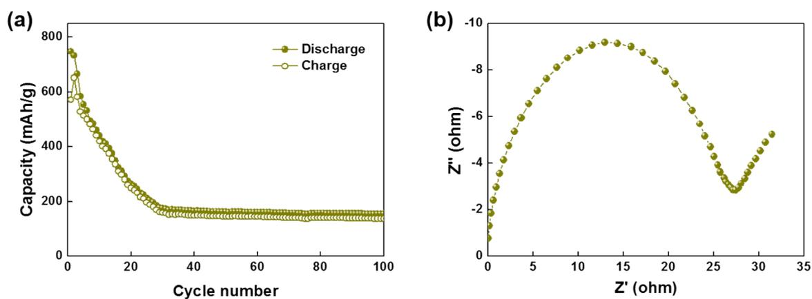
**Figure S10.** (a) Cycling performance and (b) EIS plot of bare MoS<sub>2</sub> nanoparticle based on various current densities: 1<sup>st</sup> = 100 mA/g, 2<sup>nd</sup> = 200 mA/g, and 3<sup>rd</sup> and following = 500 mA/g.
