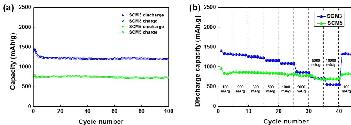
**Figure S4.** (a) Cycling performance and coulombic efficiency of SCM3 and SCM5 based on various current densities: 1<sup>st</sup> = 100 mA/g, 2<sup>nd</sup> = 200 mA/g, and 3<sup>rd</sup> and following = 500 mA/g. (b) Rate capabilities of SCM3, SCM5.
