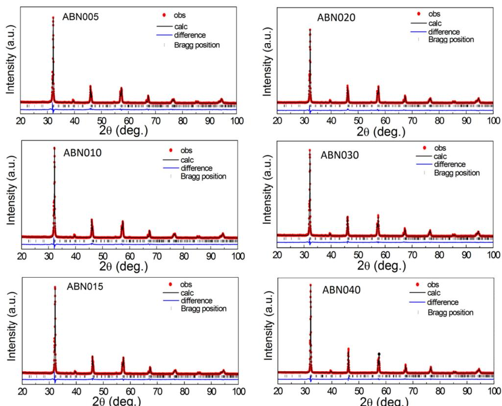
Fig. S1. Fitted X-ray diffraction profiles for crushed ABNx ceramic powders.
