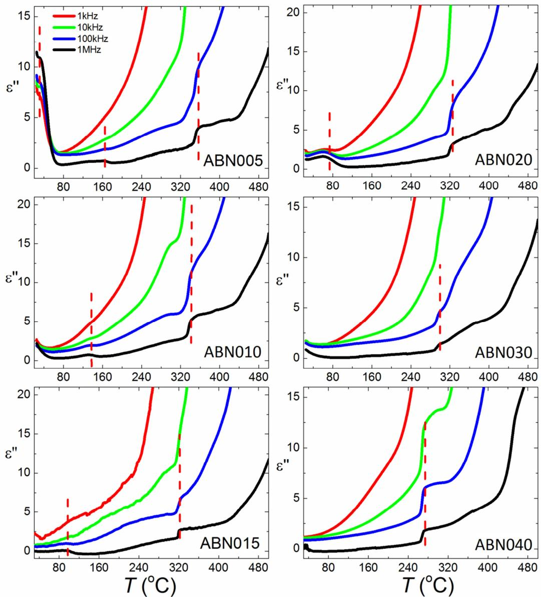
Fig. S2. Temperature dependence on heating of imaginary ( $\epsilon''$ ) part of dielectric permittivity in ABNx ceramics.
