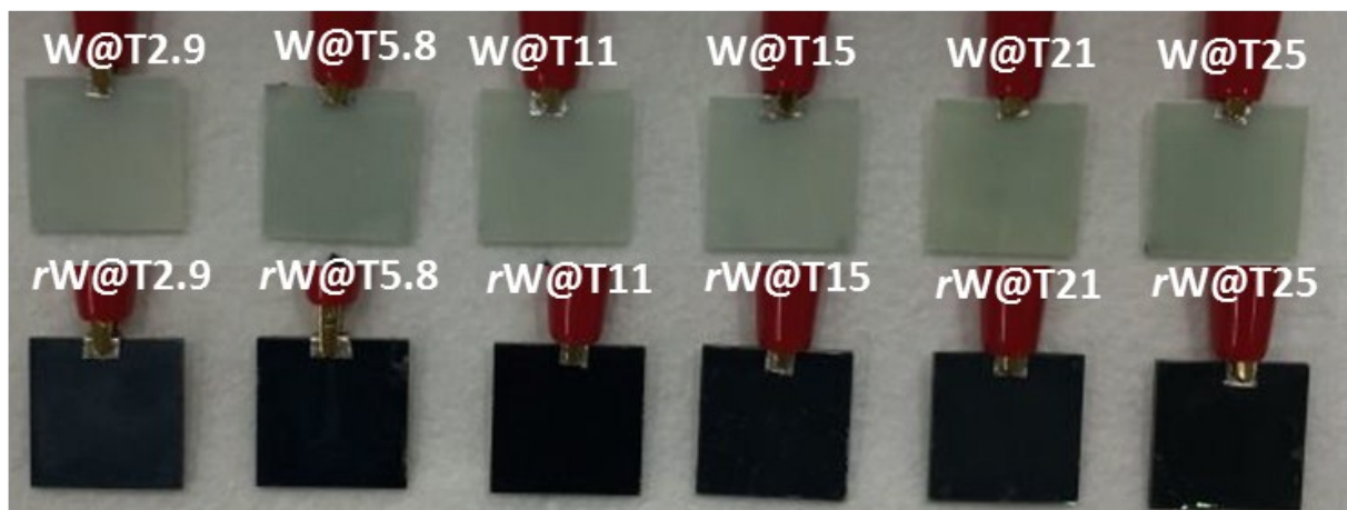
Figure S11. Digital photographs of all the obtained \text{WO}_3@TiO_2 and \text{WO}_{3-x}@TiO_{2-x} core-shell nanosheets samples.
