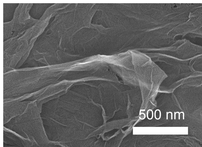
**Figure S10.** SEM image of synthesized reduce graphene oxide (rGO).
