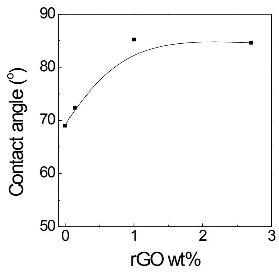
**Figure S4.** Change of the contact angle on PRC/PSCs, as function of rGO contents.
