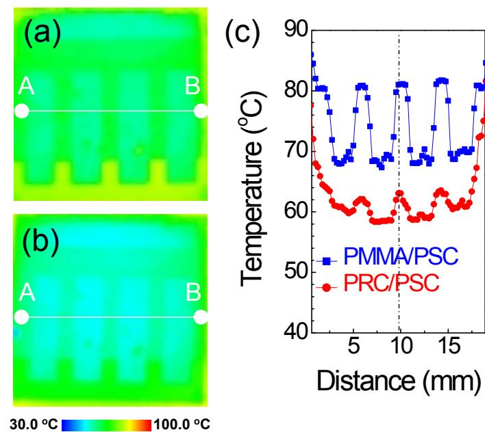
**Figure S7.** Infrared thermal camera image of (a) the PMMA layer coated perovskite solar cell and (b) the PRC layer coated perovskite solar cell, (c) surface temperature variation of PMMA/PSC and PRC/PSC on the hot plate at 93 °C.
