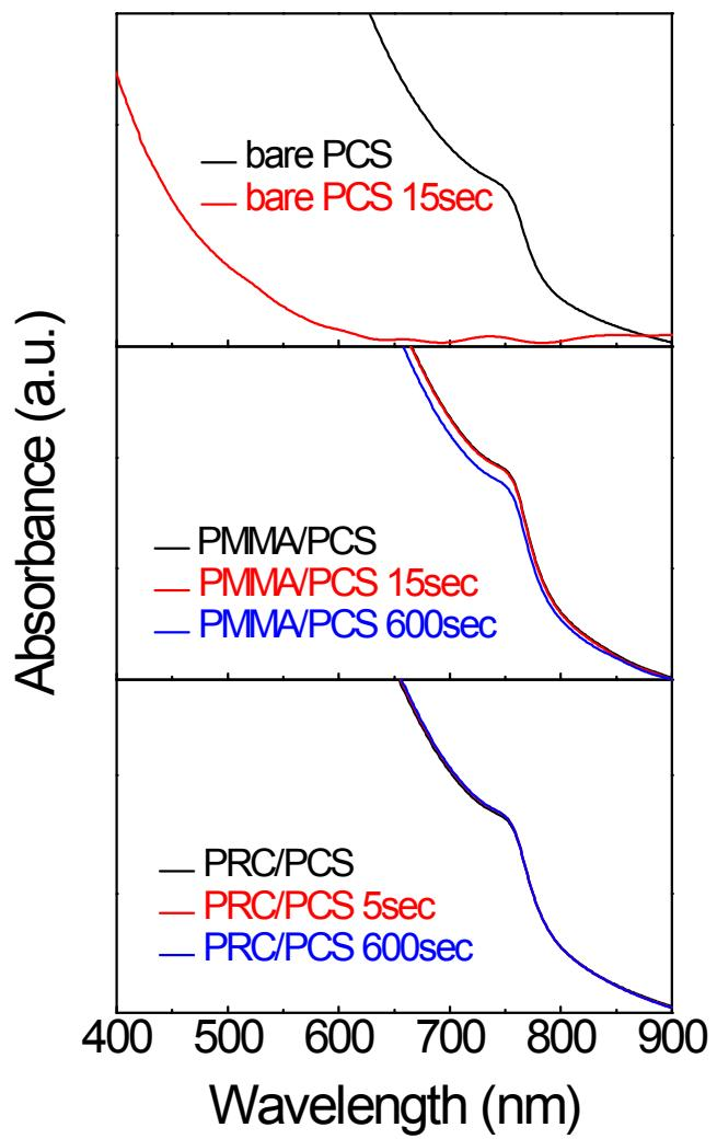
**Figure S5.** Absorbance of bare PSC, PMMA/PSC and PRC/PSC after samples were submerged in water for 15 sec and 600 sec.
