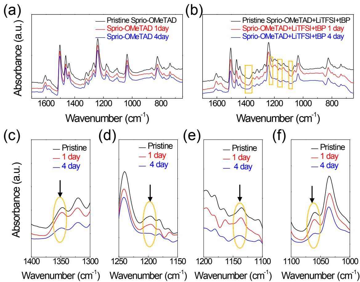
**Figure S8.** ATR-FTIR spectra of (a) the undoped spiro-OMeTAD and (b) spiro+LiTFSI+tBP films after aging at 90 °C. Magnified regions of (c, d, e, f) highlighting the differences.
