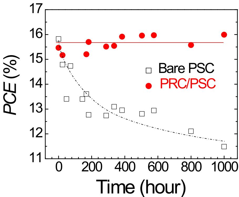
**Figure S9.** Long term stability of a bare PSC and PRC/PSC as a function of storage time in air for 1000 h (Humidity: ~40 %, Temperature: ~35 °C).
