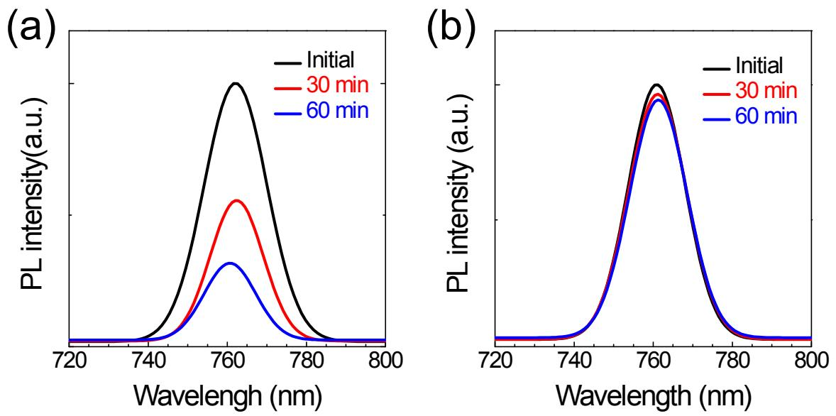
**Figure S6.** Steady-state Photoluminescence (PL) of the perovskite films (a) perovskite/TiO<sub>2</sub>/FTO, (b) PRC/perovskite/TiO<sub>2</sub>/FTO film with aging time in very humid condition, under 560 nm excitation
