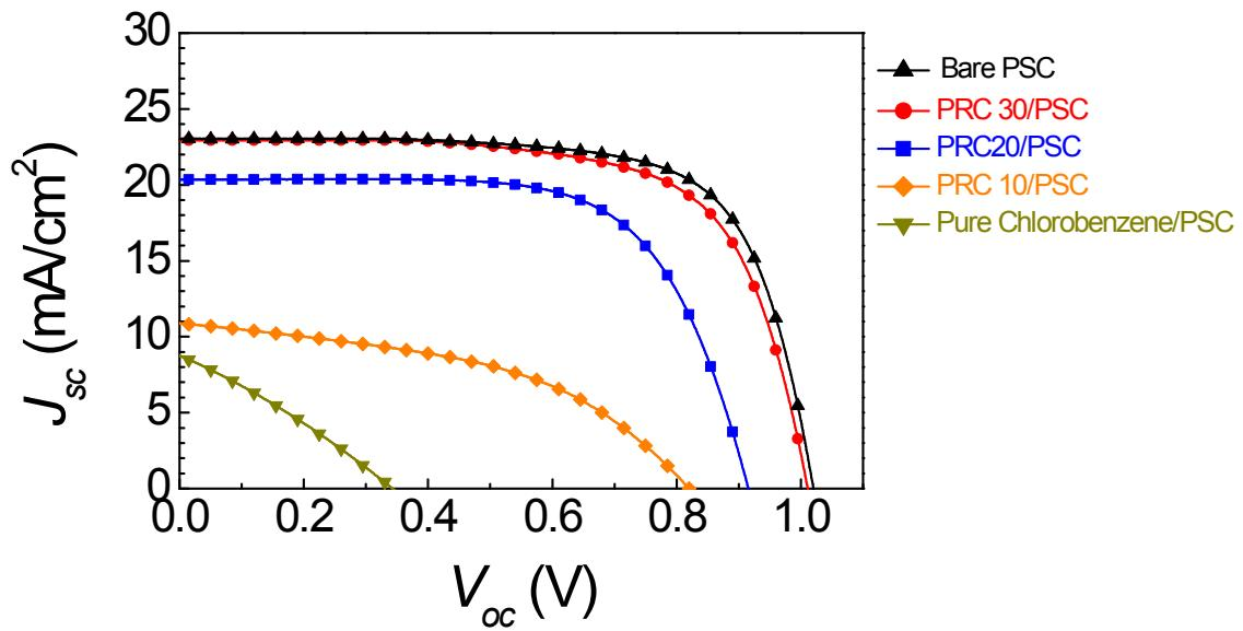
**Figure S2.**  $J$ - $V$  curves of the perovskite solar cells coated with solutions containing different amounts of PMMA in chlorobenzene.
