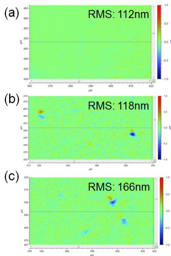
**Figure S1.** A change in the surface roughness of (a) pure PMMA, (b) PRC (rGO: 1wt%), and (c) PRC (rGO: 2wt%)
