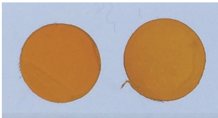
Figure S6. 8 mm discs of F2 photographed after immersion for 24 hours at room temperature in a 10^{-3} M solution of mercury nitrate monohydrate (left) and methylmercury(II) chloride (right). Due to the insolubility of methylmercury(II) chloride in pure water, the media in this case was MeOH:water-buffer-pH 2.2 (10/90 v/v).
