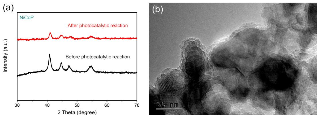
**Fig. S8** (a) The XRD patterns of NiCoP@NiCo-Pi/g-C<sub>3</sub>N<sub>4</sub> before and after photocatalytic reaction in TEOA and K<sub>2</sub>HPO<sub>4</sub> solution. (b) HRTEM image of NiCoP@NiCo-Pi/g-C<sub>3</sub>N<sub>4</sub> after photocatalytic reaction in TEOA and K<sub>2</sub>HPO<sub>4</sub> solution.
