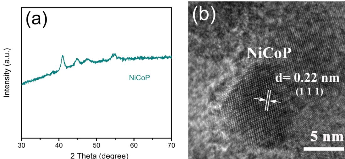
**Fig. S10** (a) XRD pattern and (b) TEM image of NiCoP particles.
