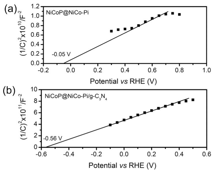
**Fig. S17** Mott-Schottky plots of NiCoP@NiCo-Pi and NiCoP@NiCo-Pi/g-C<sub>3</sub>N<sub>4</sub> in 0.5 M Na<sub>2</sub>SO<sub>4</sub> solution.
