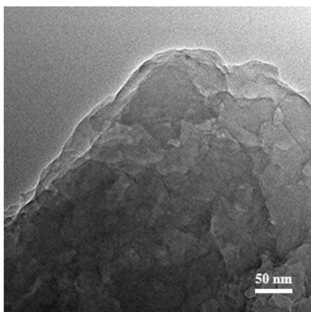
**Fig. S2** TEM image of g-C<sub>3</sub>N<sub>4</sub>.
