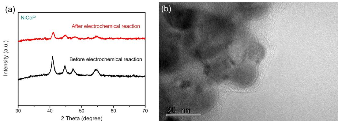
**Fig. S5** (a) The XRD patterns of NiCoP@NiCo-Pi/g-C<sub>3</sub>N<sub>4</sub> before and after electrochemical reaction in Na<sub>2</sub>SO<sub>4</sub> solution. (b) HRTEM image of NiCoP@NiCo-Pi/g-C<sub>3</sub>N<sub>4</sub> after electrochemical reaction in Na<sub>2</sub>SO<sub>4</sub> solution.
