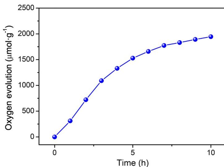
**Fig. S14** Long-time photocatalytic oxygen evolution test of NiCoP@NiCo-Pi/g-C<sub>3</sub>N<sub>4</sub>. Reaction conditions: 50 mg of photocatalysts, 80 mL of 0.02 M AgNO<sub>3</sub> aqueous solution containing 0.2 g of La<sub>2</sub>O<sub>3</sub> as a pH buffer agent, 300 W Xe lamp.
