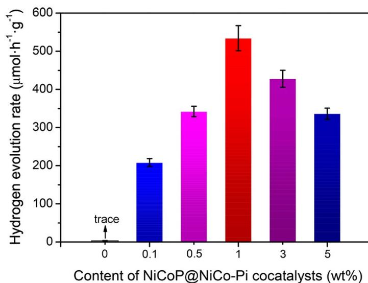
**Fig. S6** Photocatalytic hydrogen evolution rates over NiCoP@NiCo-Pi/g-C<sub>3</sub>N<sub>4</sub> with different contents of NiCoP@NiCo-Pi (0, 0.1, 0.5, 1, 3, 5 wt%). Reaction conditions: 50 mg of photocatalysts, 80 mL of aqueous solution containing 10 vol% TEOA, 300 W Xe lamp equipped with a cutoff filter ( $\lambda \geq 420$  nm).
