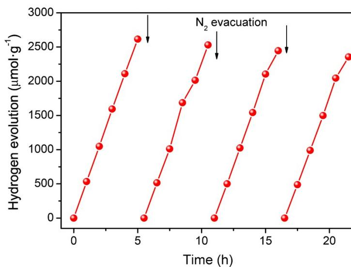
**Fig. S13** Long-time photocatalytic hydrogen evolution test of NiCoP@NiCo-Pi/g-C<sub>3</sub>N<sub>4</sub>. Reaction conditions: 50 mg of photocatalysts, 80 mL of aqueous solution containing 10 vol% TEOA, 300 W Xe lamp equipped with a cutoff filter ( $\lambda \geq 420$  nm).
