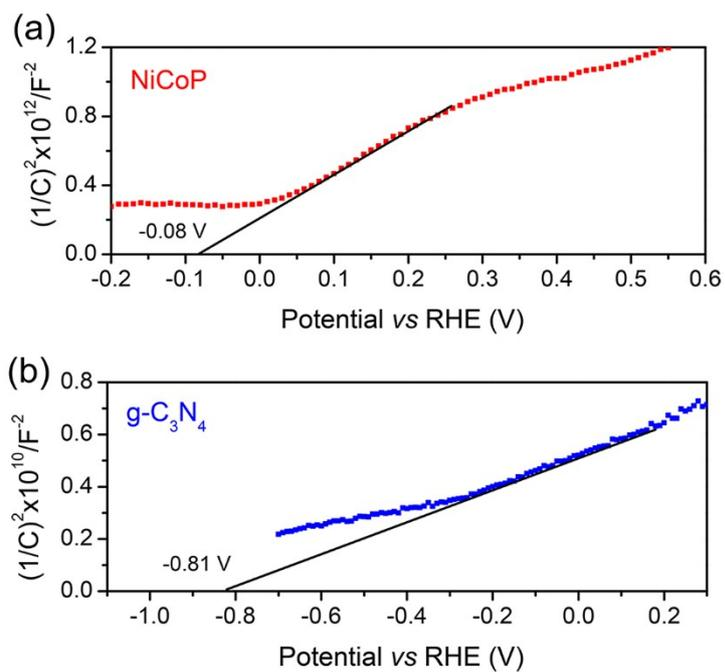
**Fig. S16** Mott-Schottky plots of NiCoP and g-C<sub>3</sub>N<sub>4</sub> in 0.5 M Na<sub>2</sub>SO<sub>4</sub> solution.
