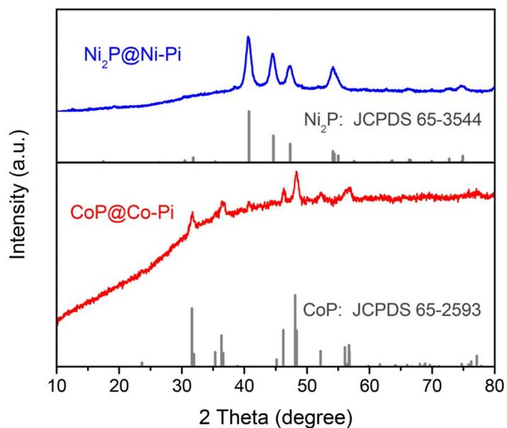
**Fig. S11** XRD patterns of  $\text{Ni}_2\text{P}@Ni\text{-Pi}$  and  $\text{CoP}@Co\text{-Pi}$  samples.
