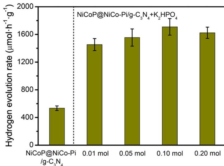
**Fig. S7** Photocatalytic hydrogen evolution rates over NiCoP@NiCo-Pi/g-C<sub>3</sub>N<sub>4</sub> with different amounts of K<sub>2</sub>HPO<sub>4</sub> in the reaction solution. Reaction conditions: 50 mg of photocatalysts, 80 mL of aqueous solution containing 10 vol% TEOA with different amounts of K<sub>2</sub>HPO<sub>4</sub>. 300 W Xe lamp equipped with a cutoff filter ( $\lambda \geq 420$  nm).
