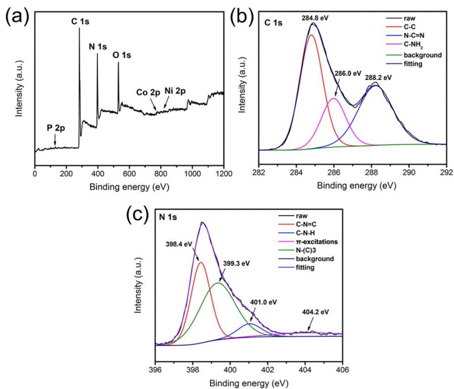
**Fig. S4** (a) The survey XPS spectrum of NiCoP@NiCo-Pi/g-C<sub>3</sub>N<sub>4</sub>. The XPS spectra of (b) C 1s and (c) N 1s.
