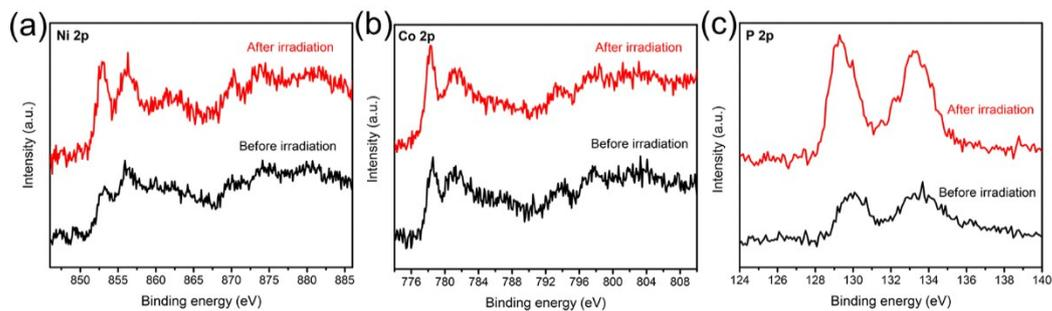
**Fig. S15** XPS spectra of (a) Ni 2p, (b) Co 2p, and (c) P 2p in NiCoP@NiCo-Pi/g-C<sub>3</sub>N<sub>4</sub> before and after photocatalytic reaction.
