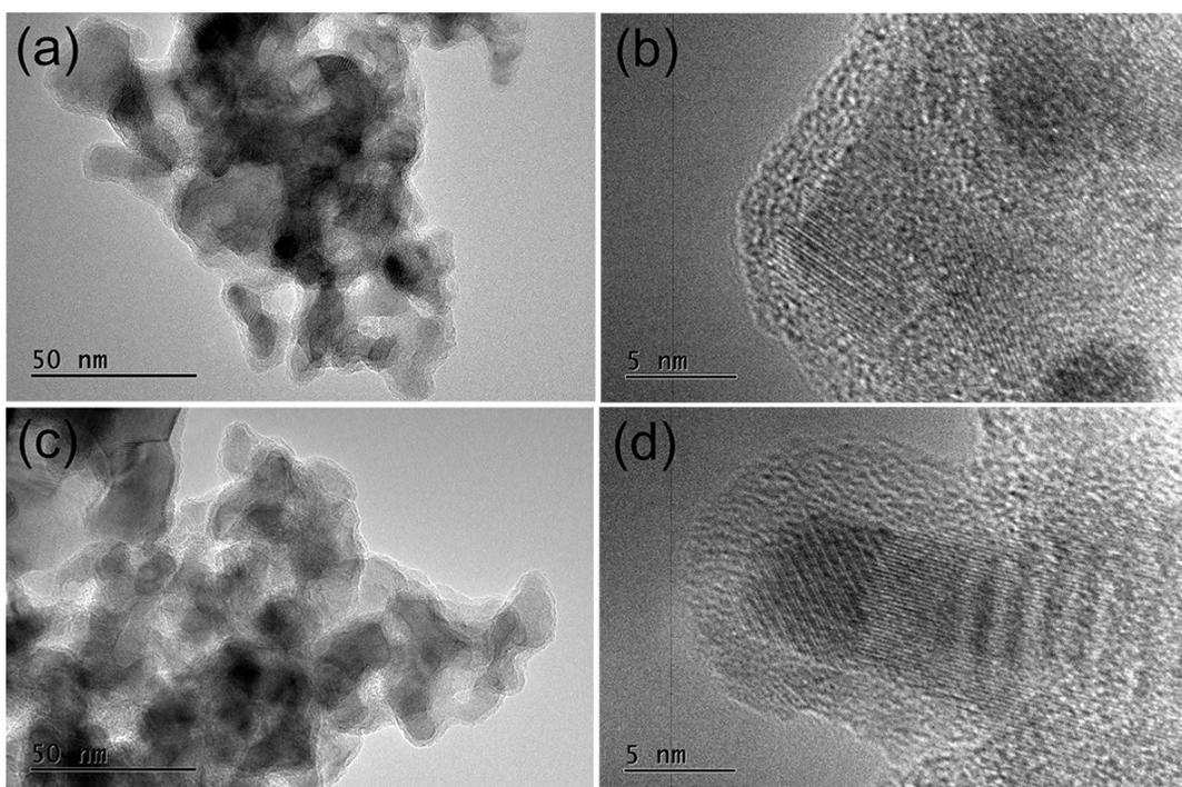
**Fig. S1** (a, b) TEM and HRTEM images of NiCoP@NiCo-Pi core/shell nanoparticles just after the solid-state reaction. (c, d) TEM and HRTEM images of NiCoP@NiCo-Pi core/shell nanoparticles after placed in the air for 3 days.
