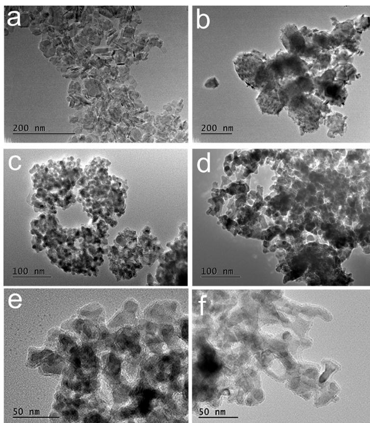
**Fig. S12** TEM images of (a)  $\text{Ni}(\text{OH})_2$  precursors, (b)  $\text{Co}(\text{OH})_2$  precursors, (c)  $\text{Ni}_2\text{P}@Ni\text{-Pi}$  nanoparticles, and (d)  $\text{CoP}@Co\text{-Pi}$  nanoparticles. (e, f) HRTEM images of  $\text{Ni}_2\text{P}@Ni\text{-Pi}$  and  $\text{CoP}@Co\text{-Pi}$  core/shell nanoparticles.
