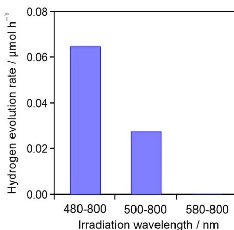
Figure S6 Dependence of the rate of H<sub>2</sub> evolution from Pt/LaOInS<sub>2</sub> on different ranges of irradiation wavelength by changing cutoff wavelength of an incident light.
