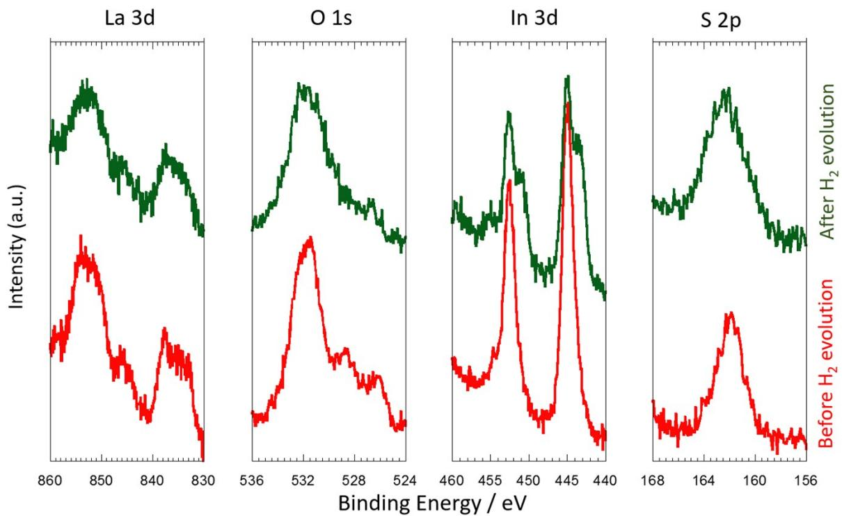
Figure S8 XPS spectra of LaOInS<sub>2</sub> (a) before and (b) after photocatalytic H<sub>2</sub> evolution.
