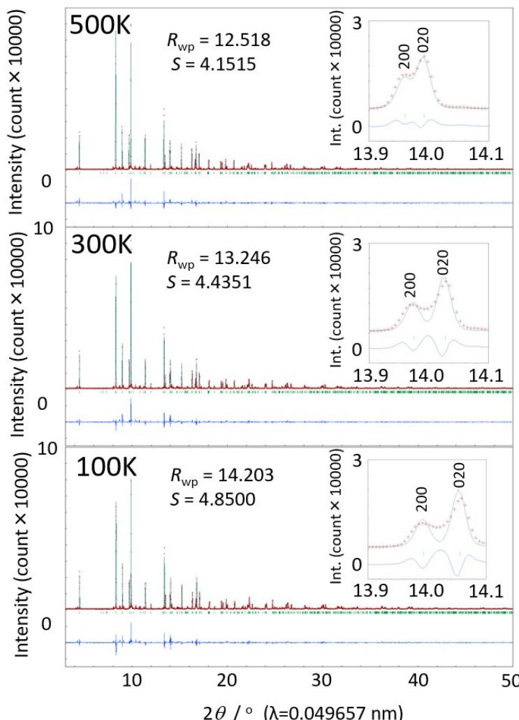
Figure S1 Rietveld refinement profile of LaOInS<sub>2</sub> at 100, 300 and 500 K.
