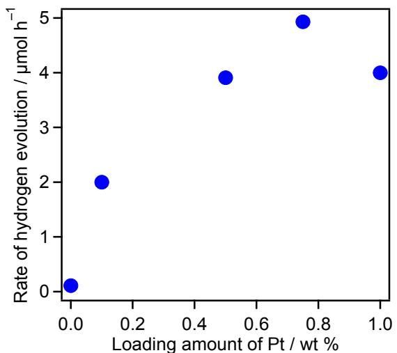
Figure S3 Dependence of photocatalytic H<sub>2</sub> evolution activity of Pt/LaOInS<sub>2</sub> on the loading amount of Pt under visible light ( $420 < \lambda < 800$  nm). Reaction conditions: catalyst, 50 mg; aqueous methanol solution (10 vol%, 140 mL); light source, xenon lamp (300 W) with cutoff filter; reaction vessel, Pyrex top-irradiation type.
