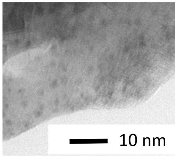
Fig S4 TEM image of 0.75 wt % Pt-loaded LaOInS<sub>2</sub>.
