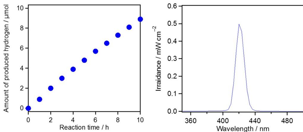
Figure S5 Time course of H<sub>2</sub> evolution on 0.75 wt% Pt/LaOInS<sub>2</sub> under visible light irradiation ( $\lambda = 420$  nm, 8.7 mW). Reaction conditions: catalyst, 50 mg; reactant solution, aqueous methanol solution, 140 mL (10 vol.%); light source, xenon lamp (300 W). (Right) Spectral irradiance from the light source.
