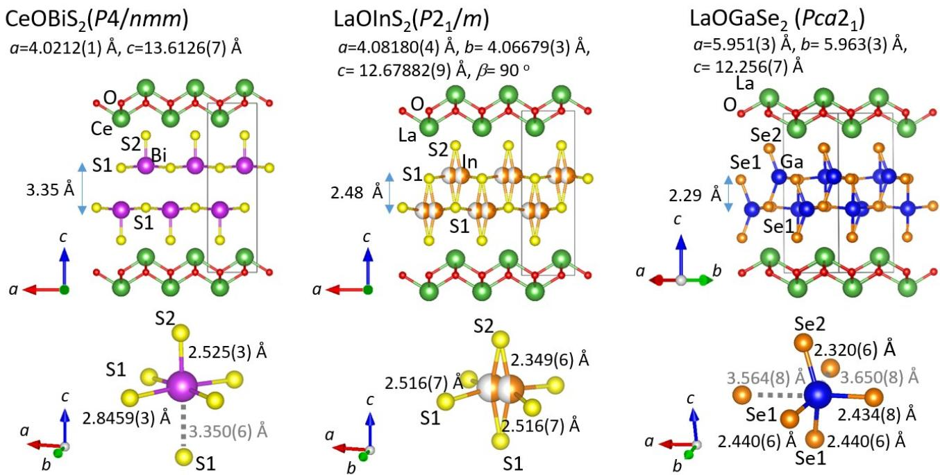
Figure S2 Crystal structure of structurally related layered oxychalcogenides: CeOBiS<sub>2</sub><sup>1</sup>, LaOInS<sub>2</sub>(this work) and LaOGaSe<sub>2</sub><sup>2</sup>. Grey lines indicate the unit cell.
