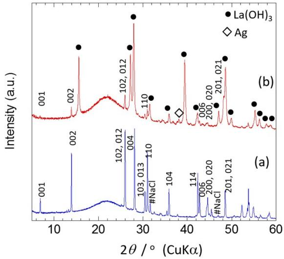
Figure S9 XRD diffraction patterns (a) before and (b) after photocatalytic O<sub>2</sub> evolution.
