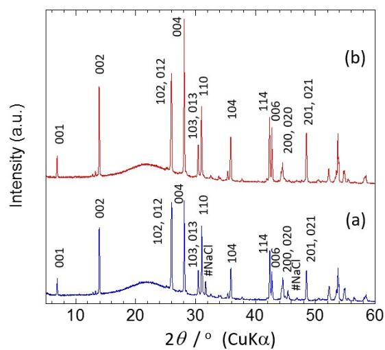
Figure S7 XRD diffraction patterns (a) before and (b) after photocatalytic H<sub>2</sub> evolution.
