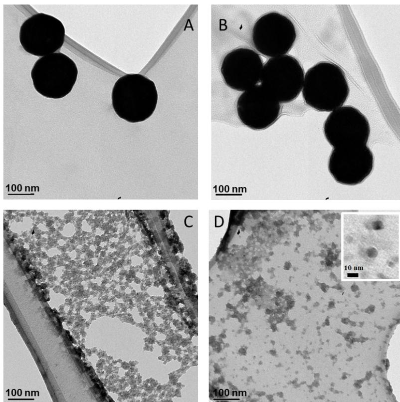
Figure S1. TEM images of the SiO<sub>2</sub>/Au NS (A & B) and CB NP (C & D) nanoparticles.
