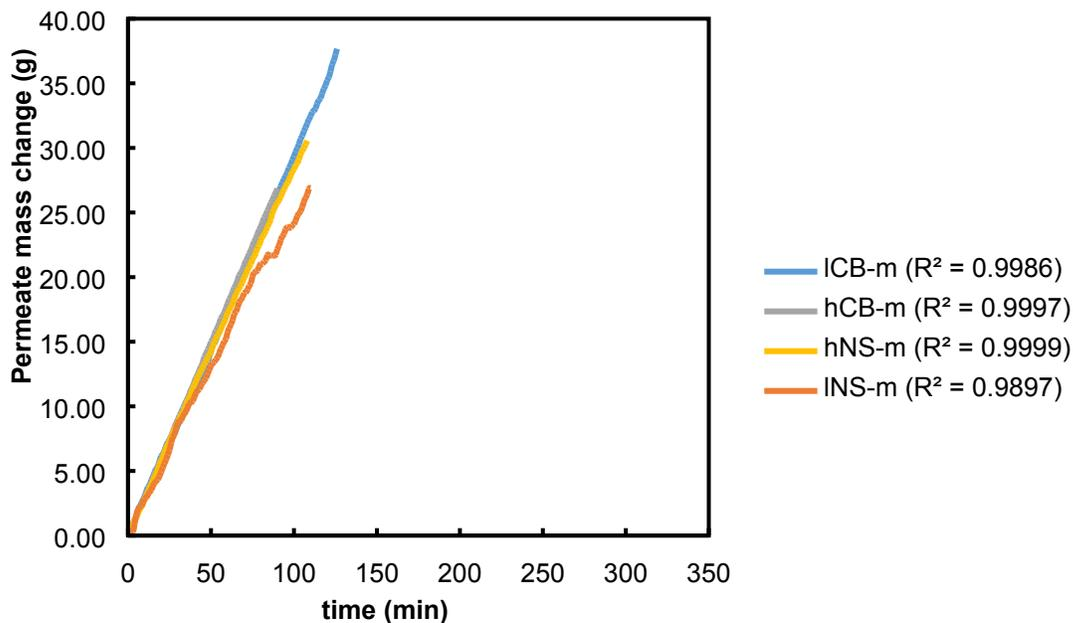
Figure S2. Representative curves of the permeate mass change over time of the modified membranes.
