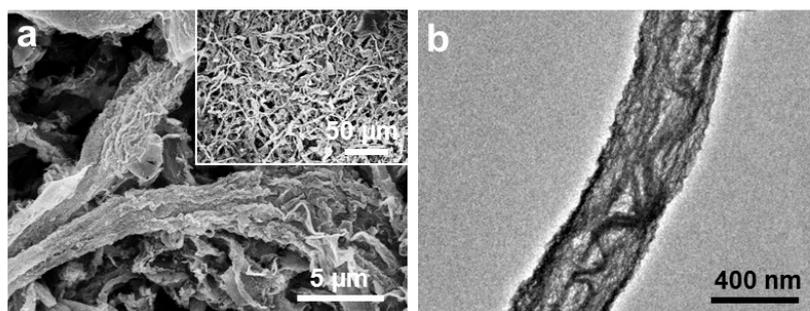
**Fig. S5** Electron microscope images of the  $(\text{ITO})_{10}\text{-NTs}$  film pasted on the Au photoanode. (a) Overview FE-SEM image; inset of (a) shows a hierarchical irregular porous nanotube networks of the  $(\text{ITO})_{10}\text{-NTs}$  film, and (b) overview TEM image of an individual ITO nanotube.
