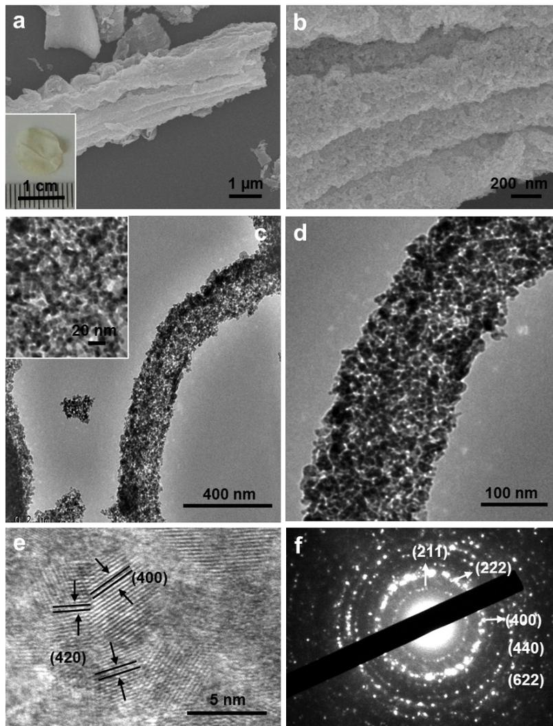
**Fig. S7** Electron microscope images of the sample  $(\text{ITO})_{15}\text{-NTs}$ . (a) Overview and (b) enlarged FE-SEM images of the sample  $(\text{ITO})_{15}\text{-NTs}$ ; inset of (a) shows the photograph of the  $(\text{ITO})_{15}\text{-NTs}$  film. (c) Overview and (d) enlarged TEM images of an individual ITO nanotube; inset of (c) shows the average size of ITO nanoparticle is about 6 nm. (e) HR-TEM micrograph and (f) SAED pattern of the sample  $(\text{ITO})_{15}\text{-NTs}$ .
