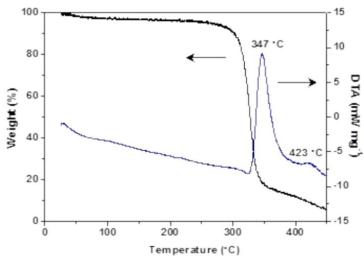
**Fig. S1** DTA/TG curves of the as-deposited ITO gel layer/filter paper composite sheet. The composite sheet was calcined at a heating rate of  $10\text{ }^{\circ}\text{C min}^{-1}$  from  $25\text{ }^{\circ}\text{C}$  to  $450\text{ }^{\circ}\text{C}$  in air.
