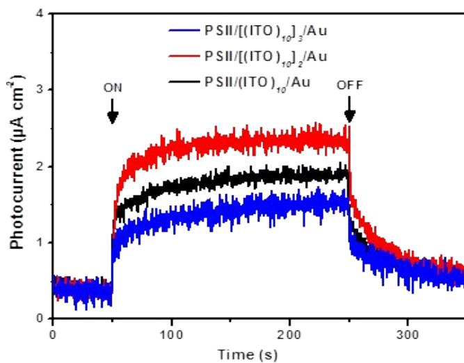
**Fig. S9** DET photocurrent responses of the PSII/ $(\text{ITO})_{10}/\text{Au}$ , PSII/ $[(\text{ITO})_{10}]_2/\text{Au}$  and PSII/ $[(\text{ITO})_{10}]_3/\text{Au}$  photoanodes. A bias potential of +0.25 V vs. SCE was applied at 25 °C.
