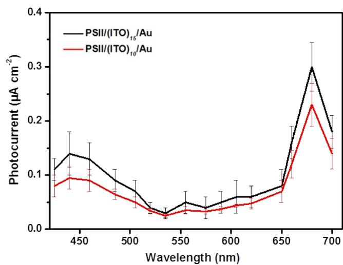
**Fig. S10** Photocurrent action spectra of the PSII/ITO/Au photoanodes.
