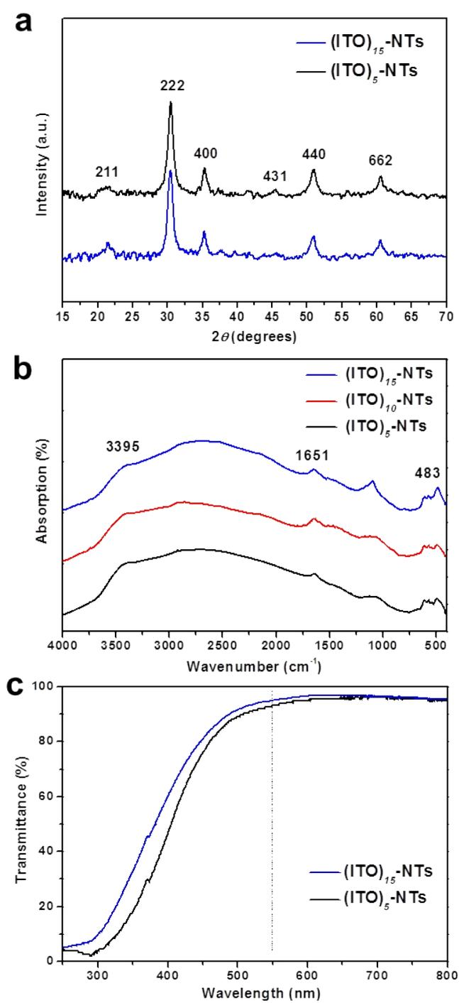
**Fig. S2** Spectral characterizations of the samples (ITO)<sub>n</sub>-NTs. (a) XRD patterns ( $n = 5, 15$ ), (b) FTIR spectra ( $n = 5, 10, 15$ ), (c) UV-vis spectra ( $n = 5, 15$ ).
