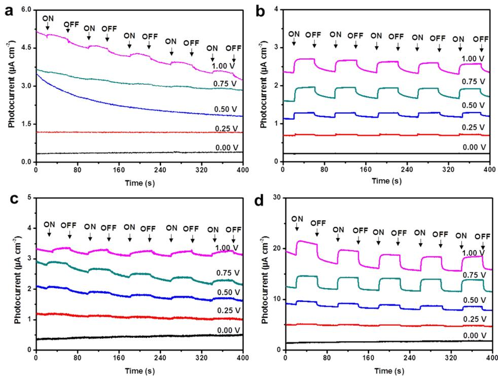
**Fig. S8** DET photocurrent responses of the fabricated photoanodes at varied bias potentials. DET photocurrent responses of the (a) Au, (b) PSII, (c) PSII/Au and (d)  $(\text{ITO})_{10}/\text{Au}$  photoanodes to repetitive illumination of white light and darkness cycles. A series of bias potentials of 0.00, +0.25, +0.50, +0.75 and +1.00 V vs. SCE were applied at 25 °C.
