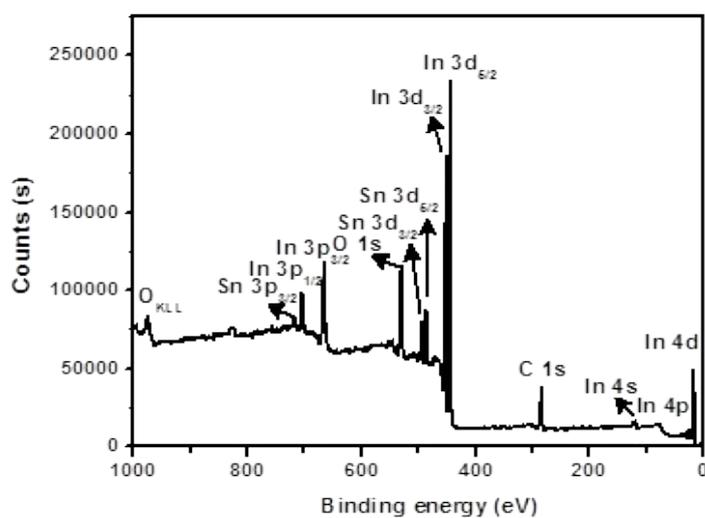
**Fig. S3** XPS wide scan spectrum of the sample (ITO)<sub>10</sub>-NTs.
