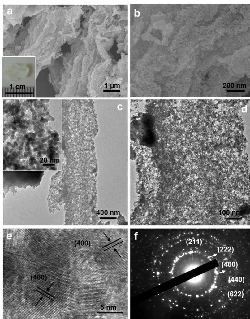
**Fig. S6** Electron microscope images of the sample  $(\text{ITO})_5\text{-NTs}$ . (a) Overview and (b) enlarged FE-SEM images of the sample  $(\text{ITO})_5\text{-NTs}$ ; inset of (a) shows the photograph of the  $(\text{ITO})_5\text{-NTs}$  film. (c) Overview and (d) enlarged TEM images of an individual ITO nanotube; inset of (c) shows the average size of ITO nanoparticle is about 6 nm. (e) HR-TEM micrograph and (f) SAED pattern of the sample  $(\text{ITO})_5\text{-NTs}$ .
