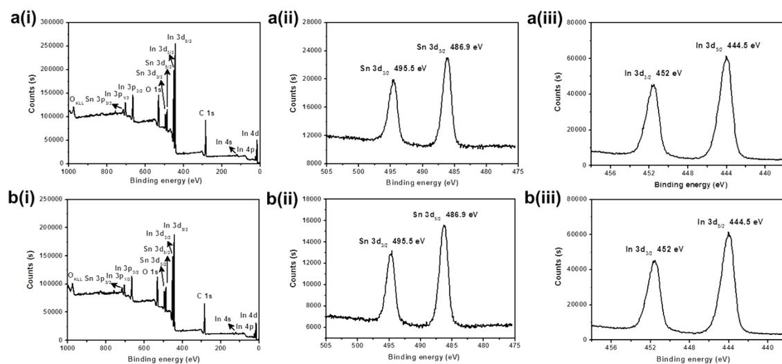
**Fig. S4** XPS spectra of the samples (ITO)<sub>n</sub>-NTs. XPS spectra of the samples (a) (ITO)<sub>5</sub>-NTs and (b) (ITO)<sub>15</sub>-NTs. (i) Wide scan spectra; (ii) Sn 3d spectra and (iii) In 3d spectra.
