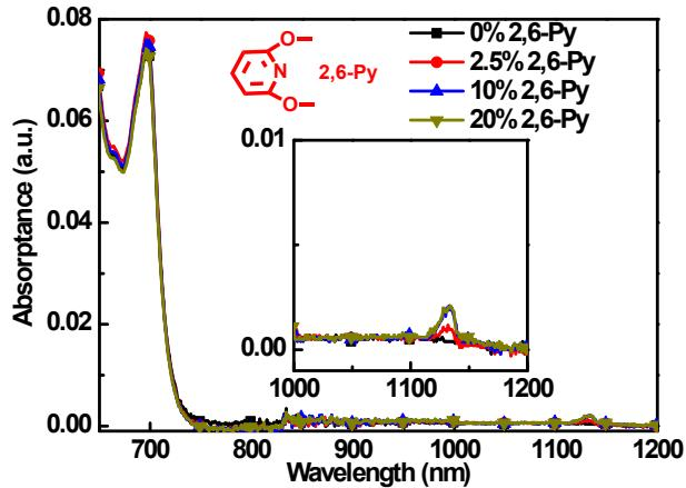
**Fig. S3.** The optical absorption of 2,6-Py doped PC<sub>61</sub>BM at varied dopant concentrations in CB solution.
