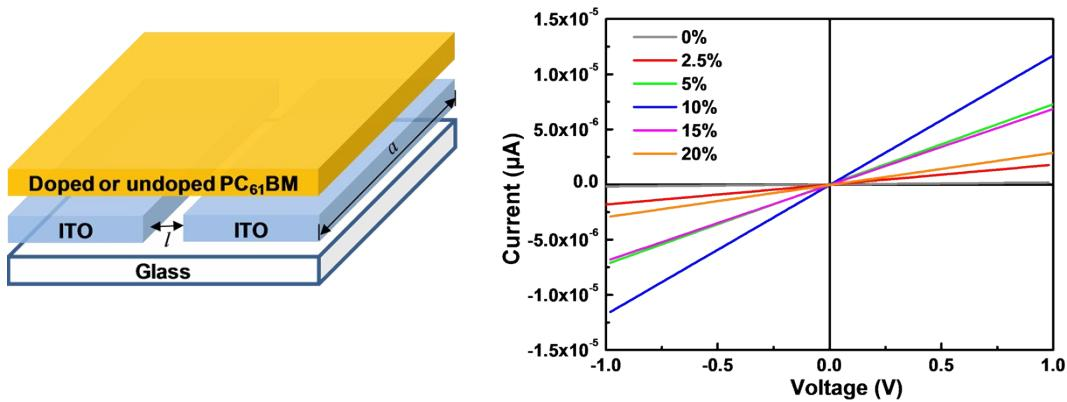
**Fig. S2.** (a) Structure of the device for conductivity measurements. (b) I-V characteristics of doped  $\text{PC}_{61}\text{BM}$  films at varied doping ratios, respectively.
