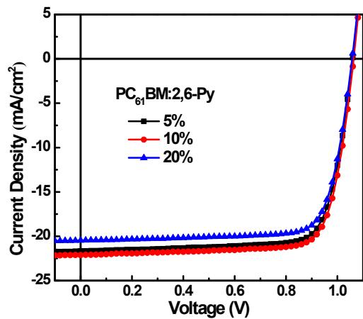
**Fig. S6.** The  $J$ - $V$  curves of perovskite solar cells with 2,6-Py doped  $\text{PC}_{61}\text{BM}$  at varied dopant concentrations.
