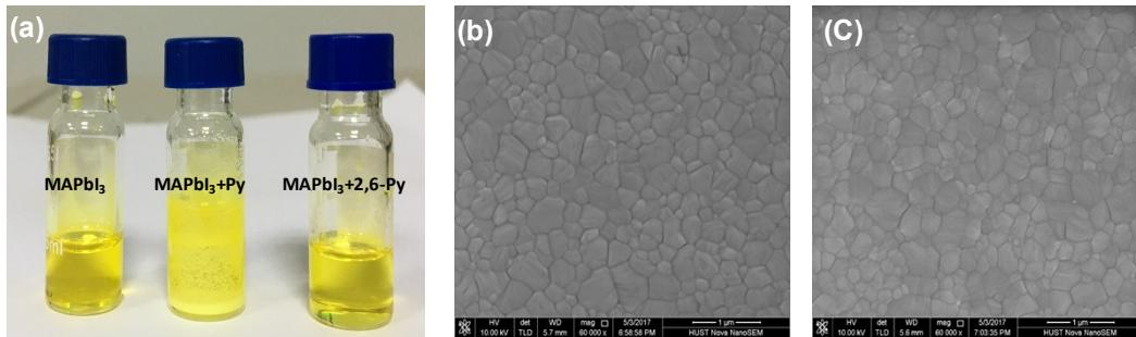
**Fig. S1.** (a) Photo images of DMF solutions with pristine  $\text{MAPbI}_3$ , mixture of  $\text{MAPbI}_3+\text{Py}$ , and  $\text{MAPbI}_3+2,6\text{-Py}$ ; Top-view SEM images of  $\text{MAPbI}_3$  films without (b) and (c) with 2,6-Py treatment.
