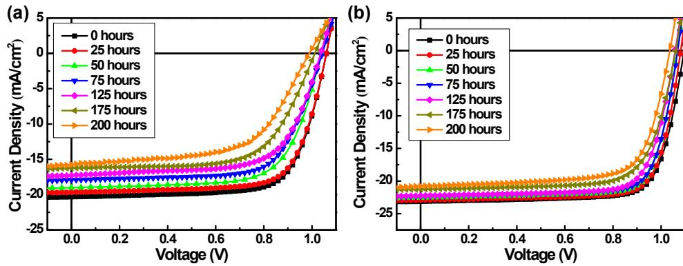
**Fig. S8.** *J-V* curves of the best MAPbI<sub>3</sub>-based devices with pristine PC<sub>61</sub>BM and (2,6-Py)/PC<sub>61</sub>BM:2,6-Py as a function of storage time under ambient conditions (25°C, 40% relative humidity).
