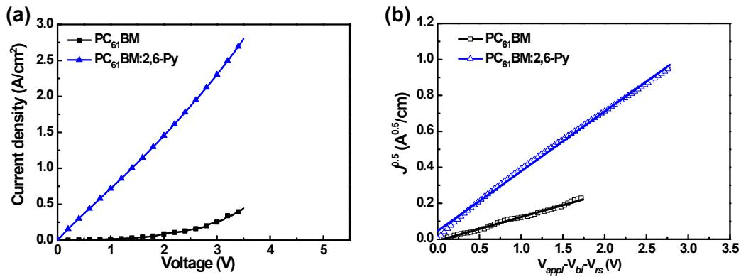
**Fig. S4.** (a)  $J$  vs  $V_{appl}$  and (b)  $J^{0.5}$  vs  $V_{appl}-V_{rs}-V_{bi}$  plots for electron only devices of ITO/ZnO (20 nm)/PCBM or doped PCBM/Ca (20 nm)/Al (80 nm).
