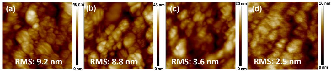
**Fig. S5.** AFM topographical height images of (a) pristine  $\text{MAPbI}_3$  film, (b) 2,6-Py treated  $\text{MAPbI}_3$  film, (c)  $\text{MAPbI}_3/\text{PC}_{61}\text{BM}$  film, and (d)  $\text{MAPbI}_3(2,6\text{-Py})/\text{PC}_{61}\text{BM}:2,6\text{-Py}$  film, respectively.
