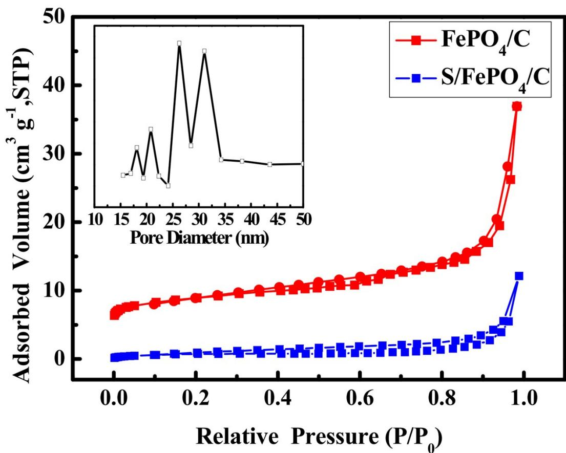
**Figure S1.** N<sub>2</sub> adsorption/desorption isotherms of FePO<sub>4</sub>/C nanocomposite (red) and S/FePO<sub>4</sub>/C nanocomposite (blue). The illustration is pore-size-distribution of FePO<sub>4</sub>/C nanocomposite.
