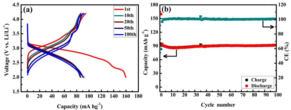
**Figure S12.** (a) Charge/discharge profiles of pure FePO<sub>4</sub> nanospheres cycled in DOL/DME /LTFSI/LiNO<sub>3</sub> electrolyte and (b) their corresponding cycling performance at 0.5 C.
