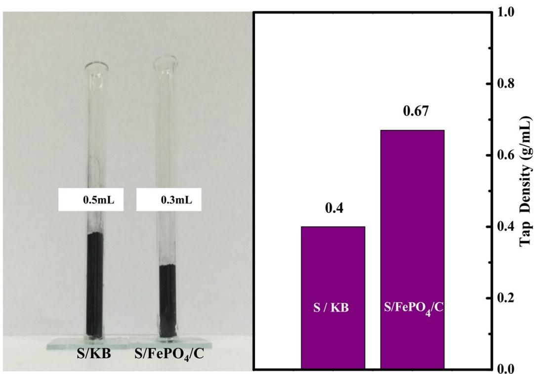
**Figure S9.** Comparison of tap densities of S/KB with 60 wt% S and S/FePO<sub>4</sub>/C with 64 wt% S for the same weight of 0.2 g, the tap densities is 0.4 and 0.67 g/mL respectively.
