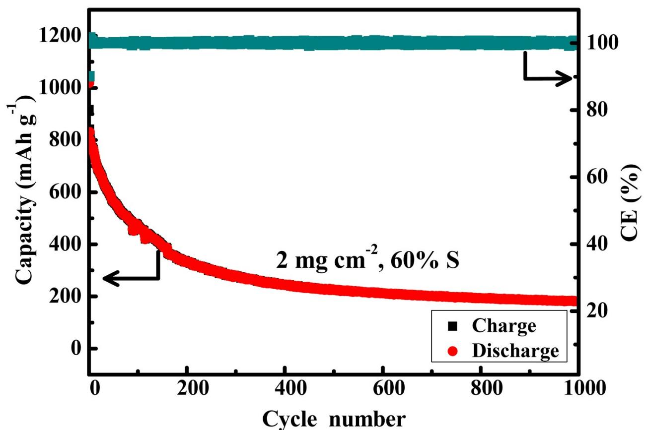
Figure S5. Cycling performance of S/KB composite with sulfur content of 60 wt% at 0.5 C.
