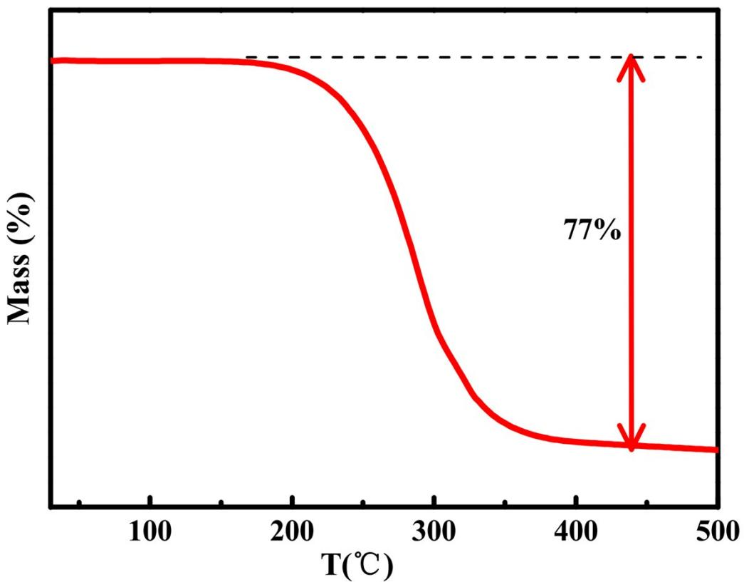
**Figure S10.** Thermo-gravimetric (TG) analysis of S/FePO<sub>4</sub>/C nanocomposite with sulfur contents of 77 wt%.
