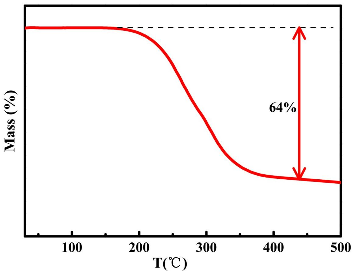
**Figure S2.** Thermo-gravimetric (TG) analysis of S/FePO<sub>4</sub>/C nanocomposite with sulfur content of 64 wt%.
