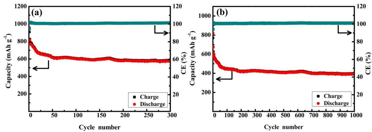
**Figure S11.** (a) Cycling performance of S/FePO<sub>4</sub>/C-77 wt% S at 0.2 C and (b) 0.5 C.
