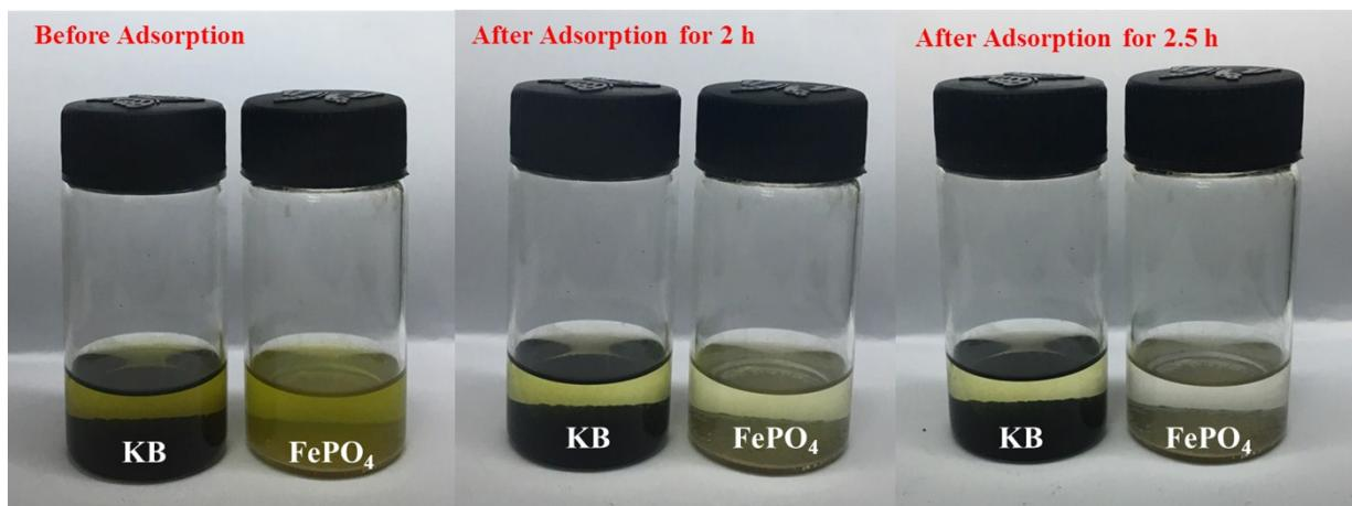
**Figure S6.** Photograph of sealed vials of a Li<sub>2</sub>S<sub>6</sub>/DME solution before and after soaking with FePO<sub>4</sub> or KB. The adsorption test was performed by adding 20 mg KB or FePO<sub>4</sub> to 0.002M Li<sub>2</sub>S<sub>6</sub> solution. Li<sub>2</sub>S<sub>6</sub> solution was prepared by adding Li<sub>2</sub>S and sulfur at a molar ratio of 1:5 in DME.
