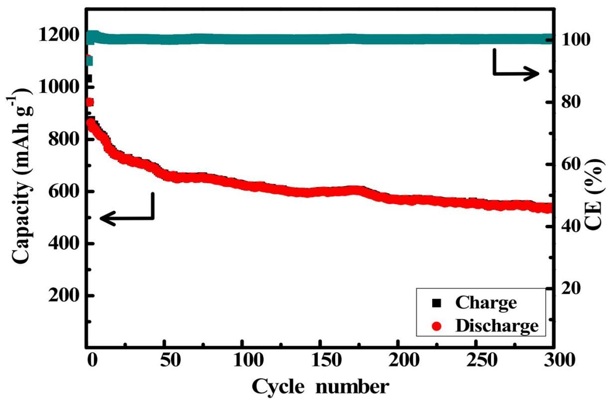
**Figure S7.** Cycling performance of S/FePO<sub>4</sub>/C-64 wt% at 0.2 C.
