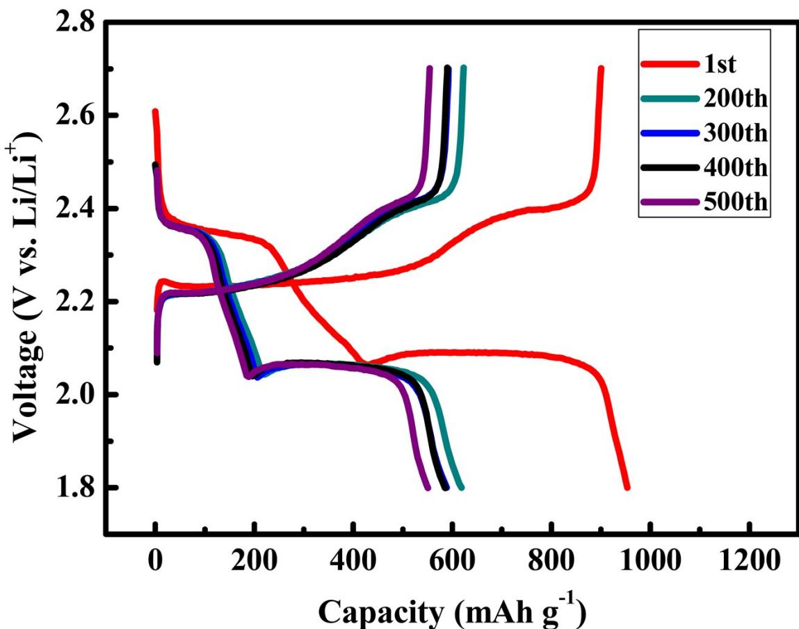
**Figure S4.** Charge-discharge profiles for selected cycles of S/FePO<sub>4</sub>/C-64 wt% at 0.5 C.
