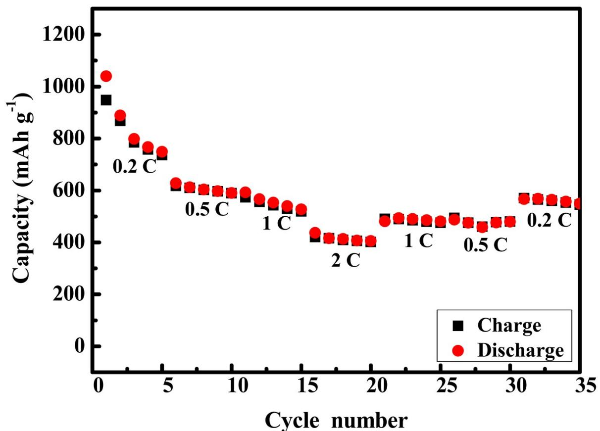
**Figure S3.** Rate performance of S/FePO<sub>4</sub>/C-64 wt% at various current densities from 0.1 C to 2 C.
