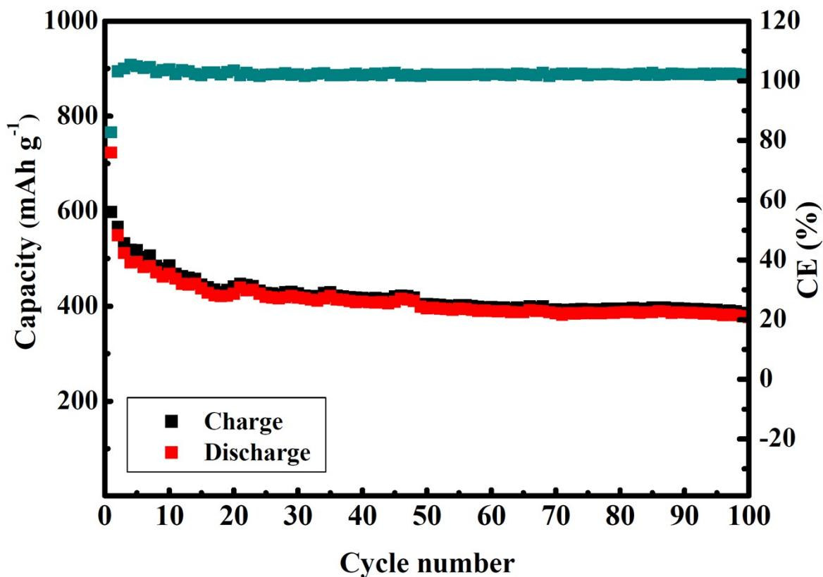
**Figure S8.** Electrochemical performance of S/FePO<sub>4</sub>/C-64 wt% with a total mass loading of 6 mg cm<sup>-2</sup> on the electrode at 0.5 C.
