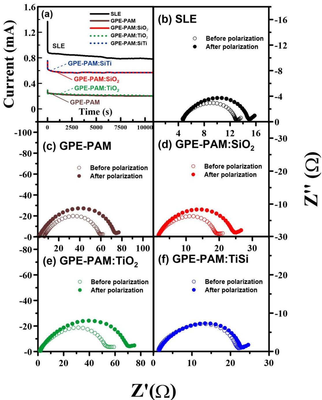
**Fig. S3.** (a) Current-time curves of Li|electrolyte|Li cells following application of DC voltage (5 mV) to the cell. (b–f) Corresponding Nyquist impedance plots of the cells, (b) SLE, (c) GPE-PAM, (d) GPE-PAM:SiO<sub>2</sub>, (e) GPE-PAM:TiO<sub>2</sub>, and (f) GPE-PAM:SiTi, which were used to determine the initial and final  $R_{\text{int}}$  values.
