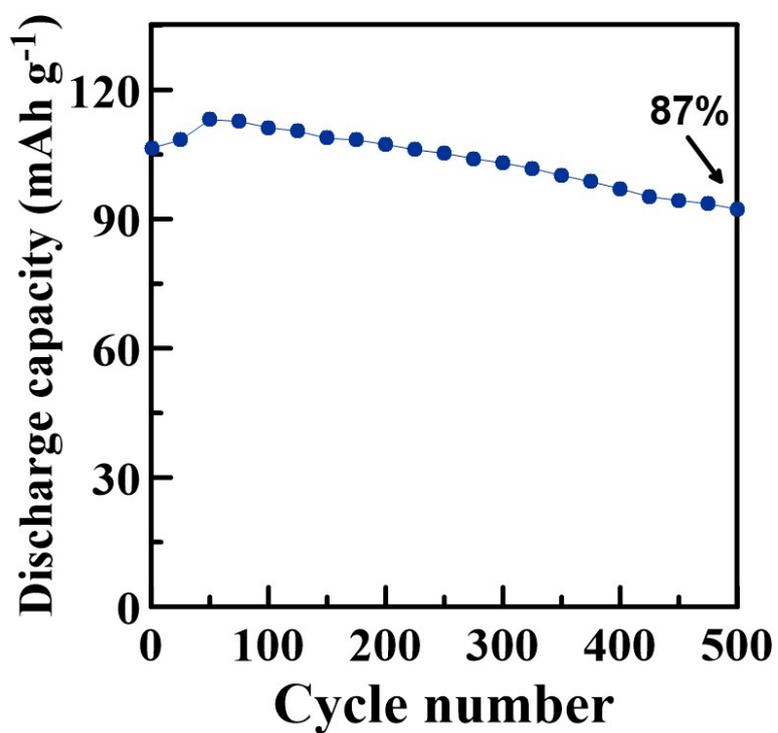
**Fig. S5.** Discharge capacities of the full-cell graphite|GPE-PAM-SiTi|LiFePO<sub>4</sub> battery following 500 cycles of charge–discharge at 5 C-rate over a voltage range of 2.0–3.8 V. The capacity retention at the 500<sup>th</sup> cycle was presented in the figure.
