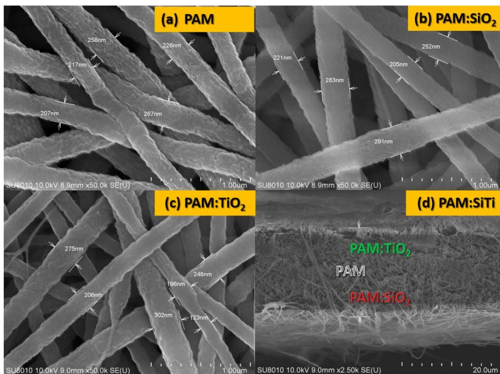
**Fig. S1.** SEM images of electrospun (a) PAM, (b) PAM:SiO<sub>2</sub>, and (c) PAM:TiO<sub>2</sub> membranes consisting of nanofibers and side-view image of the (d) PAM:SiTi membrane comprising PAM:SiO<sub>2</sub>, PAM, and PAM:TiO<sub>2</sub> layers connected in series.
