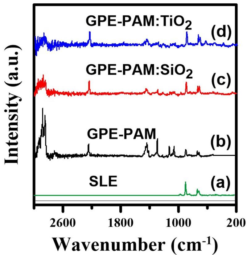
**Fig. S2.** The full-range Raman spectra of (a) SLE, (b) GPE-PAM, (c) GPE-PAM:SiO<sub>2</sub>, and (d) GPE-PAM:TiO<sub>2</sub>.
