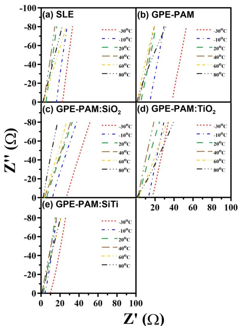
**Fig. S4.** Nyquist impedance spectra of electrolytes at various temperatures: (a) SLE; (b) GPE-PAM; (c) GPE-PAM:SiO<sub>2</sub>; (d) GPE-PAM:TiO<sub>2</sub>; (e) GPE-PAM:SiTi. The measurements were conducted by inserting the electrolytes between two stainless-steel electrodes and applying an AC potential amplitude of 5 mV over a frequency range of 0.1 Hz to 100k Hz at temperatures of -30 to 80 °C. The thicknesses of the GPEs and SLE were 50 and 12 μm, respectively.
