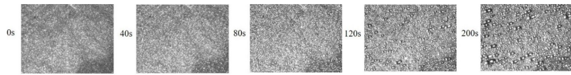
Fig. S4 Microscopic photographs of the droplets condensed on the nanostructured surface at temperatures of about 2°C.
