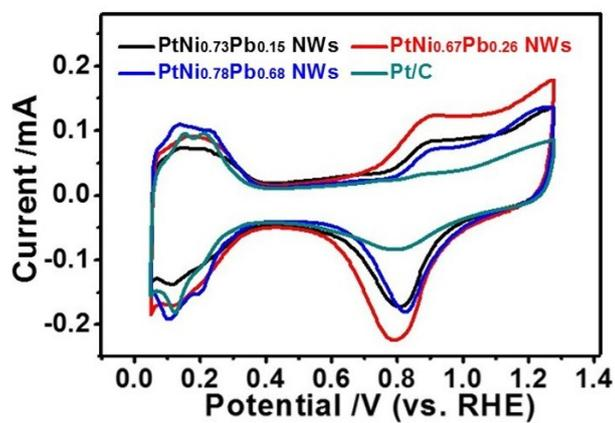
**Fig. S7** CVs of the PtNi<sub>0.73</sub>Pb<sub>0.15</sub> NWs, PtNi<sub>0.67</sub>Pb<sub>0.26</sub> NWs, PtNi<sub>0.78</sub>Pb<sub>0.68</sub> NWs and the commercial Pt/C in 0.1 M HClO<sub>4</sub> aqueous solution at scan rate of 50 mV/s.
