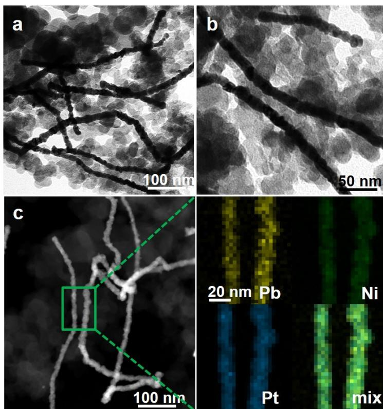
**Fig. S12** (a, b) TEM images, (c) HAADF-STEM image and EDS mapping images of PtNi<sub>0.67</sub>Pb<sub>0.26</sub> NWs/C after electrochemical durability test.
