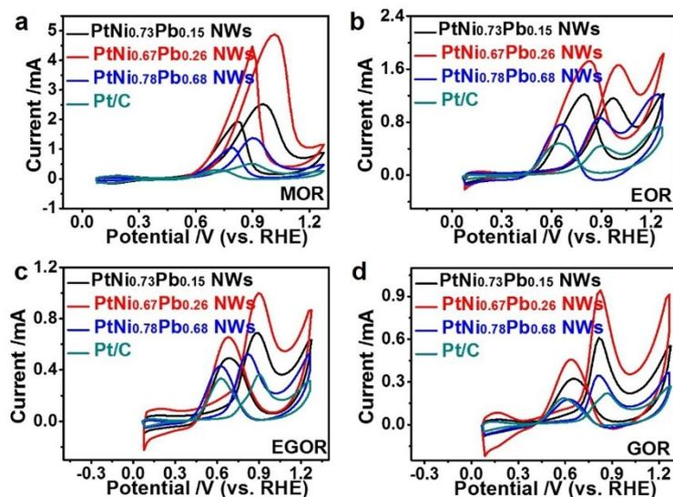
**Fig. S8** CVs of the PtNi<sub>0.73</sub>Pb<sub>0.15</sub> NWs, PtNi<sub>0.67</sub>Pb<sub>0.26</sub> NWs, PtNi<sub>0.78</sub>Pb<sub>0.68</sub> NWs and the commercial Pt/C for (a) MOR, (b) EOR, (c) EGOR and (d) GOR, respectively. The potential was scanned in 0.1 M HClO<sub>4</sub> aqueous solution containing 0.2 M methanol, 0.2 M ethanol, 0.2 M ethylene glycol or 0.2 M glycerol at scan rate of 50 mV/s.
