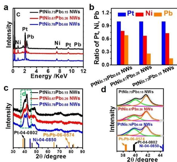
**Fig. S1** (a) SEM-EDS spectra, (b) the changes of the ratios of Pt, Ni and Pb. (c) PXRD patterns of different NWs and (d) the fitted peak curves form the marked region in (c).
