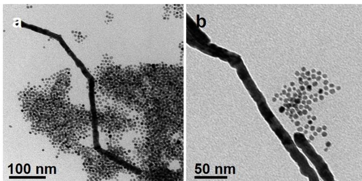
**Fig. S3** TEM images of the products obtained if the reaction temperature was not cooled to 80 °C.
