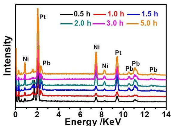
**Fig. S2** SEM-EDS spectra of the PtNi<sub>0.67</sub>Pb<sub>0.26</sub> NWs intermediates obtained after different reaction time.
