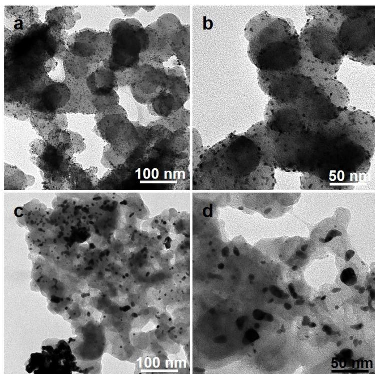
**Fig. S6** TEM images of the commercial Pt/C (a, b) before and (c, d) after the electrochemical durability test.
