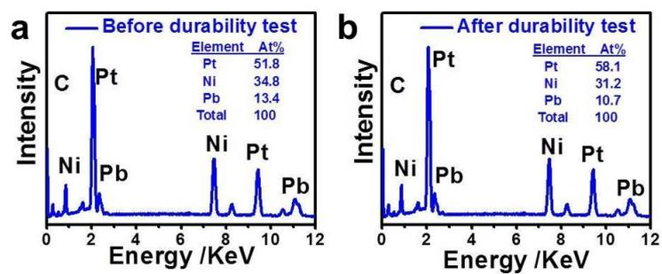
**Fig. S13** SEM-EDS spectra of PtNi<sub>0.67</sub>Pb<sub>0.26</sub> NWs/C (a) before and (b) after the electrochemical durability test.
