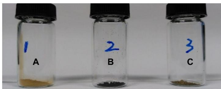
Fig. S2 Comparison of the optical images for the (a) pure FeOF, (b) PEDOT and (c) the coated FeOF powders.
