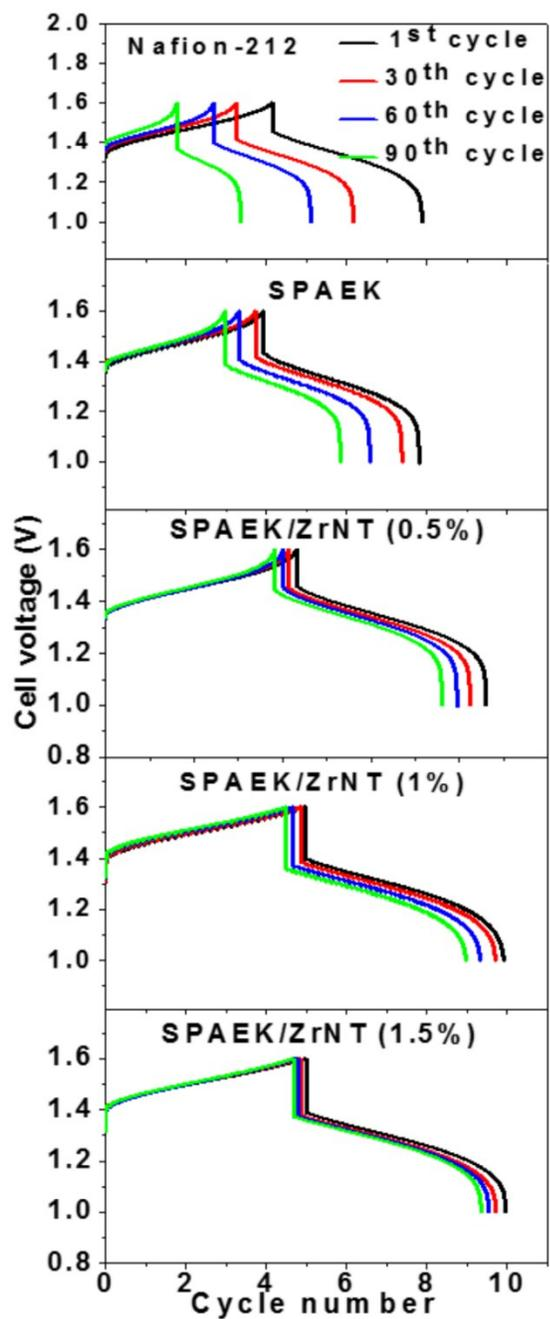
**Fig. S5** Charge-discharge curves of the VRB assembled with Nafion-212, SPAEK, SPAEK/ZrNT (0.5%), SPAEK/ZrNT (1%) and SPAEK/ZrNT (1.5%) membranes at 40 mA cm<sup>-2</sup> current density.
