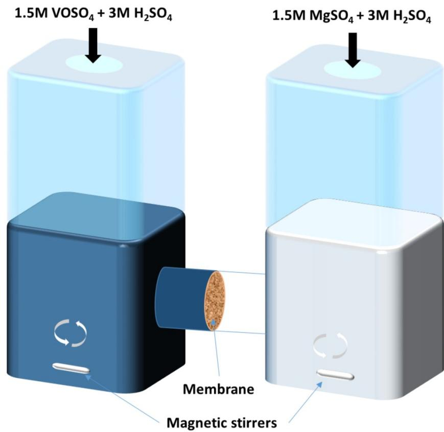
**Fig. S4** Schematic diagram of the cell used for the measurement of vanadium ion permeability of SPAEK/ZrNT composite membrane.
