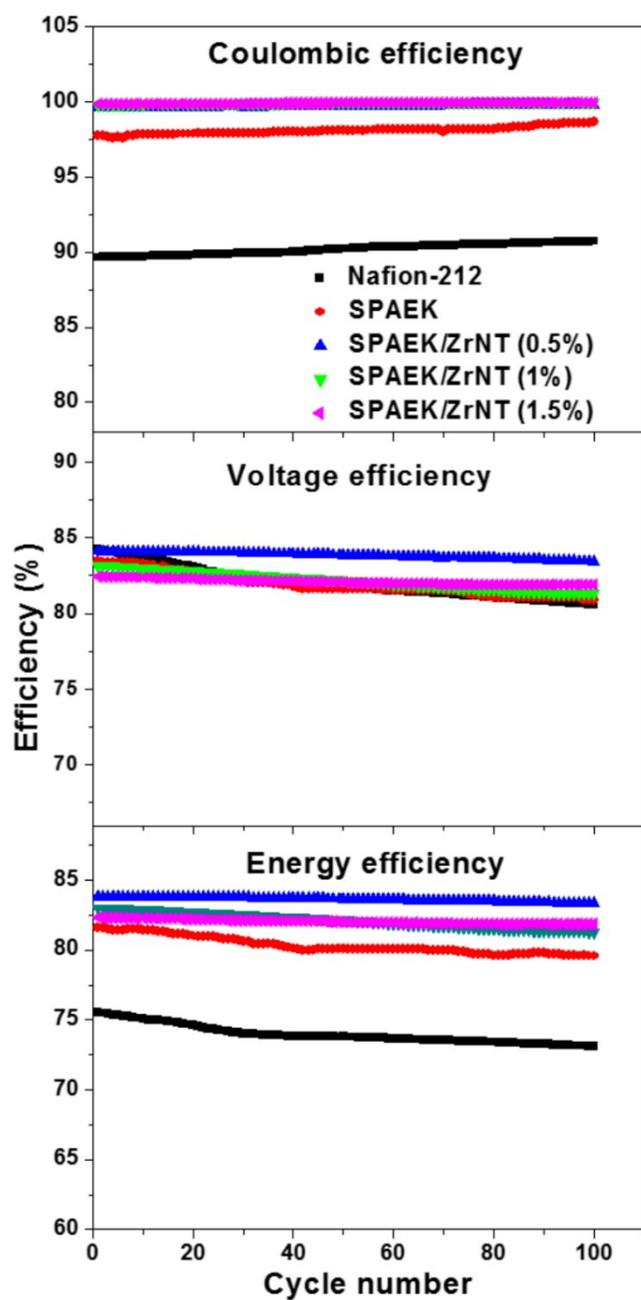
**Fig. S6** Cycle performance for the VRB assembled with Nafion-212, SPAEK, SPAEK/ZrNT (0.5%), SPAEK/ZrNT (1%) and SPAEK/ZrNT (1.5%) membranes as a function of cycling numbers at 40 mA cm<sup>-2</sup> current density.
