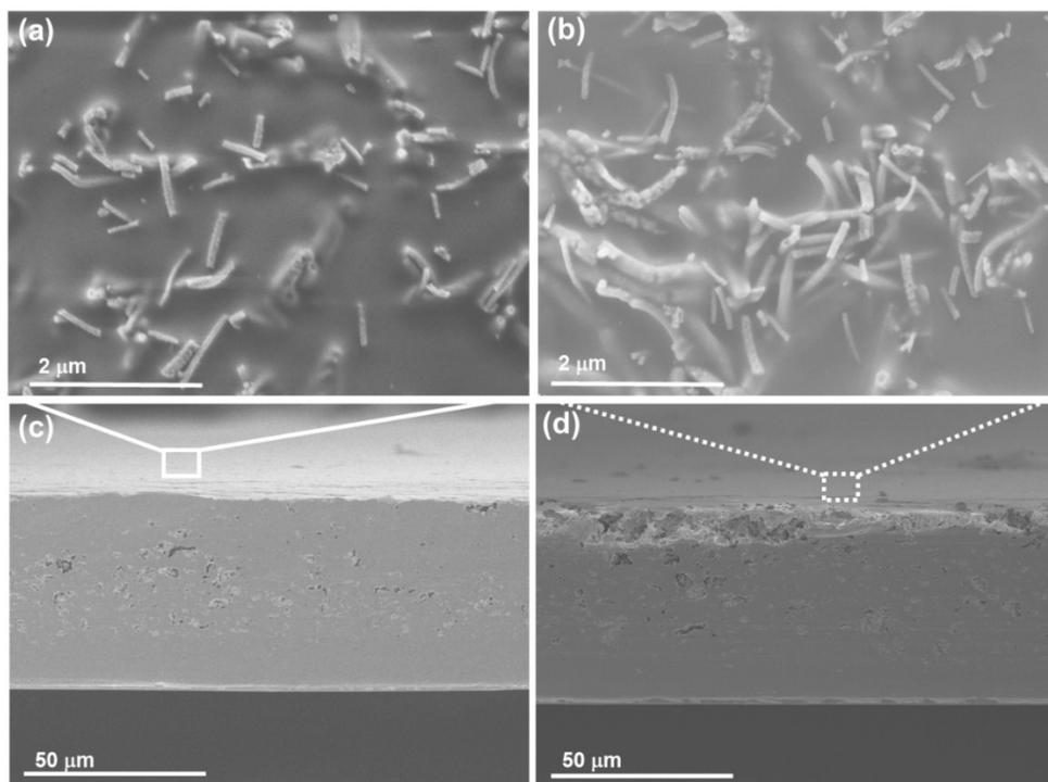
**Fig. S7** FE-SEM images of the surface and cross-section morphology of SPAEK/ZrNT (1%) composite membrane (a) and (c) initial. (b) and (d) after over 100 charge-discharge cycles in VRB.
