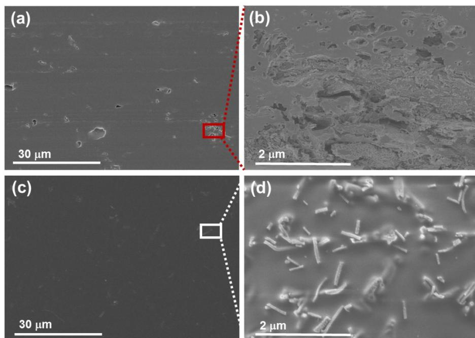
**Fig. S1** FE-SEM images of (a) and (b) SPAEK. (c) and (d) SPAEK/ZrNT (1%) membranes at different magnification.
