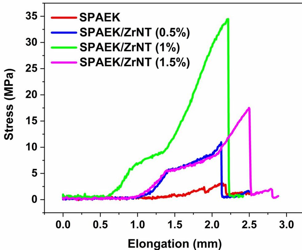
**Fig. S3** Tensile test of the dried SPAEK/ZrNT composite membranes in comparison with pristine SPAEK membrane under an ambient condition.
