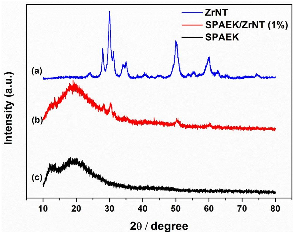
**Fig. S2** Powder X-ray diffraction pattern of samples (a) ZrNT. (b) SPAEK/ZrNT (1%) membrane. (c) SPAEK membrane.
