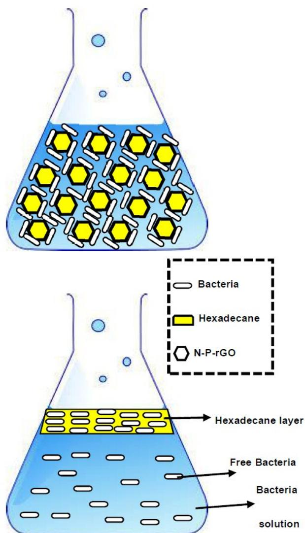
**Fig. S8.** Schematic illustration the effects of higher interfacial area and hydrophobic adsorption of hexadecane in the presence of N-P-rGO.
