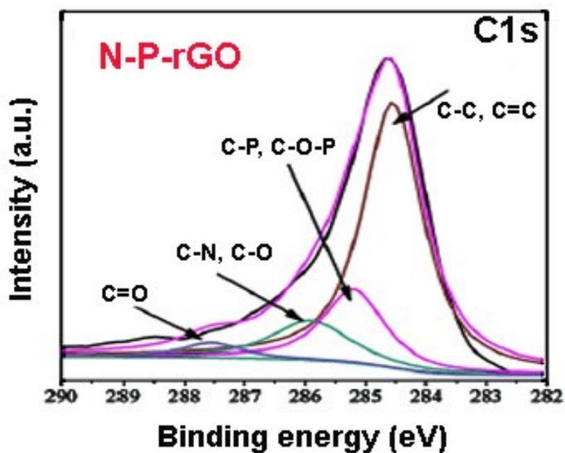
Fig. S2. High resolution spectrum of C 1s for N-P-rGO.
