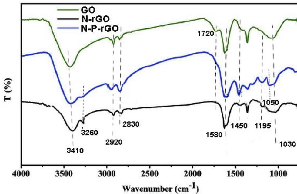
Fig. S4. IR spectra of GO, N-rGO, and N-P-rGO.
