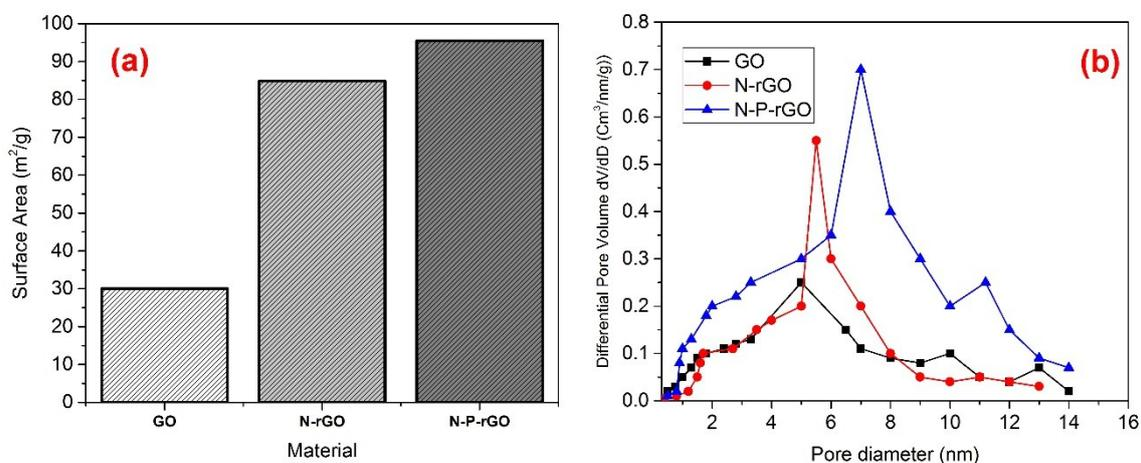
Fig. S1. (a) Specific surface areas of GO, N-rGO, and N-P-rGO; (b) Pore size distribution of GO, N-rGO, and N-P-rGO.
