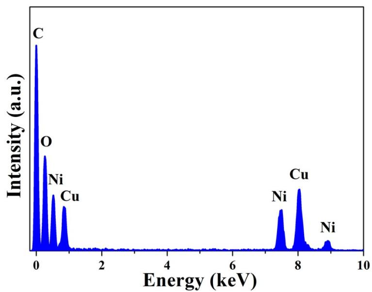
**Fig. S1** EDS spectrum of the as-prepared Ni-Tp sample.
