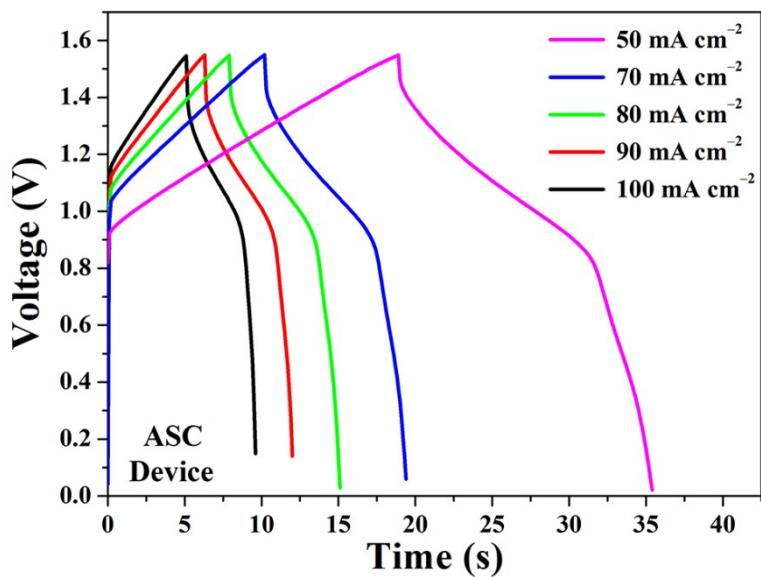
**Fig. S12** GCD curves of the assembled ASC device at the current densities of 50, 70, 80, 90, and  $100 \text{ mA cm}^{-2}$ .
