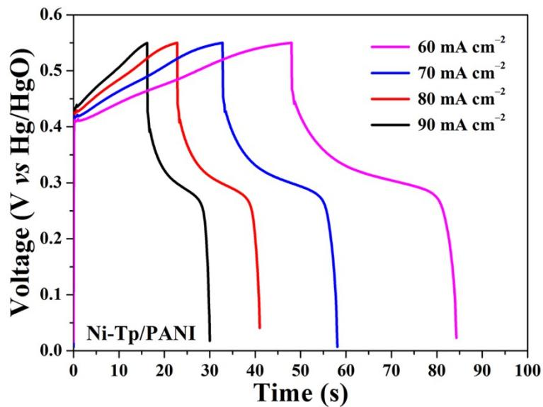
**Fig. S5** GCD curves of the prepared Ni-Tp/PANI electrode at the current densities of 60, 70, 80, and 90  $\text{mA cm}^{-2}$ .
