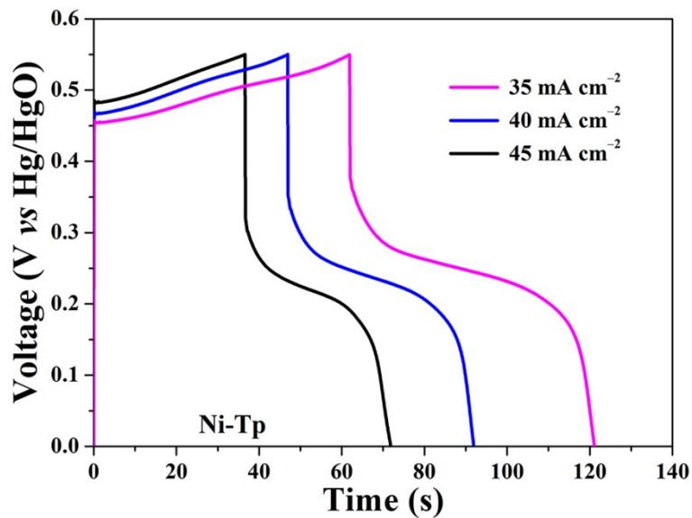
**Fig. S3** GCD curves of the prepared Ni-Tp electrode at the current densities of 35, 40, and 45 mA cm<sup>-2</sup>.
