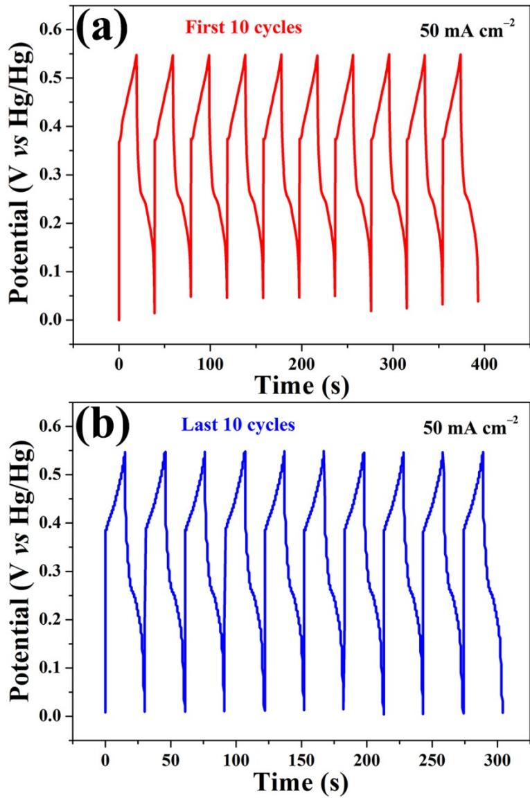
**Fig. S4** The (a) first and (b) last ten charge-discharge cycles of the as-synthesized Ni-Tp electrode at a current density of 50 mA cm<sup>-2</sup>.
