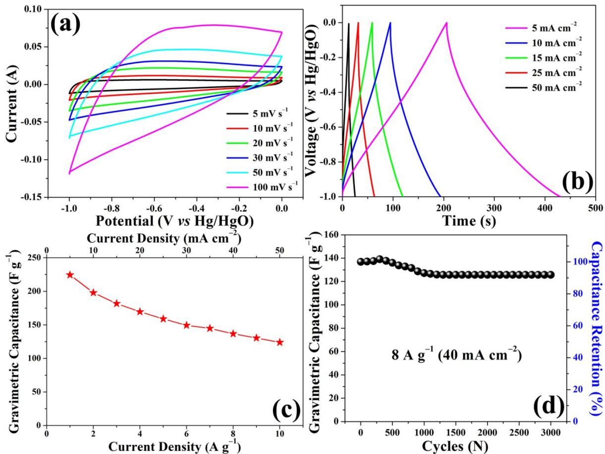
**Fig. S10** (a) CV curves of the activated carbon electrode at different scan rates in 3 M KOH aqueous solution. (b) GCD curves of the activated carbon electrode at different current densities. (c) The gravimetric capacitance of the activated carbon electrode as a function of current density. (d) Cycling performance of the activated carbon electrode at a current density of 8 A g<sup>-1</sup> (40 mA cm<sup>-2</sup>) in 3 M KOH aqueous solution.
