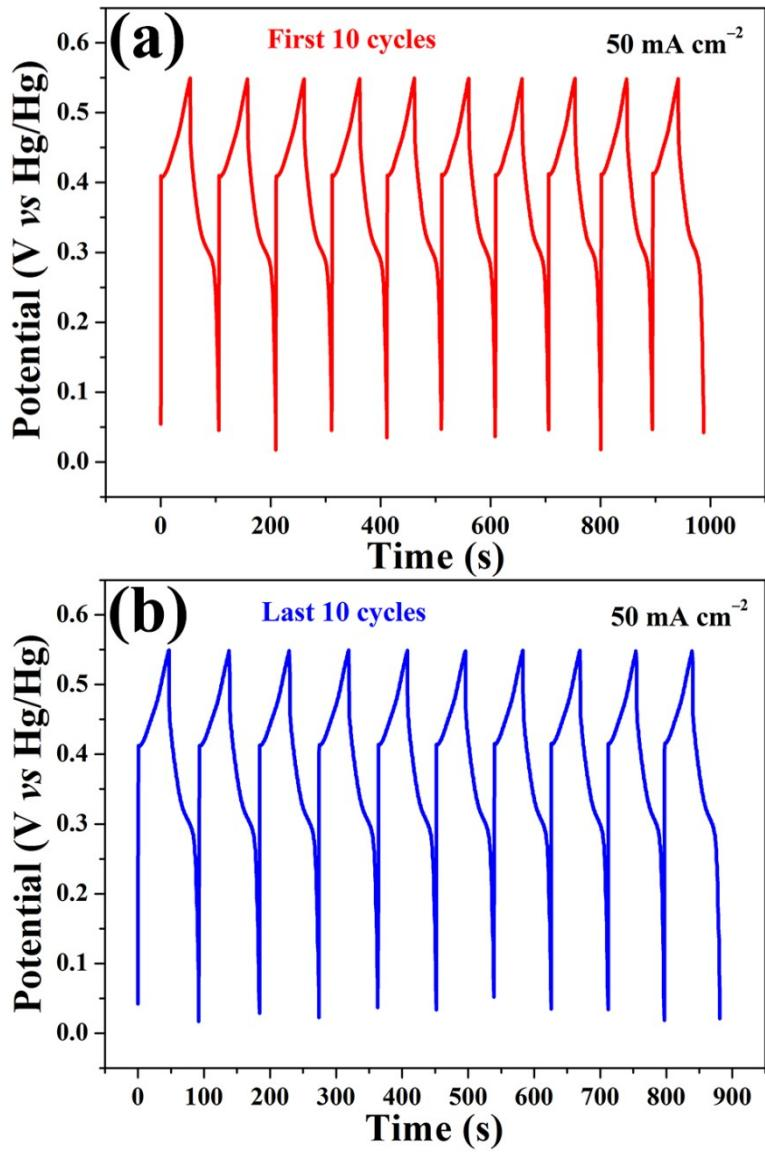
**Fig. S6** The (a) first and (b) last ten charge-discharge cycles of the as-synthesized Ni-Tp/PANI electrode at a current density of 50 mA cm<sup>-2</sup>.
