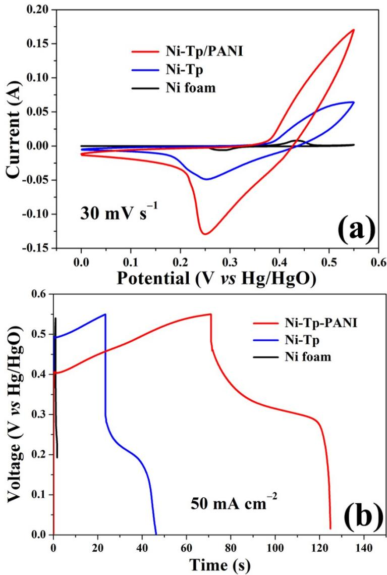
**Fig. S9** (a) Comparison of CV curves of the as-prepared Ni-Tp and Ni-Tp/PANI electrodes and the bare Ni foam at a scan rate of  $30 \text{ mV s}^{-1}$ . (b) Comparison of GCD curves of the as-prepared Ni-Tp and Ni-Tp/PANI electrodes and the bare Ni foam at a current density of  $50 \text{ mA cm}^{-2}$ .
