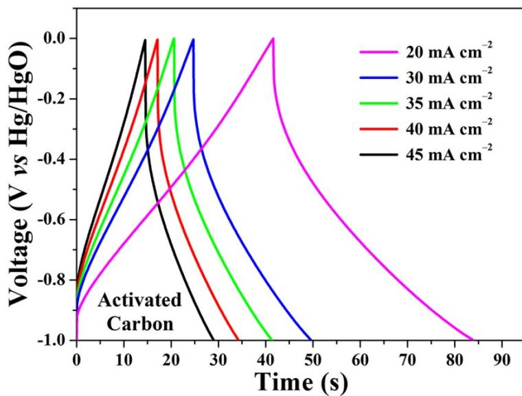
**Fig. S11** GCD curves of the prepared activated carbon electrode at the current densities of 20, 30, 35, 40, and 45 mA cm<sup>-2</sup>.
