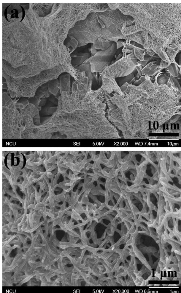
**Fig. S2** (a) The high-magnification SEM image of the PANI coated Ni-Tp and (b) the close-up SEM image of the deposited PANI.
