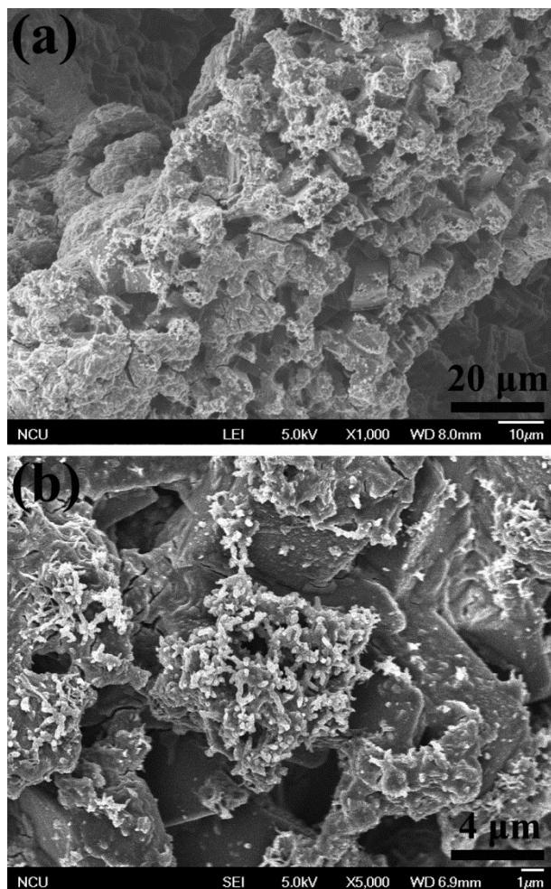
**Fig. S7** (a) The low-magnification and (b) high-magnification SEM images of the Ni-Tp/PANI electrode after cycling test.
