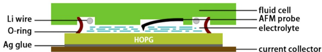
Fig. S1. The cross-sectional view of the liquid cell with electrochemical connections.
