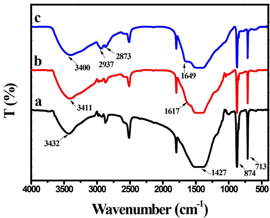
**Fig. S1.** FT-IR spectra of (a) CaCO<sub>3</sub>, (b) CaCO<sub>3</sub>@PDA and (c) CaCO<sub>3</sub>@PDA@PEI;
