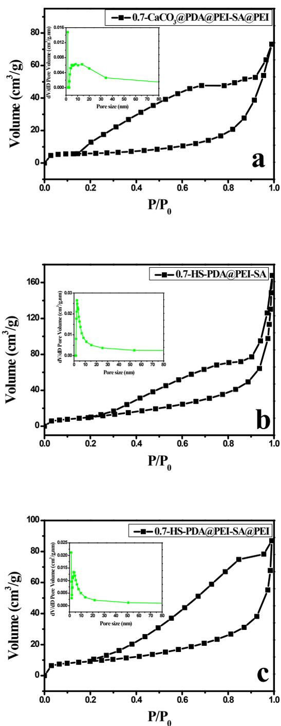
**Fig. S4.** Nitrogen adsorption–desorption isotherms and BJH pore size distribution curves of (a) 0.7-CaCO<sub>3</sub>@PDA@PEI-SA@PEI, (b) 0.7-HS-PDA@PEI-SA and (c) 0.7-HS-PDA@PEI-SA@PEI.
