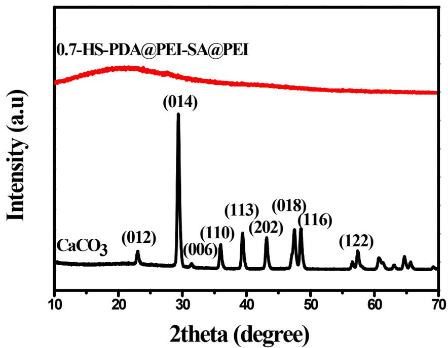
Fig. S3. XRD patterns of the  $\text{CaCO}_3$  and  $0.7\text{-HS-PDA@PEI-SA@PEI}$ .
