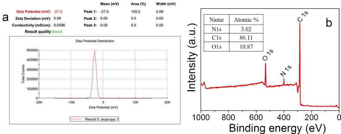
Figure S3. Zeta potential pattern of AMCRs (a), XPS survey spectrum of AMCRs (b).
