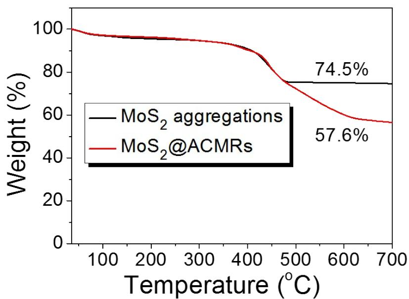
Figure S7. Thermogravimetric analysis of self-assembly MoS<sub>2</sub> and MoS<sub>2</sub>@AMCRs. Let the weight percentage of MoS<sub>2</sub> in the MoS<sub>2</sub>@AMCRs to be x. Assuming AMCRs are completely removed after combustion, one has  $0.745x = 0.576$ . Therefore  $x = 0.773$ .
