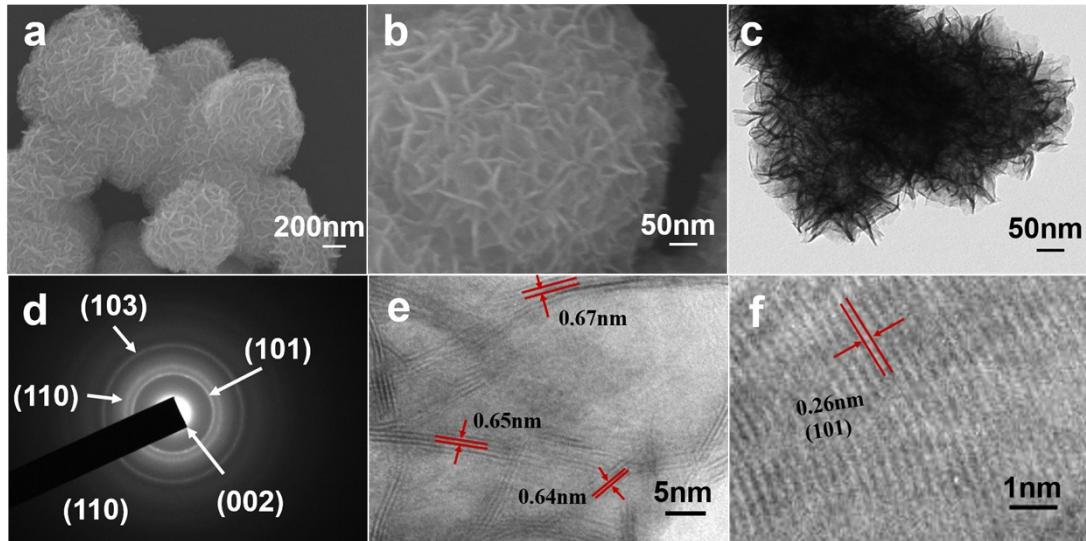
Figure S4. Electron microscopic characterization of  $\text{MoS}_2$  aggregations. SEM morphologys (a, b) in different magnifications, TEM image (c), SAED pattern (d), and HRTEM images (e, f).
