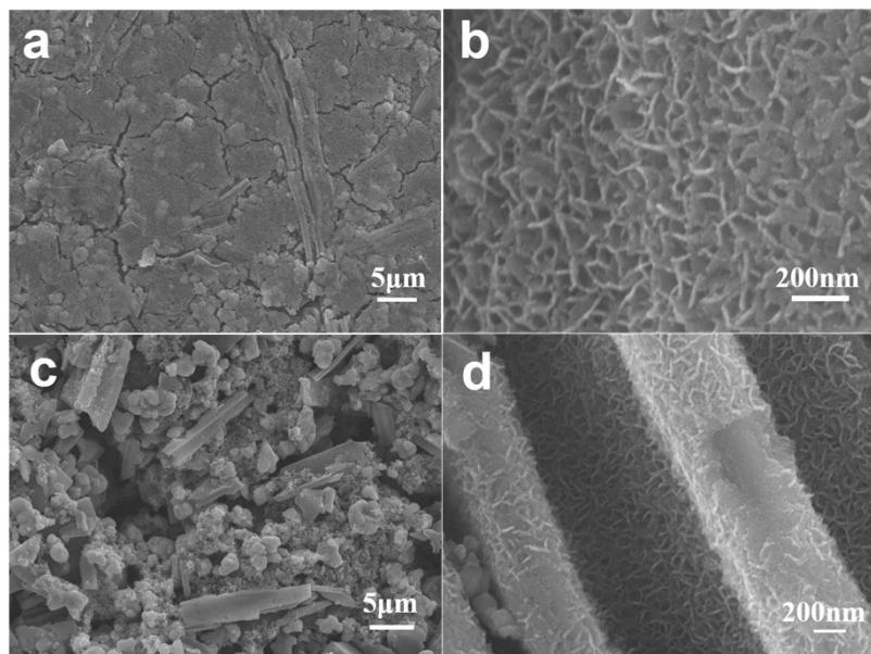
Figure S8. Postmortem morphologys of anodes after 10 charge-discharge cycles: CMC as the binder (a, b), and PVDF as the binder (c, d) in different magnifications.
