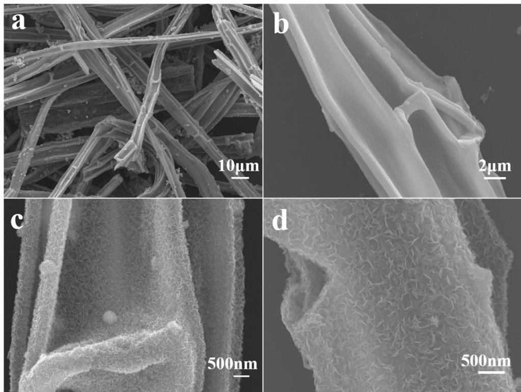
Figure S5. SEM images of  $\text{MoS}_2$ @AMCRs at different scales (a, b, c, d).
