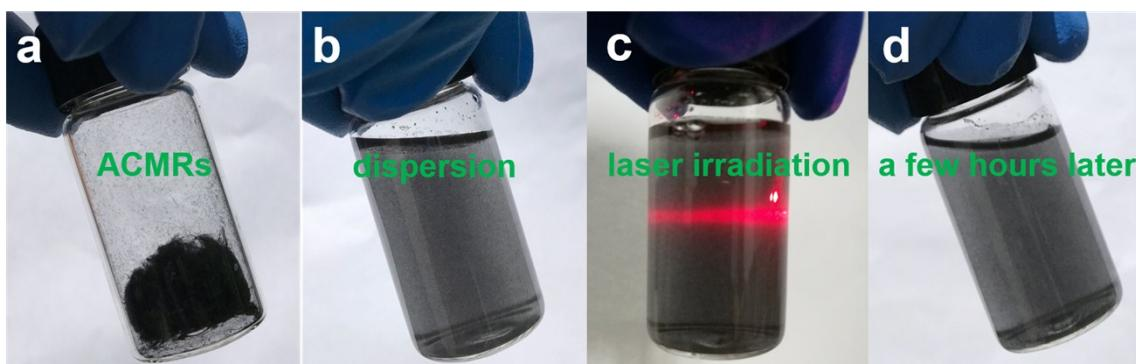
Figure S2. The excellent dispersion of AMCRs in distilled water. Moderate AMCRs in a vial (a), the AMCRs dispersing in equivalent amount of water relative with synthetic procedure (b), and Tyndall effect under laser irradiation (c), the dispersion retention of AMCRs in water after a few hours.
