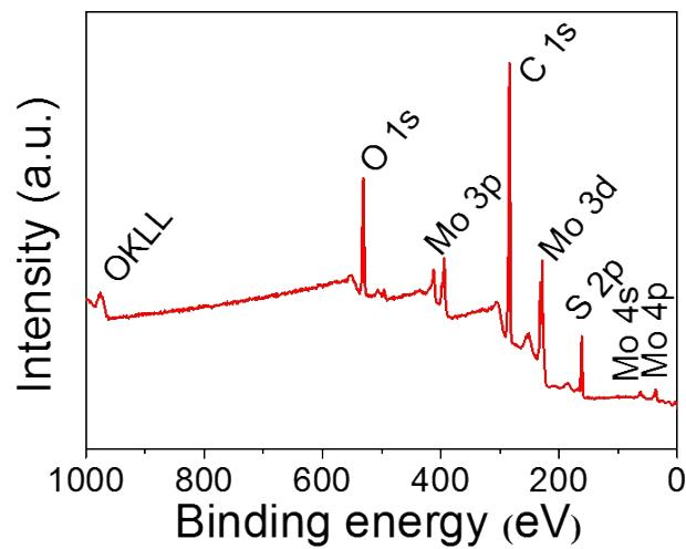
Figure S6. XPS survey spectrum of  $\text{MoS}_2$ @AMCRs composite.
