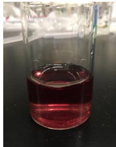
**Fig. S11** Digital photograph of PCN-222 upon exposure to basic solution (pH=11).
