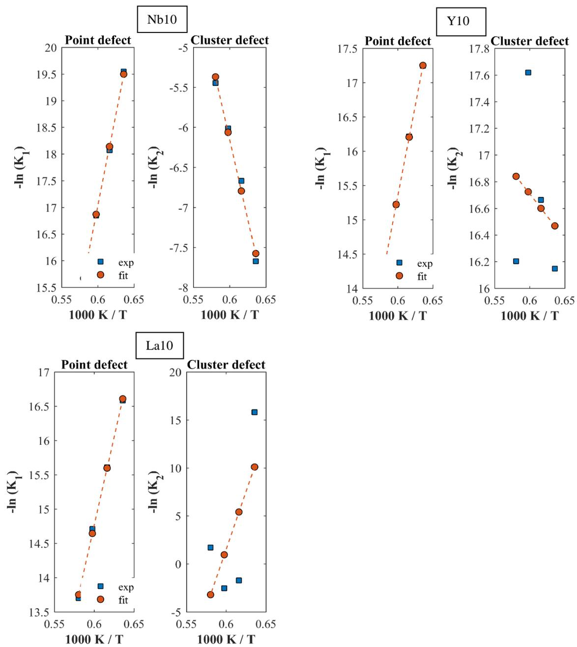
Fig. S5 Equilibrium constants  $K_1$  and  $K_2$ . The squares are isothermally derived values, the dots are based on a linear fit in the Van't Hoff plot.
