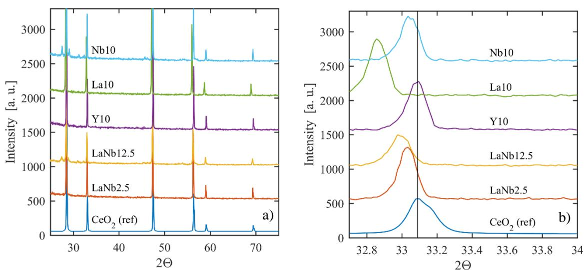
Fig. S1a) XRD patterns of LaNb2.5, LaNb12.5, Y10, La10 and Nb10 after TG analysis. A reference pattern of undoped ceria is included for comparison. b) Close up of peaks around 33.1°.
