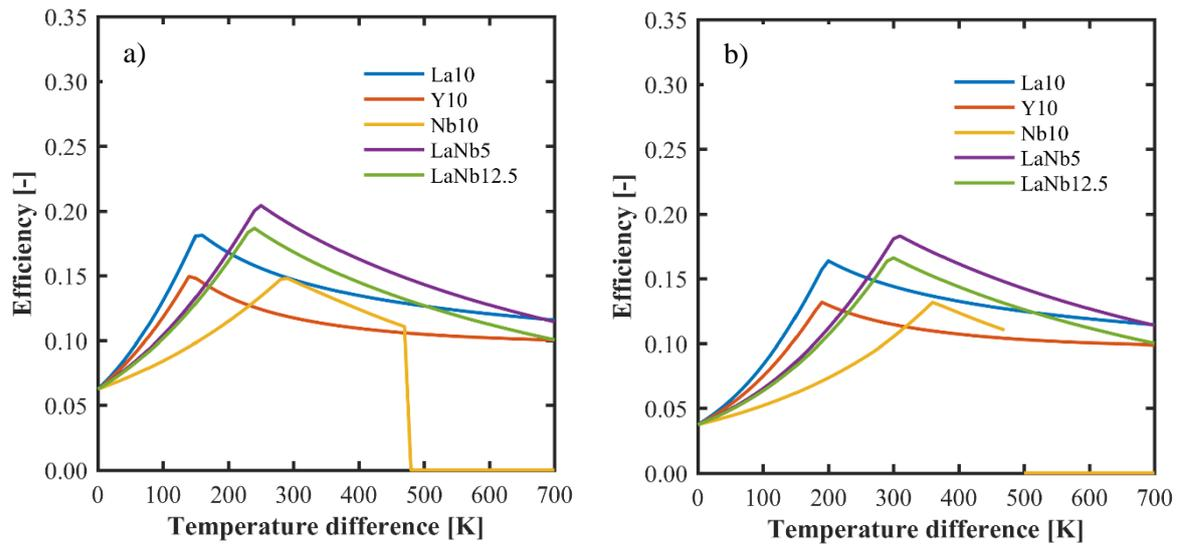
Fig. S6 Solar-to-fuel energy conversion efficiency as a function of the temperature swing between reduction and oxidation for the production of H<sub>2</sub> from H<sub>2</sub>O (a) and CO from CO<sub>2</sub> (b).
