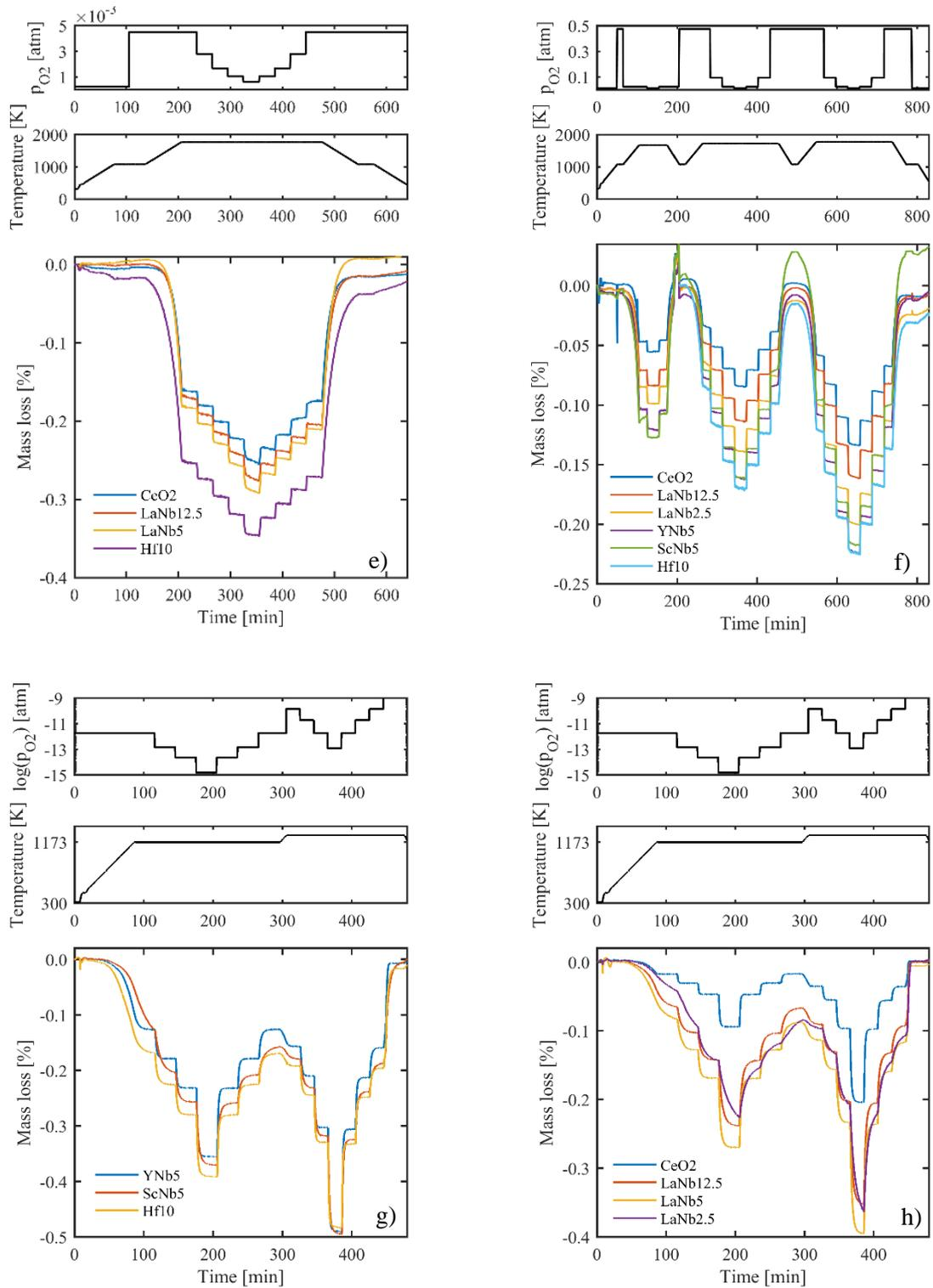
Fig. S3 TG experiments in the range (a) and (b) 1573 – 1673 K and  $2.5 \times 10^{-5}$  –  $4.8 \times 10^{-4}$  atm, (c) and (d) 1573 - 1773 K and  $2.5 \times 10^{-4}$  –  $4.8 \times 10^{-3}$  atm, (e) 1773 K and  $6.5 \times 10^{-4}$  –  $4.8 \times 10^{-3}$  atm, (f) 1673 – 1773 K and  $4.8 \times 10^{-3}$  –  $5.0 \times 10^{-1}$  atm (g) and (h) 1173 – 1273 K and  $1.6 \times 10^{-15}$  –  $1.4 \times 10^{-10}$  atm
