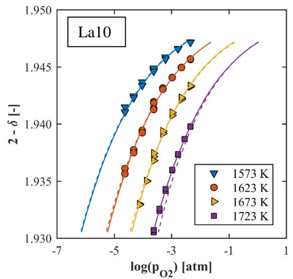
Fig. S4 Measured nonstoichiometries (symbols) of investigated materials. Solid lines show the predicted nonstoichiometry based on isothermally derived equilibrium constants; the dashed lines are based on the inversed temperature dependence of  $\ln(K1)$  and  $\ln(K2)$ .
