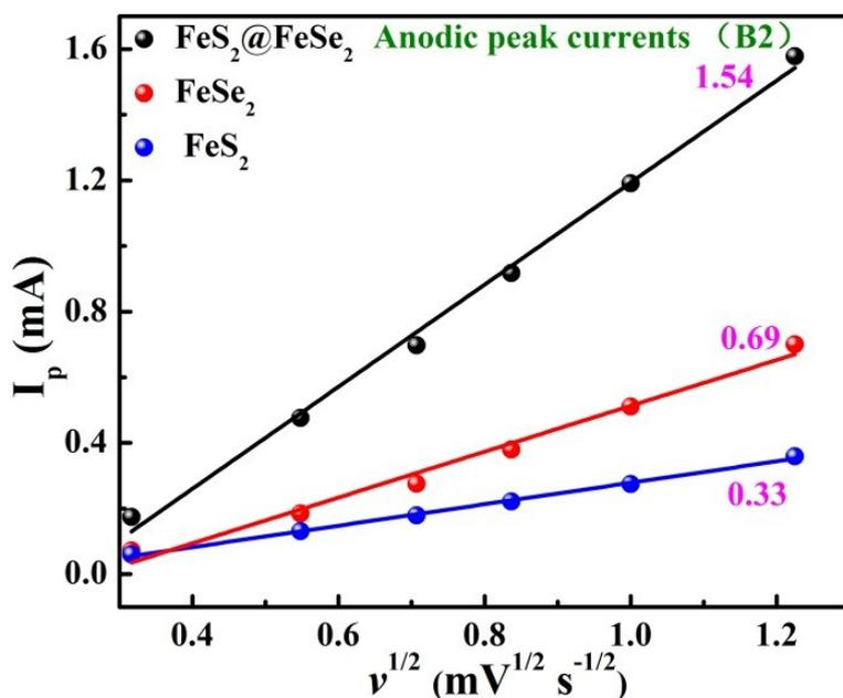
**Fig. S22.** Liner relationship between the peak current ( $I_p$ ) and square root of the scan rate ( $v^{1/2}$ ) of  $\text{FeS}_2@\text{FeSe}_2$ ,  $\text{FeSe}_2$  and  $\text{FeS}_2$ , respectively.
