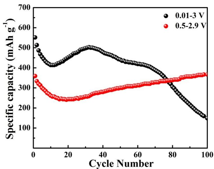
Fig. S8 The comparison of cycling performance for  $\text{FeS}_2@\text{FeSe}_2$  electrode at a voltage windows of 0.5-2.9 V and 0.01-3 V at  $1 \text{ A g}^{-1}$ .
