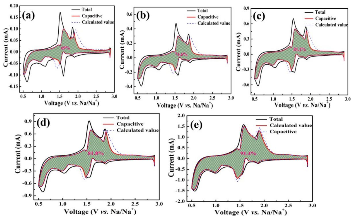
Fig. S20. Different CV curves of the FeS<sub>2</sub>@FeSe<sub>2</sub> electrode with the pseudocapacitive contribution to the total current shown by the shaded part. (a) 0.1 mV s<sup>-1</sup>, (b) 0.3 mV s<sup>-1</sup>, (c) 0.5 mV s<sup>-1</sup>, (d) 0.7 mV s<sup>-1</sup>, (e) 1.5 mV s<sup>-1</sup>.
