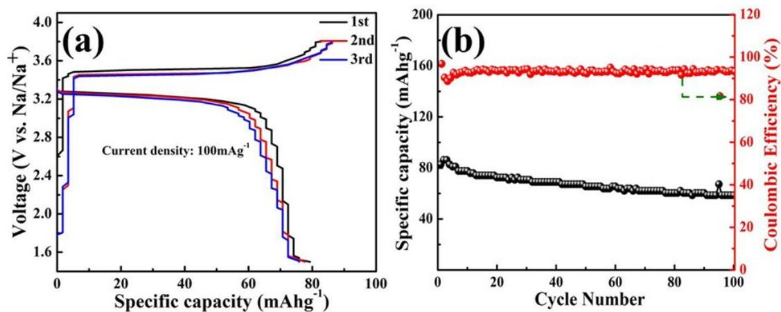
Fig. S16. Discharge-charge profiles of the  $\text{Na}_3\text{V}_2(\text{PO}_4)_3/\text{C}$  electrode at first three cycles with a potentials windows of 1.5 ~ 3.8 V at 100 mA  $\text{g}^{-1}$ , (b) Cycling stability measurement of the  $\text{Na}_3\text{V}_2(\text{PO}_4)_3/\text{C}$  electrode at 100 mA  $\text{g}^{-1}$ .
