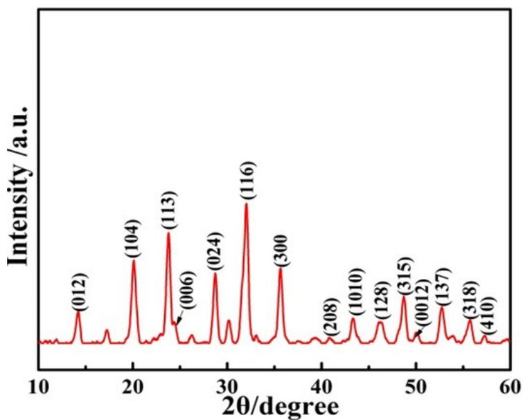
Fig. S15. XRD pattern of the  $\text{Na}_3\text{V}_2(\text{PO}_4)_3/\text{C}$  sample.
