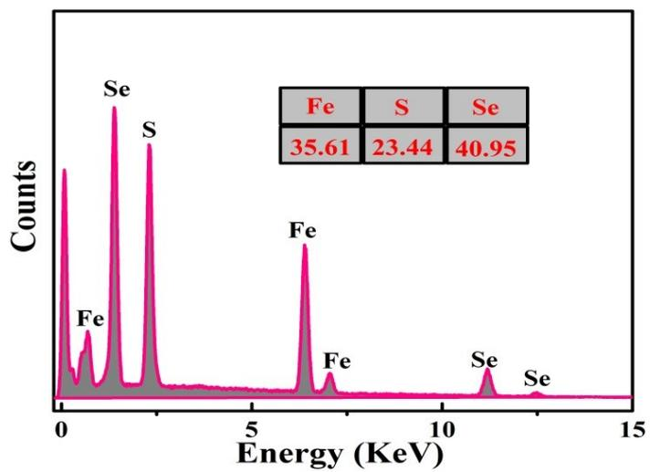
**Fig. S1.** EDS spectrum of FeS<sub>2</sub>@FeSe<sub>2</sub> microspheres.
