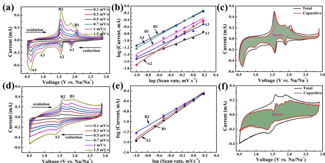
**Fig. S21.** CV curves of the electrode at different scan rates from 0.1 to 1.5  $\text{mV s}^{-1}$ , (a)  $\text{FeSe}_2$ , (d)  $\text{FeS}_2$ ;  $\text{Log}(i)$  vs.  $\text{log}(v)$  plots at each redox peak. (b)  $\text{FeSe}_2$ , (e)  $\text{FeS}_2$ ; Different CV curves of the  $\text{FeS}_2@\text{FeSe}_2$  electrode with the pseudocapacitive contribution to the total current shown by the shaded part at 1  $\text{mV s}^{-1}$ , (c)  $\text{FeSe}_2$ , (f)  $\text{FeS}_2$ .
