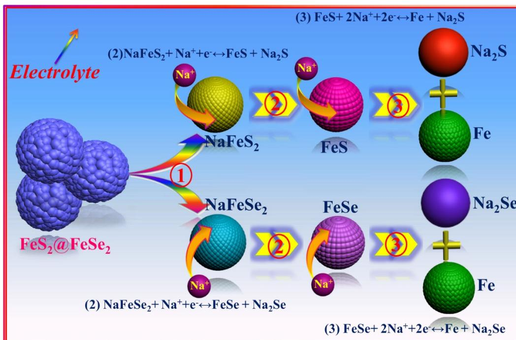
**Scheme S1.** Schematic illustration of reaction mechanism of  $\text{FeS}_2@FeSe_2$  electrode during the sodiation and desodiation process.
