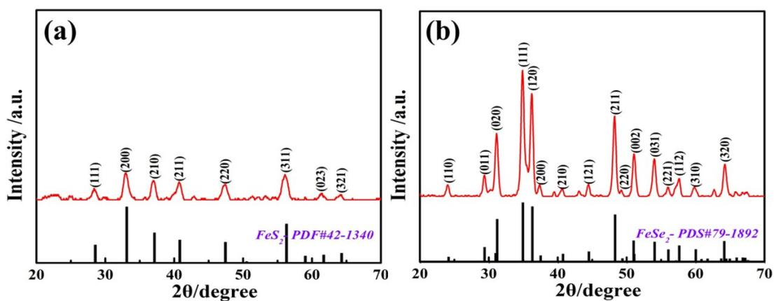
**Fig. S4.** (a, b) XRD pattern of FeS<sub>2</sub> microspheres and FeSe<sub>2</sub> nanoparticles, respectively.
