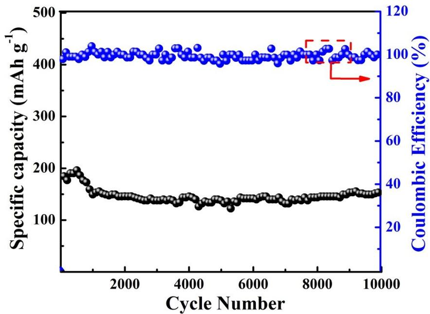
Fig.S11 Cycling stability test of the FeS<sub>2</sub>@FeSe<sub>2</sub> electrode at 7 A g<sup>-1</sup>.
