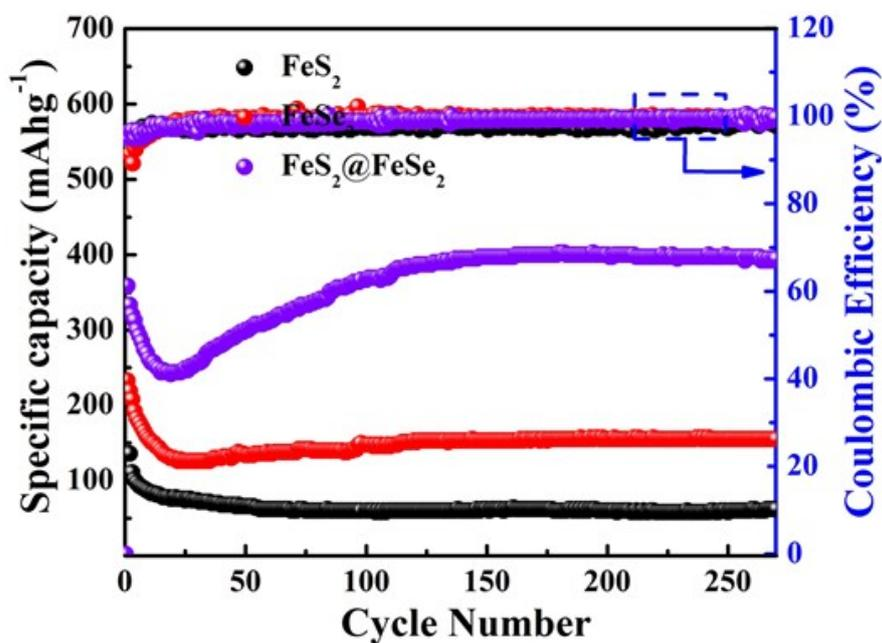
**Fig. S10.** The comparison of cycling performance for  $\text{FeS}_2@\text{FeSe}_2$ ,  $\text{FeS}_2$  and  $\text{FeSe}_2$  electrode with potential range from 0.5 to 2.9 V at  $1 \text{ A g}^{-1}$ .
