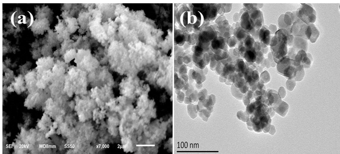
**Fig. S2.** SEM (a) and TEM (b) images of FeSe<sub>2</sub> nanoparticles, respectively.
