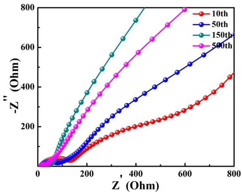
Fig. S12. Nyquist plots of FeS<sub>2</sub>@FeSe<sub>2</sub> electrode after different cycles.
