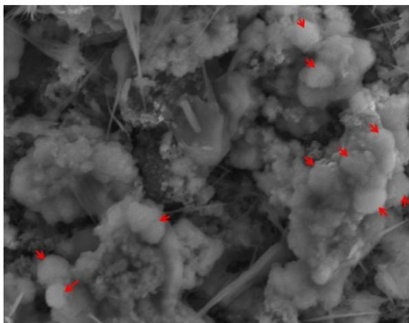
**Fig. S13** The SEM image of  $\text{FeS}_2@\text{FeSe}_2$  at  $1 \text{ A g}^{-1}$  after 200 cycles.
