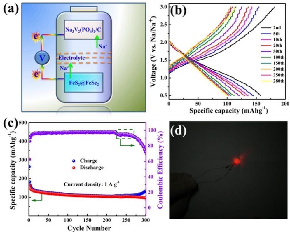
**Fig. S17.** Na<sub>3</sub>V<sub>2</sub>(PO<sub>4</sub>)<sub>3</sub>/C ~ FeS<sub>2</sub>@FeSe<sub>2</sub> full cell Configuration, (a) Schematic representation, (b) Discharge-charge profiles at different cycles, (c) Cycling performance at 1 A g<sup>-1</sup>, (d) Optical image.
