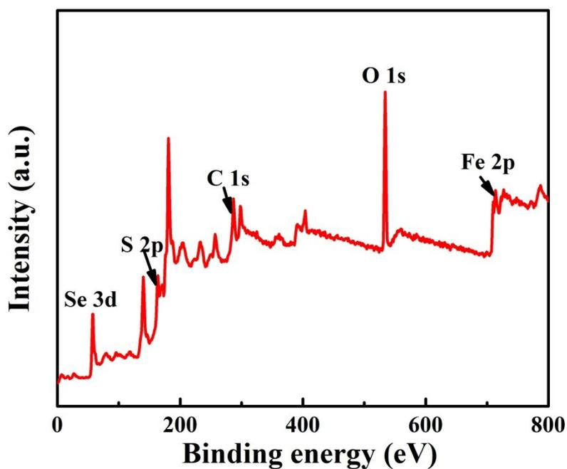
**Fig. S6.** XPS survey spectrum of FeS<sub>2</sub>@FeSe<sub>2</sub> microspheres.
