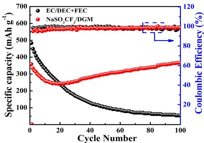
Fig. S7 The comparison of cycling performance for  $\text{FeS}_2@\text{FeSe}_2$  electrode with ether- and carbonate-based electrolyte at a voltage windows of 0.5-2.9 V at  $1 \text{ A g}^{-1}$ .
