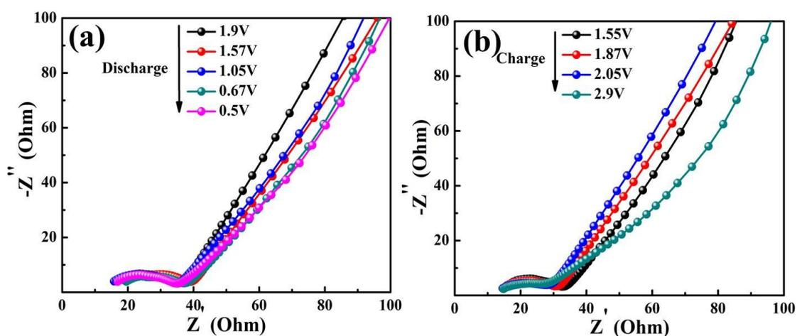
**Fig. S9.** (a, b) Nyquist plots of  $\text{FeS}_2@\text{FeSe}_2$  electrode at different discharged and charged state with the frequency range from 100 kHz to 0.01 Hz, respectively.
