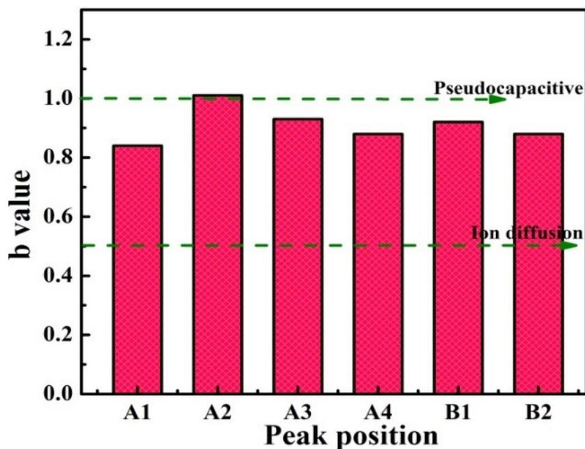
Fig. S19. Calculated b values at different peak position for FeS<sub>2</sub>@FeSe<sub>2</sub> electrode.
