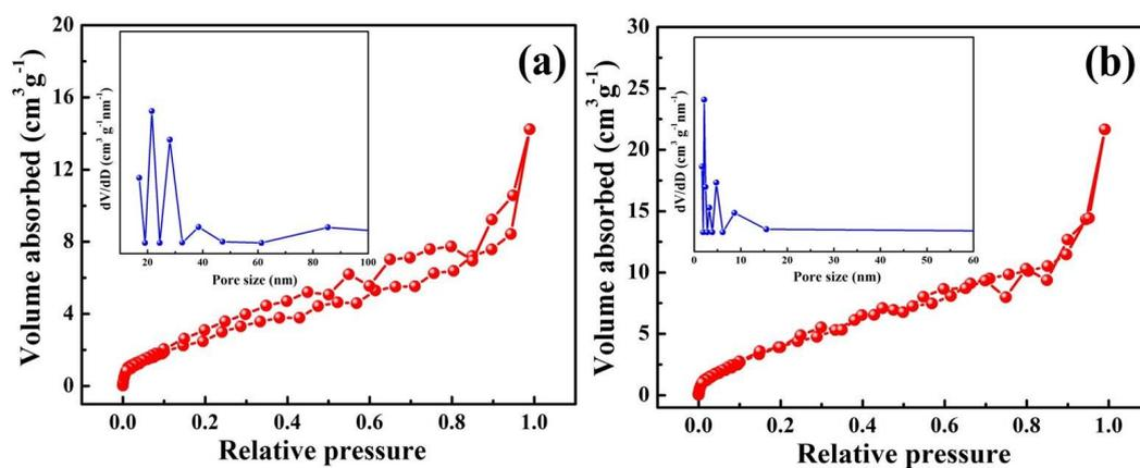
**Fig. S5.** (a, b) N<sub>2</sub> adsorption/desorption isotherms curves and BJH pore size distribution of FeS<sub>2</sub> microspheres and FeSe<sub>2</sub> nanoparticles, respectively.
