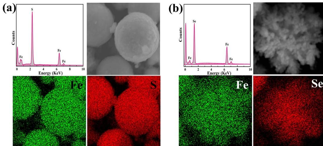
**Fig. S3.** (a, b) EDS spectra and elemental mapping of FeS<sub>2</sub> microspheres and FeSe<sub>2</sub> nanoparticles, respectively.
