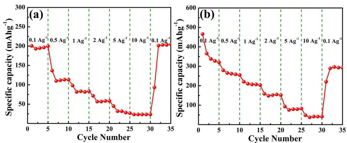
**Fig. S14.** (a, b) Rate capability measurement of plain  $\text{FeS}_2$  and  $\text{FeSe}_2$  electrode, respectively.
