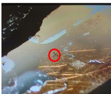
**Figure S16:** High resolution XPS spectra of the Cl 2p and Sn 3d regions at the point marked in the photograph (lower). The photograph shows the surface of device with the structure ITO|CsSnI<sub>3</sub>:SnCl<sub>2</sub>|C<sub>60</sub>|BCP|Al, in which the BCP|Al and part of the C<sub>60</sub> layer has been removed using carbon tape to expose the interfacial region between the perovskite film and C<sub>60</sub>.
