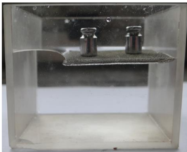
Fig. S31 Photograph of the coated nickel foam (about 0.4 g) with a loading of 4 g weights.
