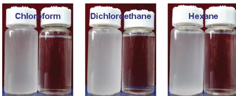
Fig. S32 Photographs of water-in-oil emulsions before and after emulsion separation.
