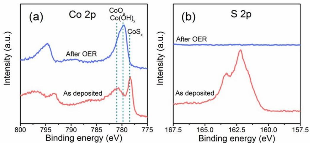
**Figure S10.** Comparison of the (a) Co 2p and (b) S 2p XPS spectra for the  $\text{Co}_9\text{S}_8/\text{CNT}$  catalyst as prepared and after OER.
