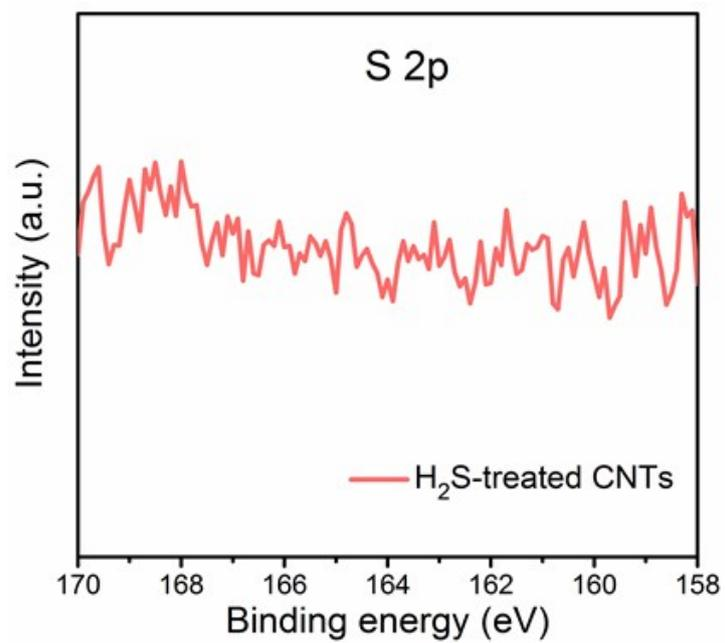
**Figure S6.** XPS S 2p spectrum of H<sub>2</sub>S-treated CNTs. The H<sub>2</sub>S treatment was performed following the same deposition conditions as for the ALD of Co<sub>9</sub>S<sub>8</sub> on CNTs except that no Co precursor was dosed (i.e. only dosing H<sub>2</sub>S).
