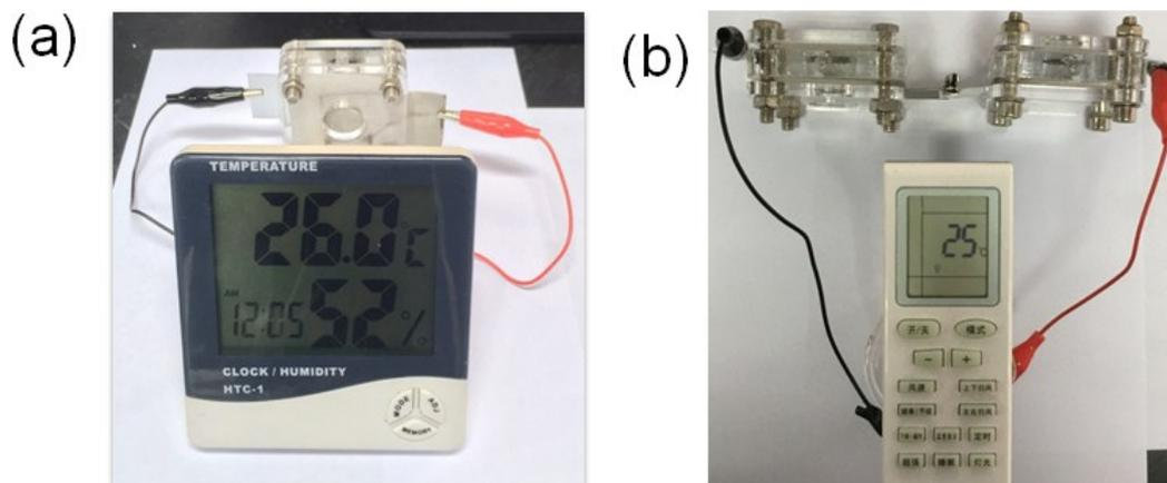
**Figure S13.** Photographs showing that the ALD-Co<sub>9</sub>S<sub>8</sub>/CNT-based aqueous Zn-air batteries can be used in replacement of (a) a 1.5 V coin cell to power a temperature/humidity monitor and (b) two AAA batteries to power a remote controller, respectively.
