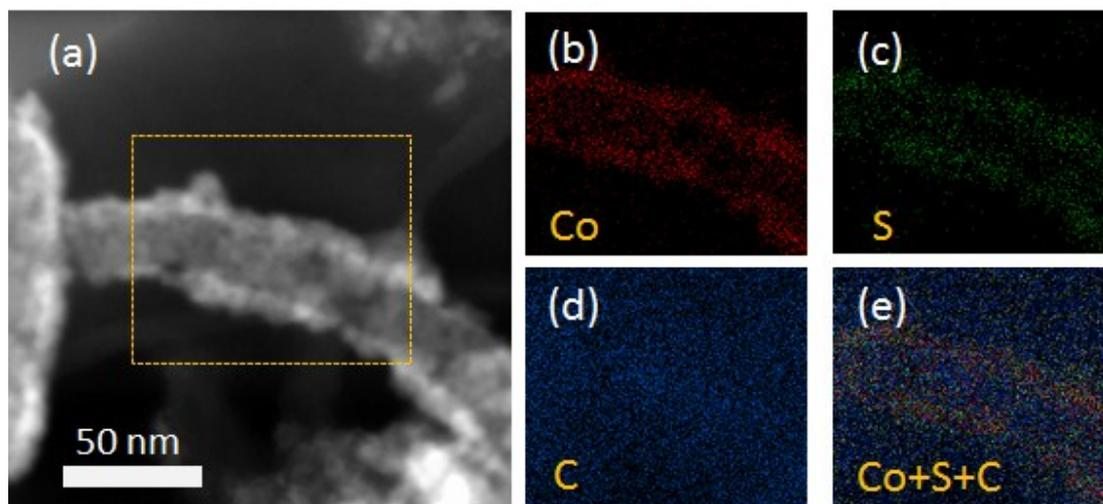
**Figure S2.** (a) STEM image of the ALD Co<sub>9</sub>S<sub>8</sub>/CNT sample, and the corresponding elemental maps of (b) Co, (c) S, (d) C, and (e) their overlay.
