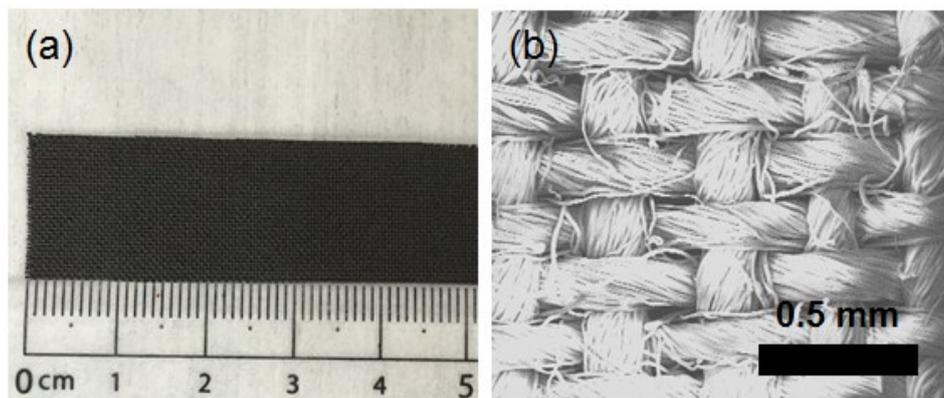
**Figure S9.** (a) Photograph and (b) SEM image of a piece of carbon cloth.
