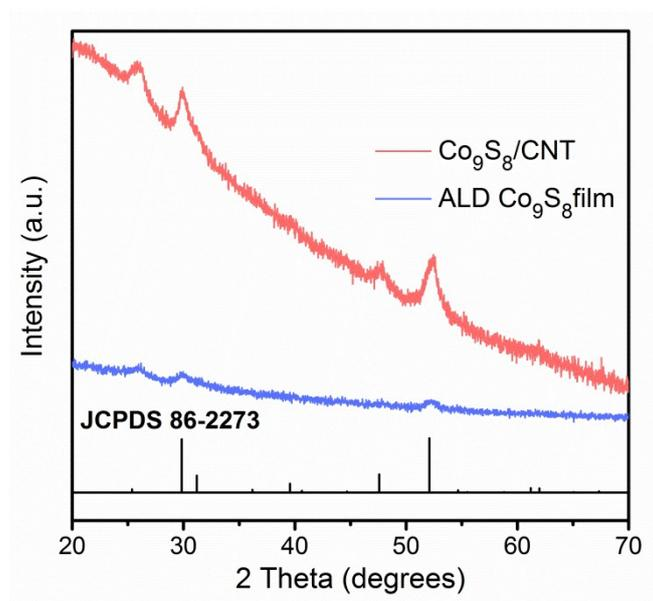
**Figure S3.** XRD patterns for the ALD Co<sub>9</sub>S<sub>8</sub>/CNT and ALD Co<sub>9</sub>S<sub>8</sub> thin film.
