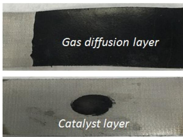
**Figure S15.** Photographs of an air cathode for the aqueous Zn-air battery. The cathode had a gas diffusion layer (upper) on one side of its stainless steel mesh, and the catalyst was loaded on the other side (lower).
