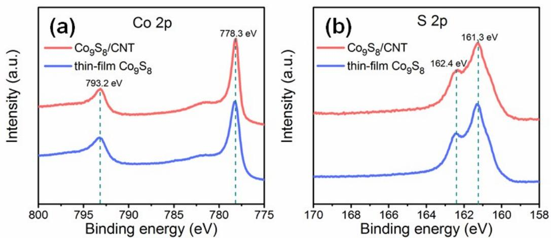
**Figure S5.** Comparison of the XPS spectra of (a) Co 2p and (b) S 2p peaks for the ALD Co<sub>9</sub>S<sub>8</sub>/CNT and ALD Co<sub>9</sub>S<sub>8</sub> thin film.
