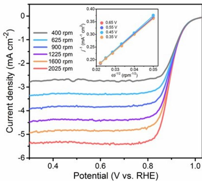
**Figure S12.** RDE voltammograms of the Pt/C catalyst with various rotation speeds for the electrode. The electrolyte was O<sub>2</sub>-saturated 0.1 mol/L KOH, and the voltage scan rate was 10 mV/s. The inset shows the corresponding Koutecky-Levich plots ( $j^{-1}$  vs.  $\omega^{-1/2}$ ).
