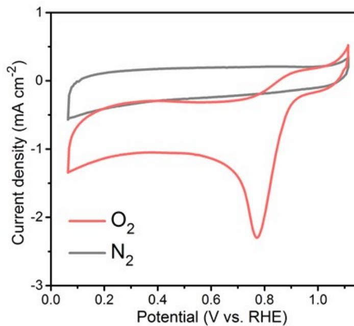
**Figure S11.** CV curves for the Co<sub>9</sub>S<sub>8</sub>/CNT electrocatalyst measured in O<sub>2</sub>- and N<sub>2</sub>-saturated 0.1 mol/L KOH, respectively. The scan rate was 100 mV/s.
