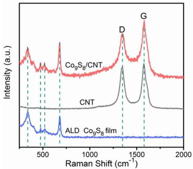
**Figure S4.** Raman spectra for the ALD Co<sub>9</sub>S<sub>8</sub>/CNT, uncoated bare CNTs, and ALD Co<sub>9</sub>S<sub>8</sub> thin film.
