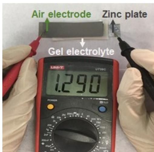
**Figure S14.** Photograph of a solid-state rechargeable Zn-air battery using the ALD  $\text{Co}_9\text{S}_8/\text{CNT}$  catalyst for the air electrode. The open-circuit voltage was measured as 1.290 V.
