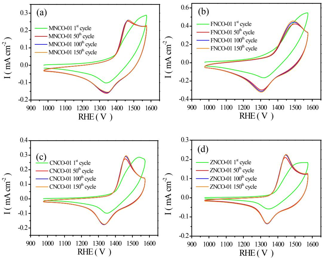
Fig. S3 Cyclic Voltammograms of the (a) MNCO-01, (b) FNCO-01, (c) CNCO-01, and (d) ZNCO-01 electrodes with 1<sup>st</sup>, 50<sup>th</sup>, 100<sup>th</sup>, and 150<sup>th</sup> cycle in 0.1 M KOH at 25  $\text{mV s}^{-1}$ .
