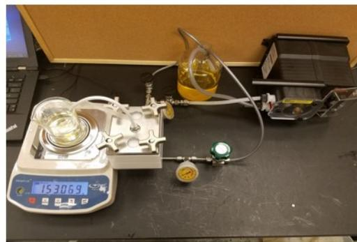
Figure S10: Experimental setup of water permeation and purification systems.
