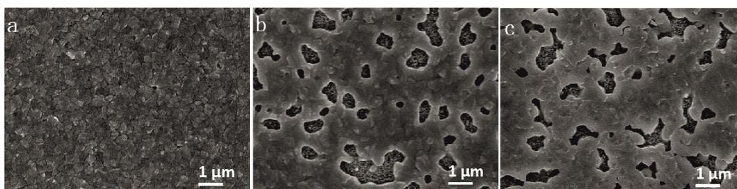
**Figure S2** Top-view SEM images of perovskite films washed with different temperature of toluene at (a) 0, (b) 15 and (c) 30 °C, respectively.
