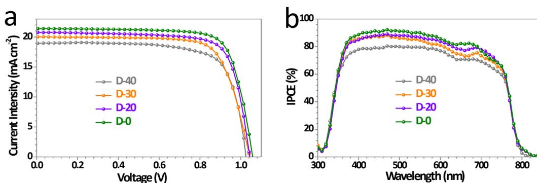
**Figure S1** (a) The current density–voltage curves of PSCs dripping with DE at different temperatures. (b) Internal photo-to-current efficiency measurement for the corresponding devices.
