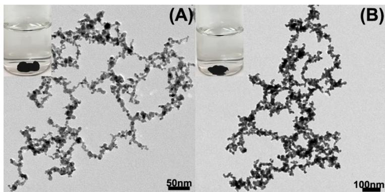
**Figure S6.** TEM and digital pictures of as-obtained Pt<sub>3</sub>Co (A) and Pt<sub>3</sub>Pb (B) metallic hydrogels.
