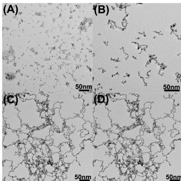
**Figure S3.** TEM images of AuPt<sub>5</sub>-25-DA metallic hydrogels obtained 0.5 min (A), 1 min (B), 5 min (C) and 10 min (D) after addition of NaBH<sub>4</sub> and DA.
