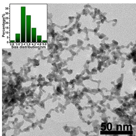
**Figure S4.** TEM image and size distribution (inset) of AuPt<sub>5</sub> metallic aerogels after CA test.
