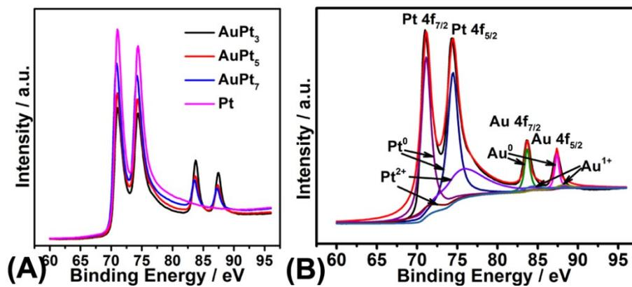
**Figure S1.** XPS of the Pt 4f and Au 4f of AuPt<sub>x</sub> and Pt metallic aerogels (A) and AuPt<sub>5</sub> metallic aerogels (B) synthesized without any capping agents at 60 °C.
