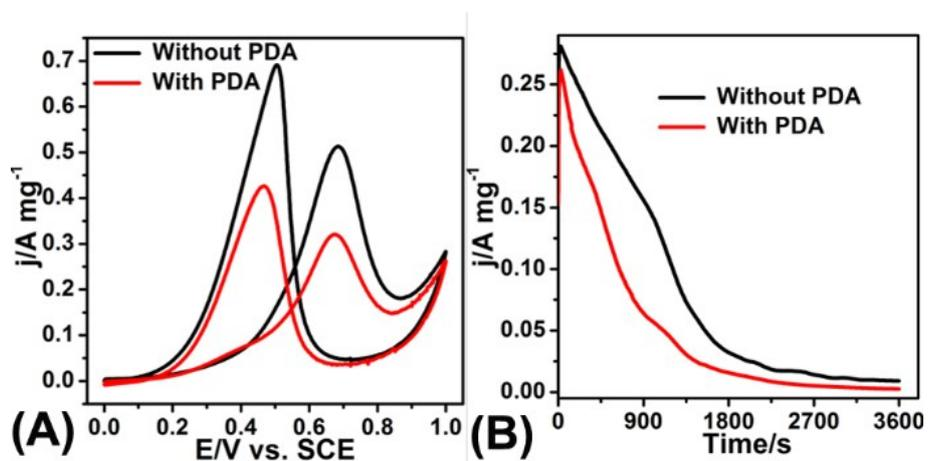
**Figure S5.** CV curves (A) and CA curves (B) of GCE modified by AuPt<sub>5</sub> and AuPt<sub>5</sub>-25-DA metallic aerogels measured in 1.0 M H<sub>2</sub>SO<sub>4</sub> solution in the presence of 1.0 M methanol. The scan rate of CV curves are 50 mV/s. CA curves are recorded at 0.55 V.
