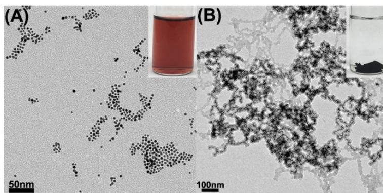
**Figure S2.** TEM images and digital pictures of the as-synthesized Au nanoparticles (A) and Au hydrogels (B).
