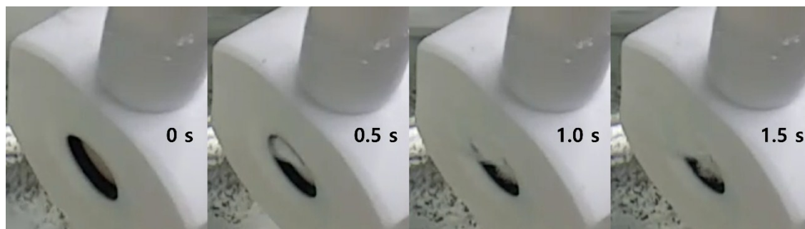
Figure S3. Pictures of electrode surface with time during electrodeposition process at -2 \text{ A cm}^{-2} for 2 s from aqueous solutions containing 0.1 \text{ M SnSO}_4 and 0.7 \text{ M H}_2\text{SO}_4 , and 120 \text{ g L}^{-1} acetone.
