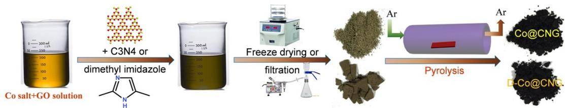
Figure 1. The preparative processes for Co@CNG and D-Co@CNG tri-functional electrocatalyst.
