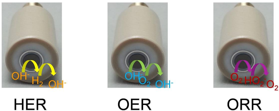
Figure 16. Schematic diagram of intermedia transform on the disk and ring during HER, OER and ORR.
