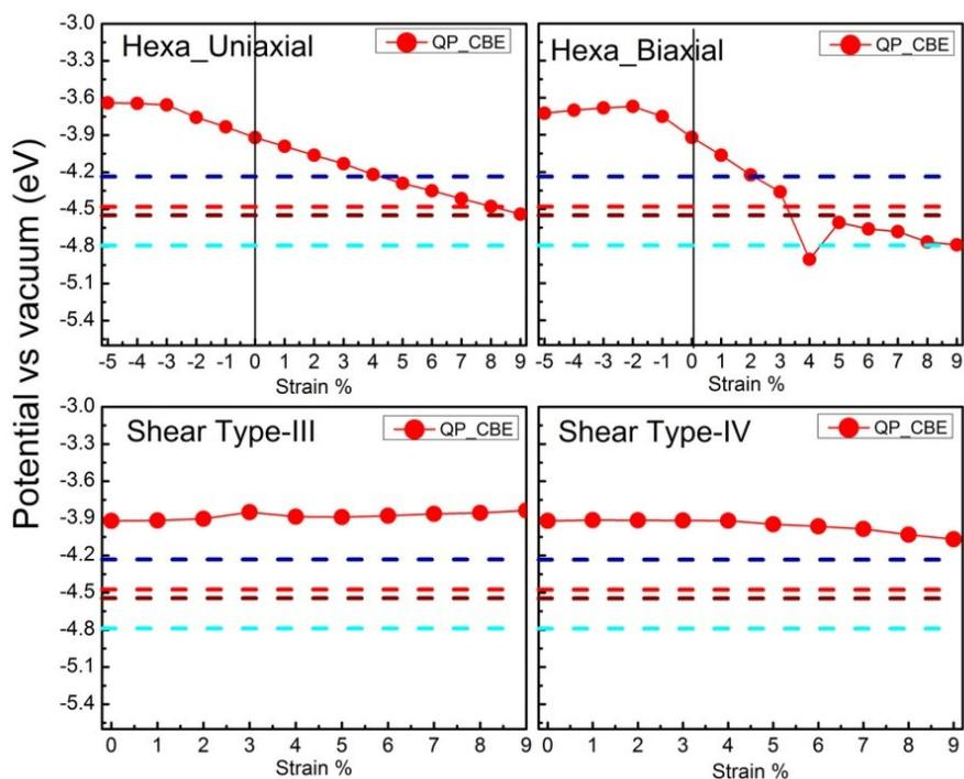
Figure S5 Variation in the valence and conduction band edges with the application of different types of strain in single layer MoS<sub>2</sub> studied in a supercell with hexagonal symmetry for CO<sub>2</sub> reduction
