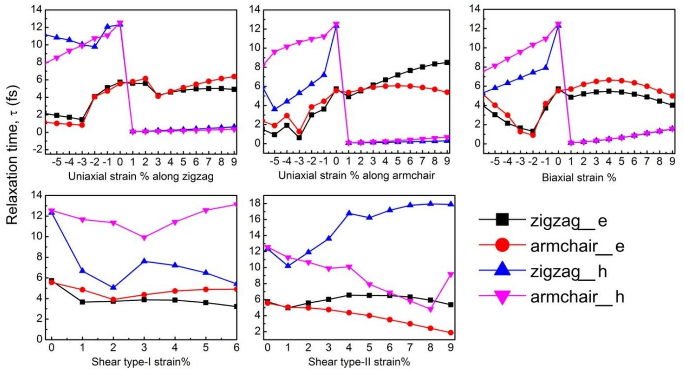
Figure S6 Variation in the relaxation time of the charge carriers along the zig-zag (zz) and arm-chair (ac) direction with mechanical strain of different types applied on to monolayer MoS<sub>2</sub> nanosheet
