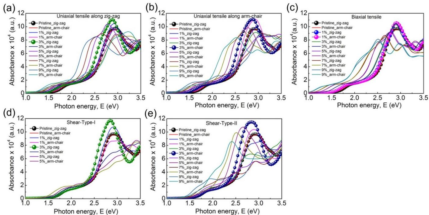
Figure S2 Variation in the absorbance spectra with different kinds of applied mechanical strain
