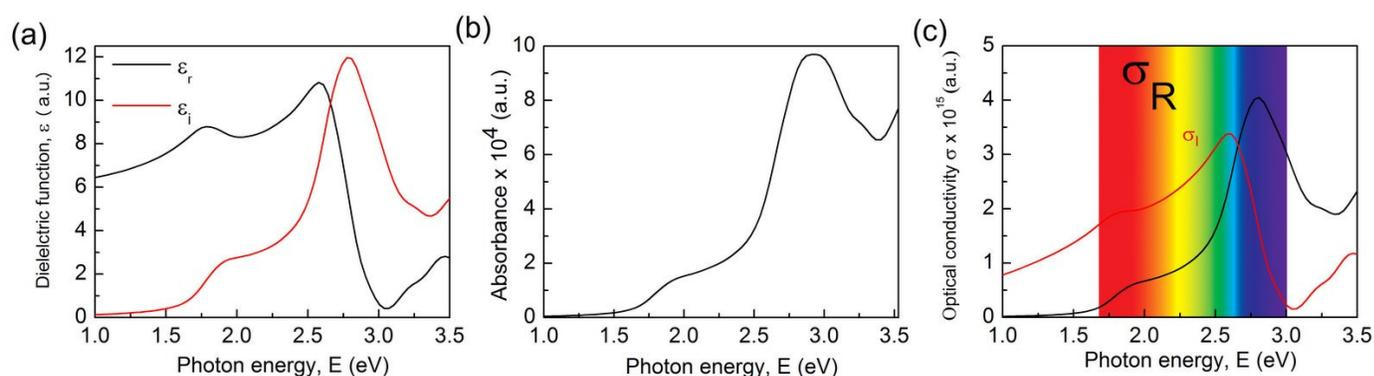
Figure S1 (a) Real  $\epsilon_1(\omega)$  and imaginary  $\epsilon_2(\omega)$  part of the frequency dependent dielectric function (b) Absorption spectra,  $\alpha_{abs}$ , (c) Real,  $\sigma_r(\omega)$  and imaginary,  $\sigma_i(\omega)$  part of optical conductivity in pristine unstrained single layer MoS<sub>2</sub>
