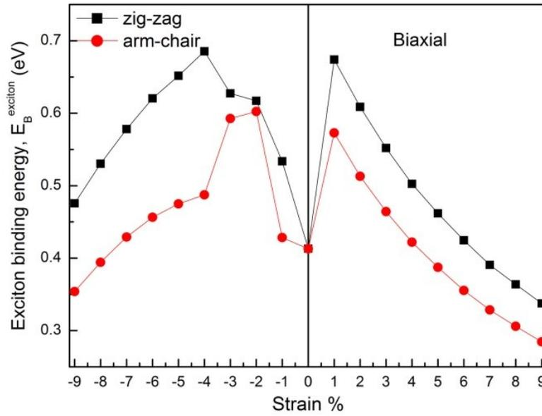
Figure S3 Variation in excitonic binding energy with biaxial strain applied on to ML-MoS<sub>2</sub> nanosheet
