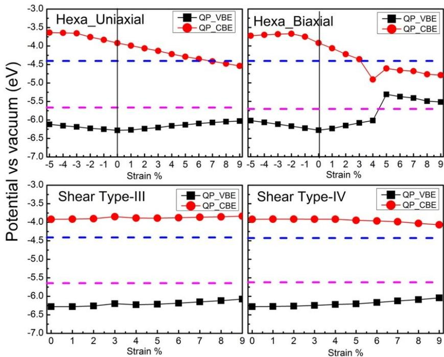
Figure S4 Variation in valence and conduction band edges with the application of different types of strain in monolayer MoS<sub>2</sub> studied in a supercell with hexagonal symmetry for solar water splitting
