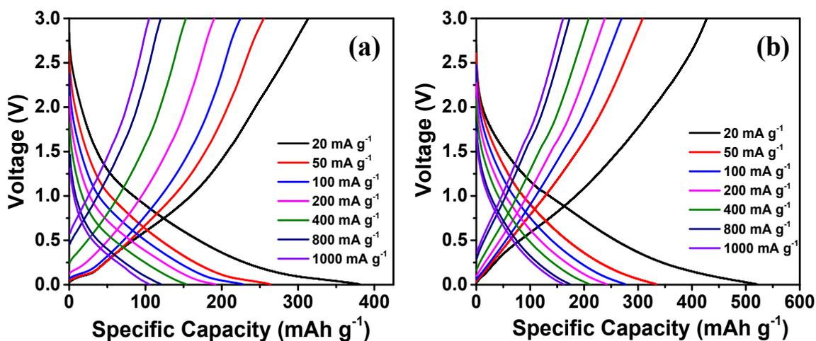
**Figure S3.** Charge-discharge curves at different rates for (a) HCS and (b) *N*-HCS tested against sodium.
