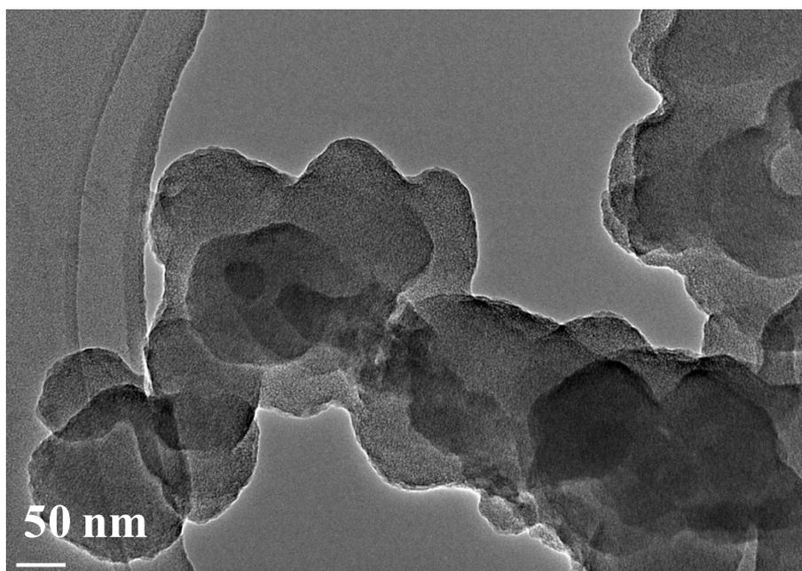
**Figure S1.** Transmission electron microscope image of HCS.
