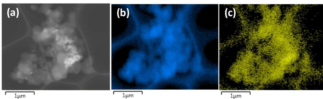
**Figure S2.** Energy dispersive X-ray mapping of HCS: (a) electron image, (b) carbon, and (c) oxygen.
