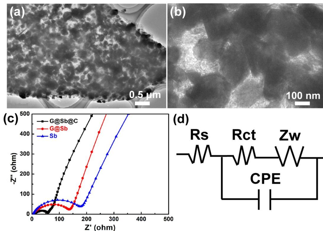
**Fig. S4.** (a and b) TEM images of the G@Sb@C composite after 50 cycles at a current rate of 0.1 A g<sup>-1</sup>; (c) Nyquist plots of the G@Sb@C, G@Sb and Sb electrodes after 50 cycles obtained by applying a sine wave with an amplitude of 5.0 mV over the frequency range 100 kHz to 0.01 Hz; (d) Equivalent circuit model of the studied system.
