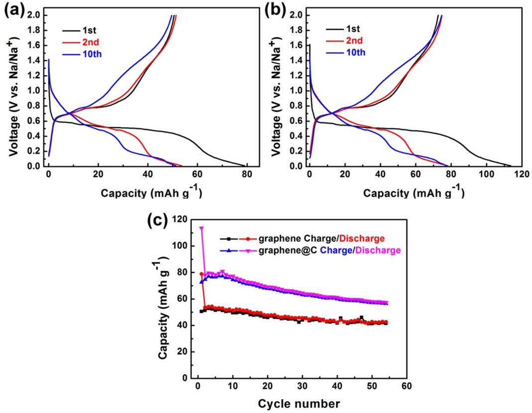
**Fig. S3.** Charge/discharge profiles of graphene (a) and graphene@C (b) electrodes at a current rate of 0.1 A g<sup>-1</sup> between 2.0 and 0.01 V for the 1st, 2nd and 10th cycles; (c) Cycling performances of graphene and graphene@C electrodes at a current rate of 0.1 A g<sup>-1</sup>.
