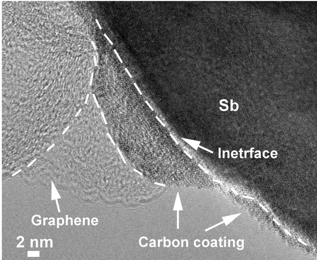
**Fig. S2.** HRTEM image of the G@Sb@C composite.
