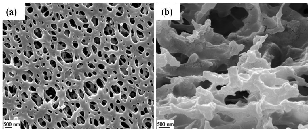
**Figure S1** Top view (a) and cross-sectional (b) SEM images of the support membrane in the present study.
