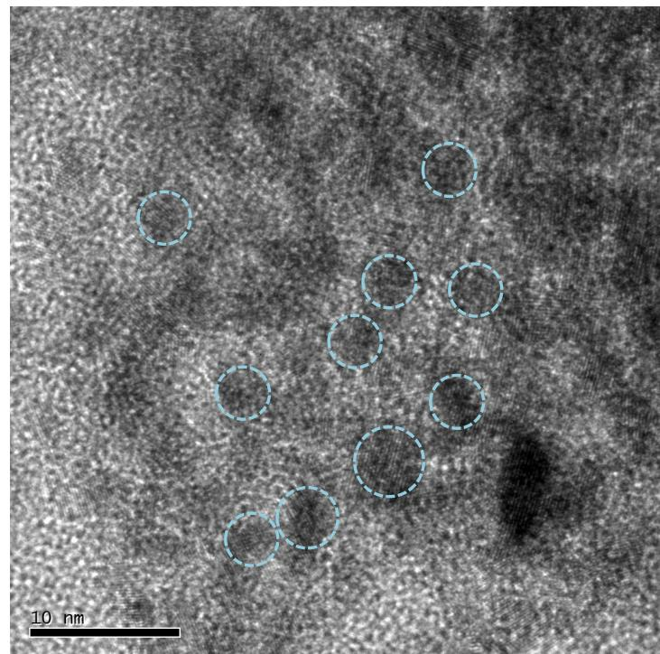
Figure S10 TEM image of Mo-600 after 1000 cycles CV measurement.
