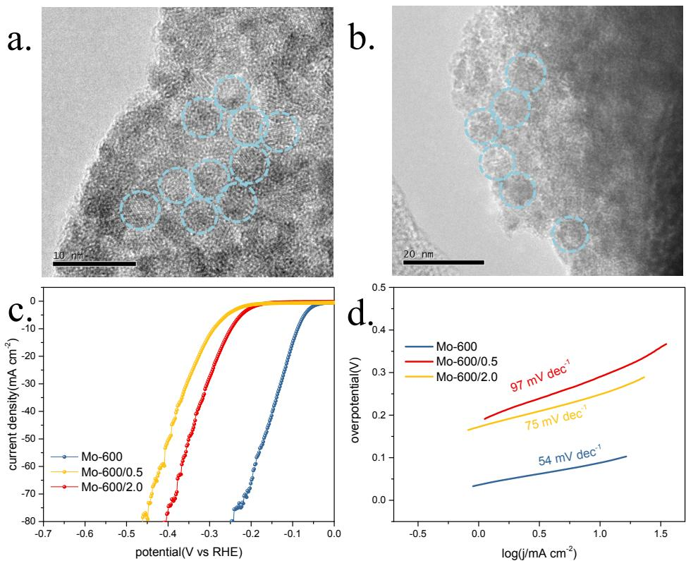
Figure S11 TEM image of (a) Mo-600/0.5 and (b) Mo-600/2.0; (c) Polarization curves and (d) Tafel slope.
