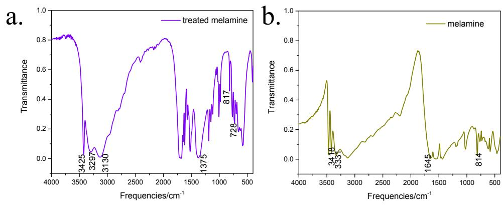
Figure S5 .FTIR results of (a)  $\text{HNO}_3$  pretreated melamine and (b) pure melamine
