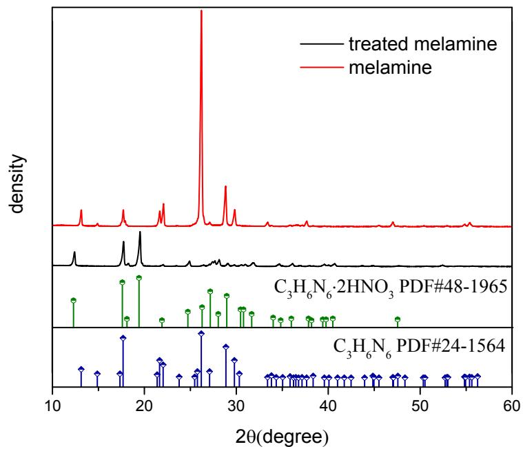
Figure S4.XRD results of pretreated melamine and pure melamine
