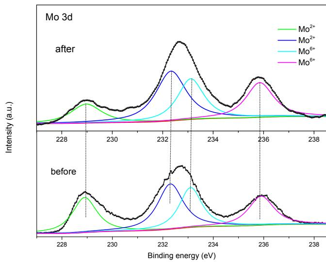
Figure S9 XPS spectra for Mo-600 before and after 1000 cycles CV measurement.
