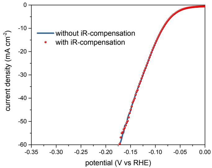
Figure S1 LSV curves of Mo-600 with and without iR compensation.
