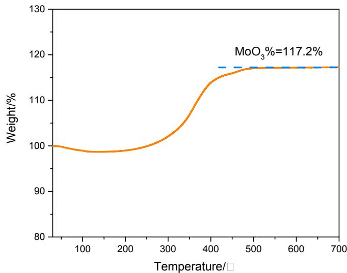
Figure S7. TGA curves of Mo-600 under air flow
