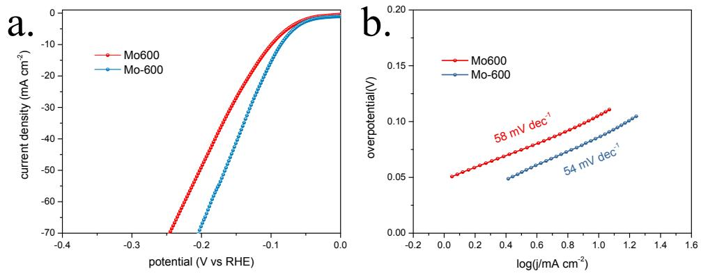
Figure S3. (a) Polarization curves of Mo-600 and Mo600 in 1 M KOH and corresponding (b) Tafel plots.
