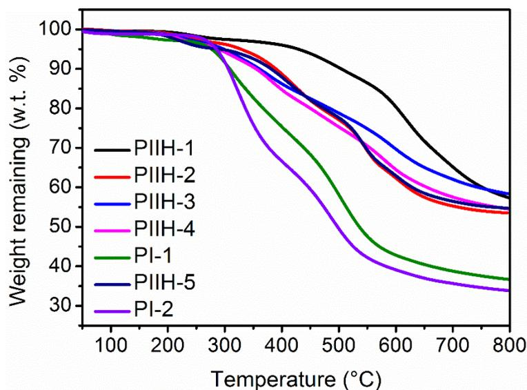
Fig. S10 TGA curves of the PI and PIIH thin films
