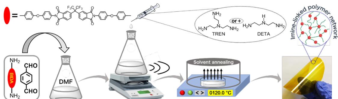
**Fig. S1** Schematic representation of the poly(imide imine) hybrid (PIIH) thin film fabrication
