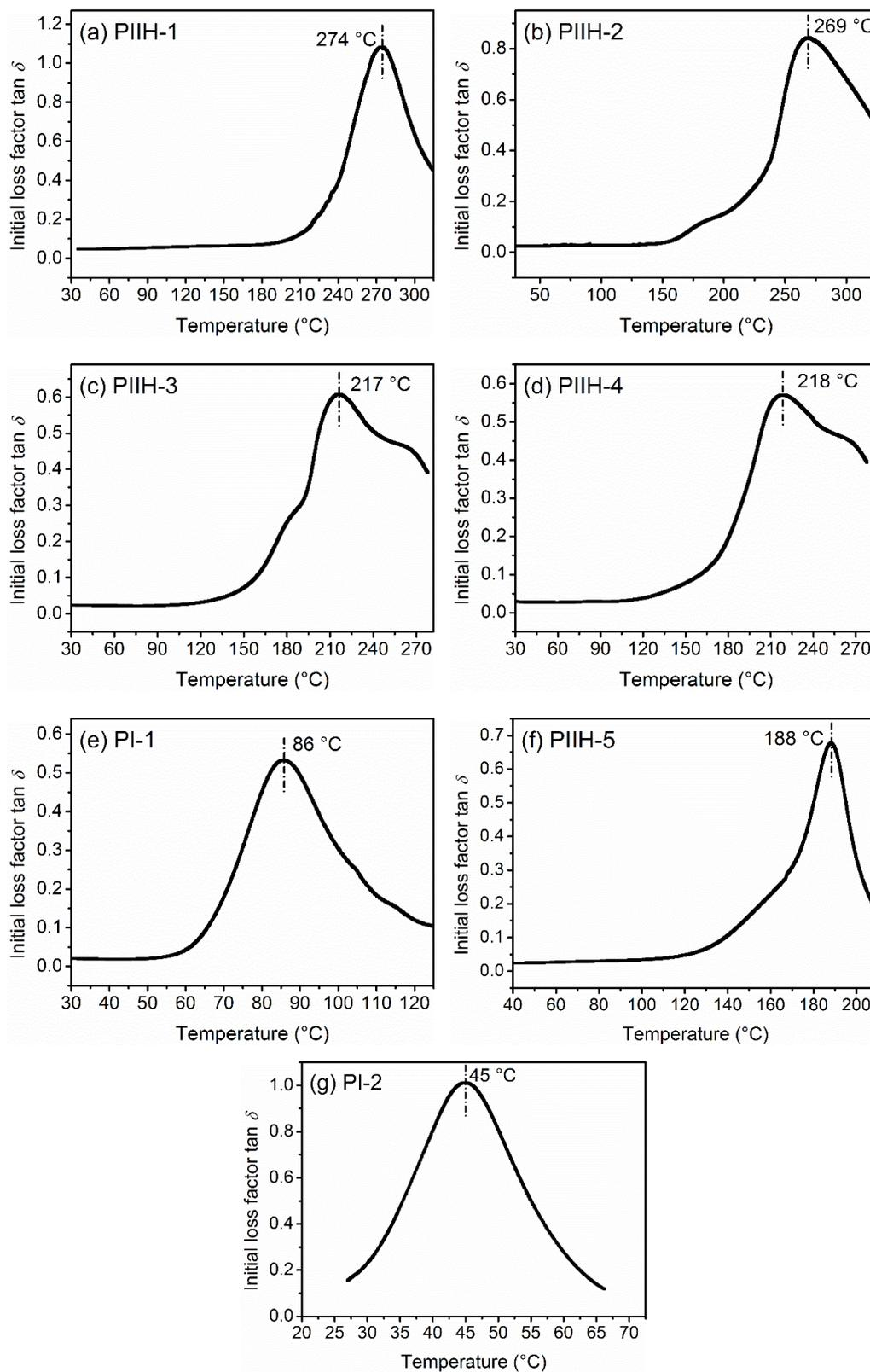
**Fig. S9** Initial loss factor  $\tan \delta$  curves of **PIIH-1** (a), **PIIH-2** (b), **PIIH-3** (c), **PIIH-4** (d), **PI-1** (e), **PIIH-5** (f) and **PI-2** (g)
