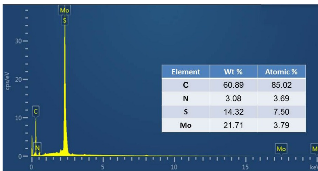
Fig. S8. EDS sum spectra of NMC-nanofilm@MoS 2 , Mo: S= 1: 1.98 (atomic ratio).
