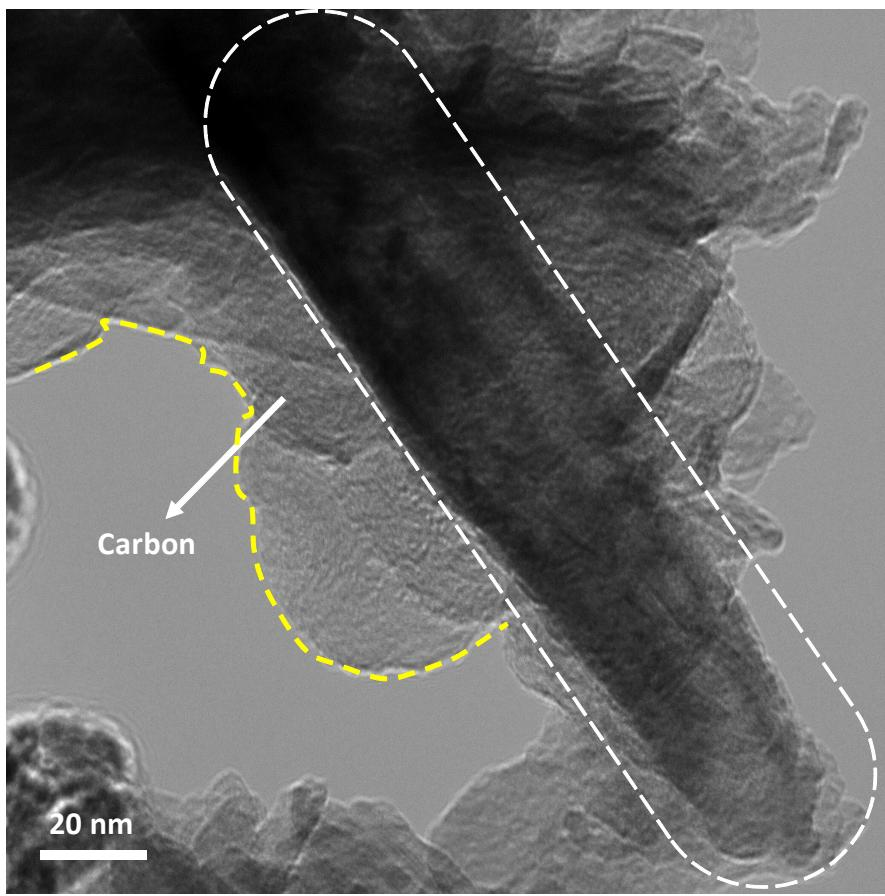
**Fig. S12** FE-TEM image of  $\beta$ -MnO<sub>2</sub> nanorod cathode after 200 cycles.
