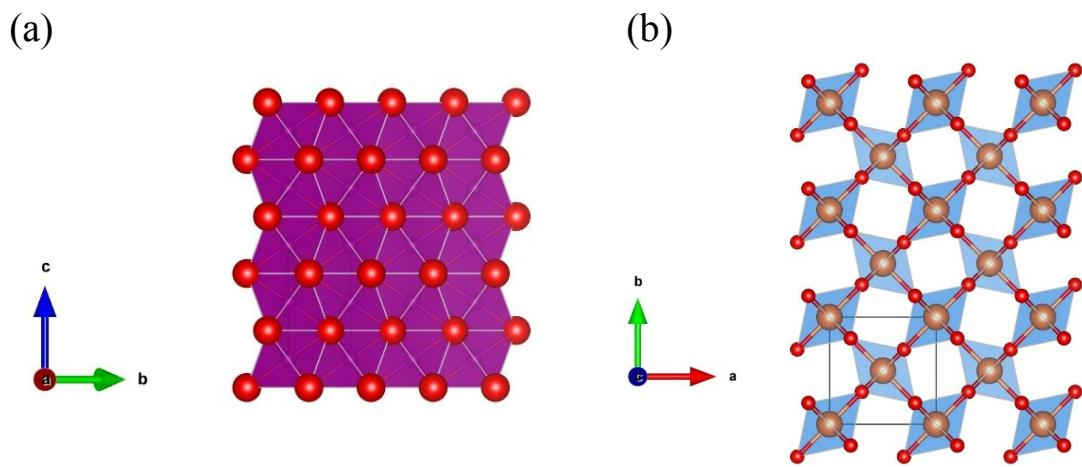
**Fig. S10** Comparison of (a)  $\epsilon$ -MnO<sub>2</sub> and (b)  $\beta$ -MnO<sub>2</sub> crystallographic structures.
