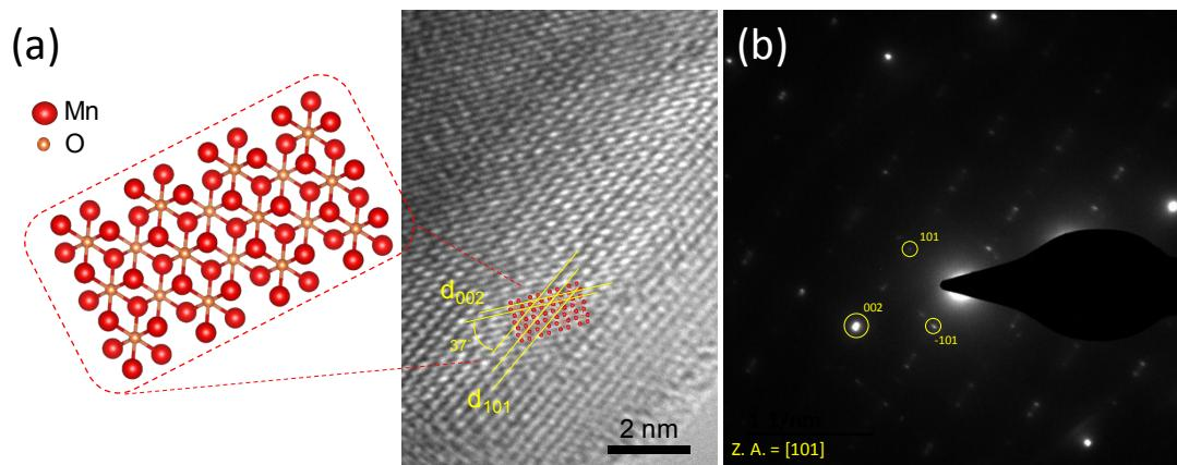
**Fig. S4** HR-TEM image and corresponding SAED pattern of the  $\beta$ -MnO<sub>2</sub> nanorod.
