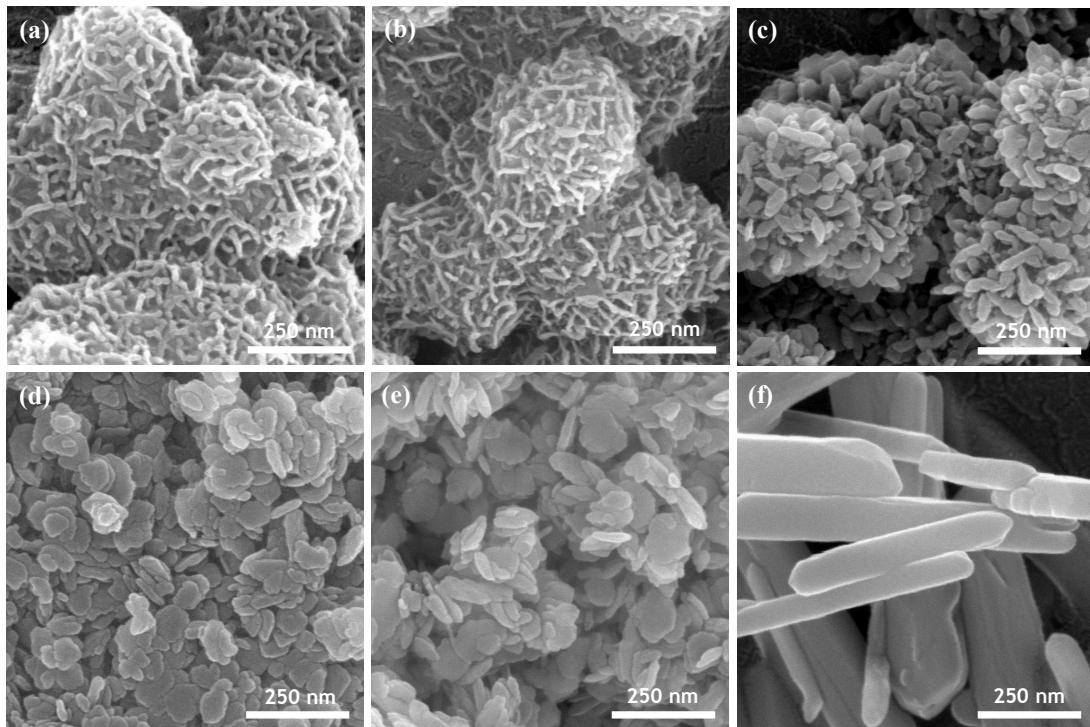
**Fig. S2** FE-SEM images of the sample prepared at various reaction temperatures: (a) 80, (b) 100, (c) 120, (d) 150, (e) 160, and (f) 180 °C.
