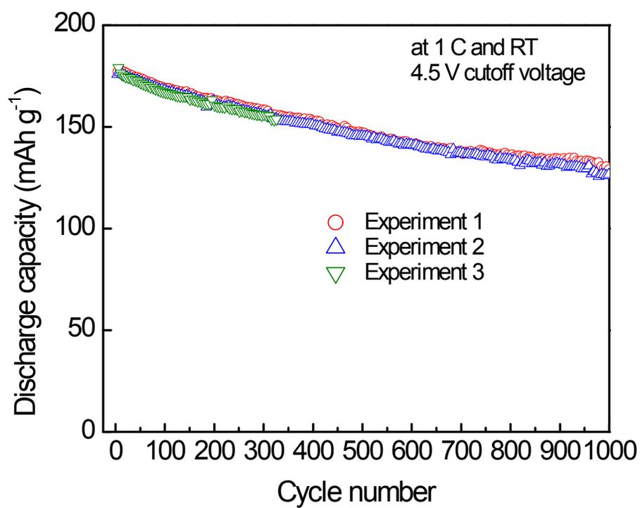
**Fig. S7.** Cycling performances of AOLCO electrodes prepared from three duplicated and independent experiments.
