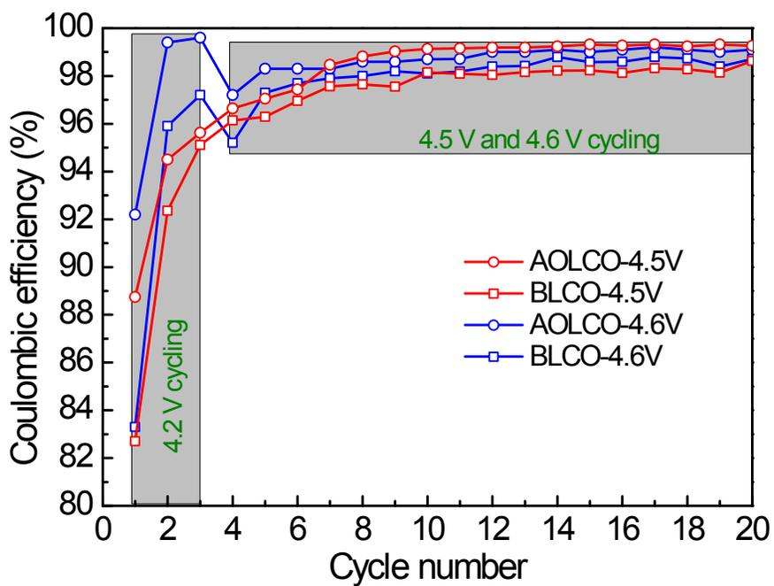
**Fig. S4.** Coulombic efficiency of BLCO and AOLCO electrodes during the first 20 cycles. The first 3 cycles were tested with 4.2 V cutoff voltage which is followed by cycling at higher voltages.
