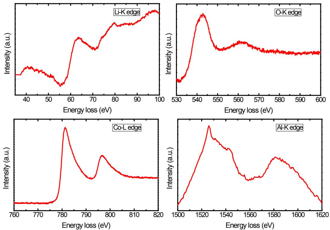
**Fig. S2.** EELS spectra of Li, O, Co and Al elements in the surface coating part of the AOLCO powders.
