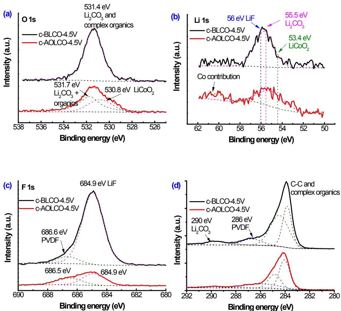
**Fig. S11.** XPS spectra analysis of the bare and coated electrodes cycled at 4.5 V cutoff for 500 cycles. (a) O 1s spectra, (b) Li 1s spectra and (c) F 1s spectra. All spectra were collected after 120 s of plasma etching.
