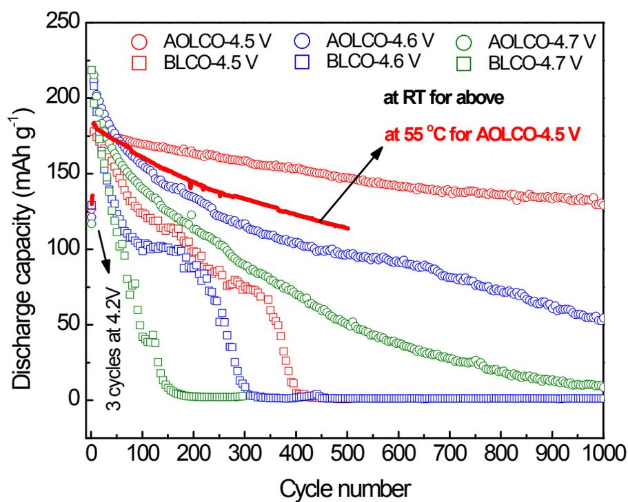
**Fig. S6.** Long-term cycling stability of BLCO and AOLCO electrodes at different cutoff voltages and temperatures. The current density is 1 C for all.
