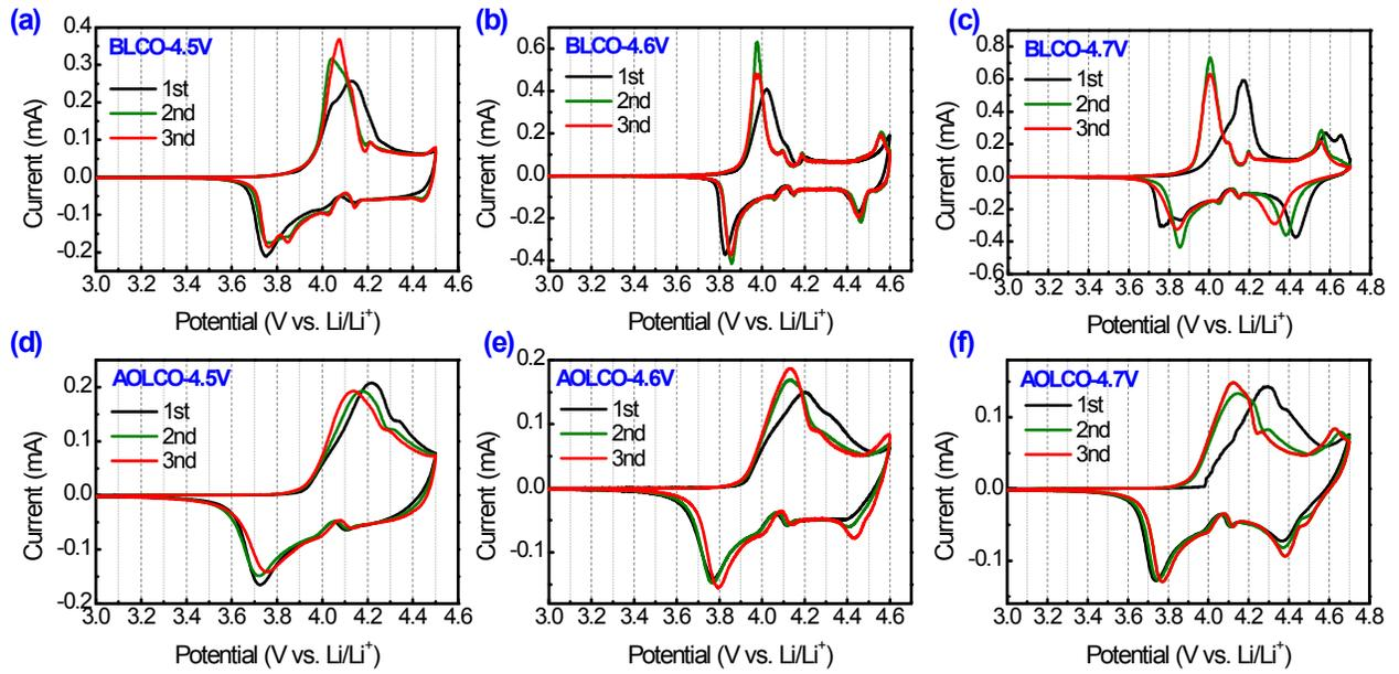
**Fig. S8.** CV profiles of the BLCO and AOLCO at different cutoff voltages during the first three cycles.
