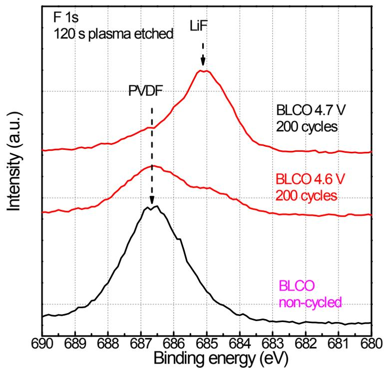
**Fig. S12.** Comparison of the F 1s spectra of BLCO before cycling and after 200 cycles at different cutoff voltages. All spectra were collected after 120 s of plasma etching.
