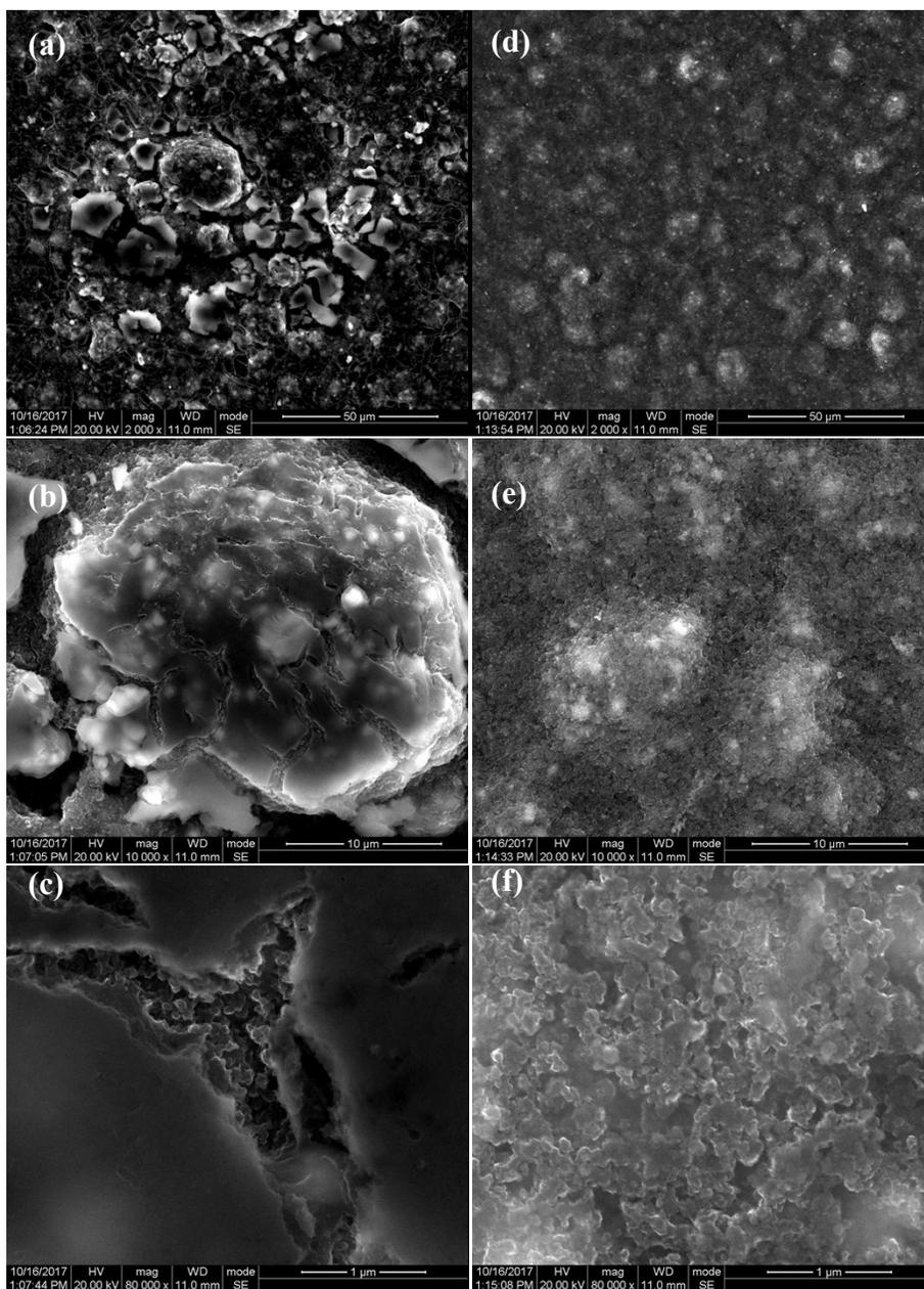
**Fig. S10.** FESEM images of bare LCO (a-c) and AOLCO (d-f) after cycling at 4.5 V for 500 cycles.
