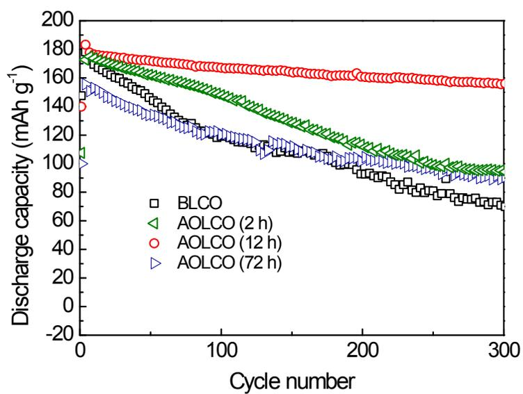
**Fig. S5.** Cycling stability of AOLCO electrodes with different coating time (stirring time in the solution) at 4.5 V cutoff, with current density of 1 C.
