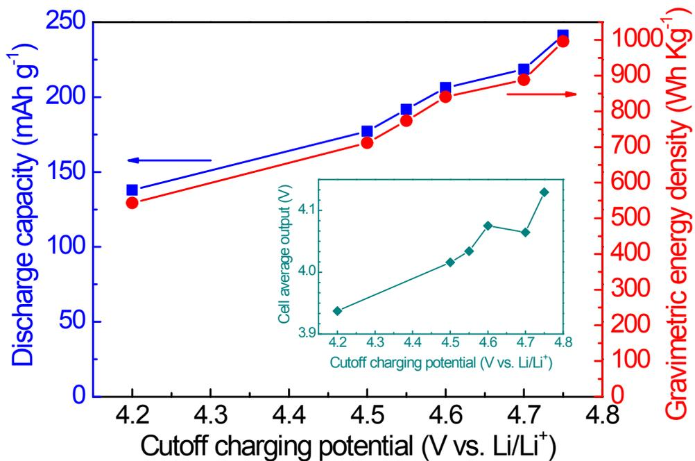
**Fig. S1.** Maximum specific capacity and gravimetric energy density of as-received commercial LiCoO<sub>2</sub> as a function of the cutoff charging potential cycled at 1 C. The inset shows the the dependence of the cell's average output voltage which is calculated by dividing the energy density by the discharge capacity.
