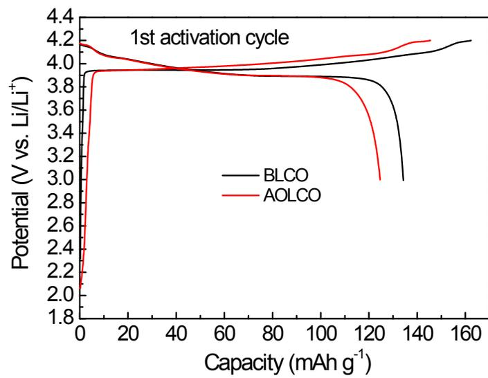
**Fig. S3.** Charge-discharge curves of BLCO and AOLCO during the 1<sup>st</sup> activation cycle within 3.0–4.2 V.
