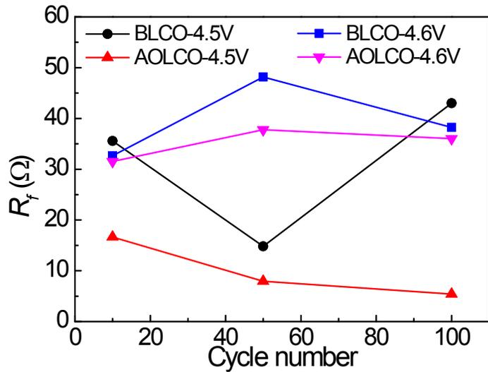
**Fig. S9.** Fitted surface layer resistance ( $R_f$ ) of BLCO and AOLCO after different number of cycles at 4.5 V and 4.6 V.
