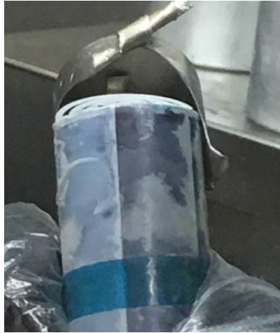
Fig. S7 Removing the steel shell.
