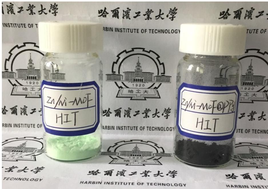
**Fig. S1.** Optical image of the Zn/Ni-MOF and Zn/Ni-MOF@PPy powder.
