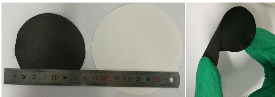
Fig. S1 (a) Digital photos of commercial filter paper and its carbonized paper; (b) Demonstration of mechanical flexibility of the carbon paper.
