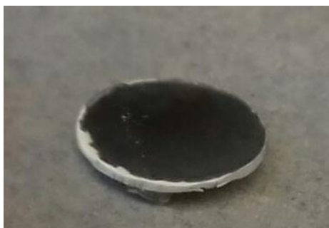
Supplementary Figure S1: Example of an extracted SSB pellet of a NCM-811 / \beta - \text{Li}_3\text{PS}_4 | \beta - \text{Li}_3\text{PS}_4 | Li-In battery, which was used for XPS depth profiling.
