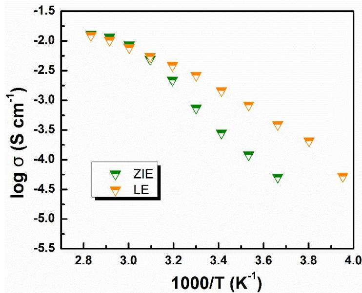
Fig. S4 Ionic Conductivity of ZIE and LE at various temperatures
