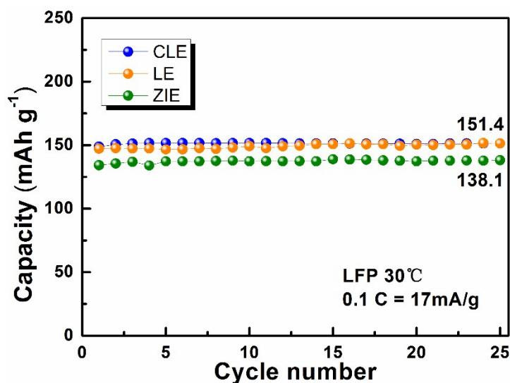
Fig. S7 Comparison of cycling performance of the Li/ LiFePO<sub>4</sub> batteries with ZIE, LE and conventional liquid electrolytes (CLE, 1 M LiPF<sub>6</sub> dissolved in ethyl carbonate (EC) and dimethyl carbonate (DMC) (1:1 by volume) )at a 0.1 C rate at 30 °C
