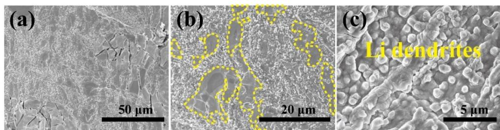
Fig. S9 SEM images of the surface of Li-metal anode in a Li/LE/LiFePO<sub>4</sub> battery after a few cycles
