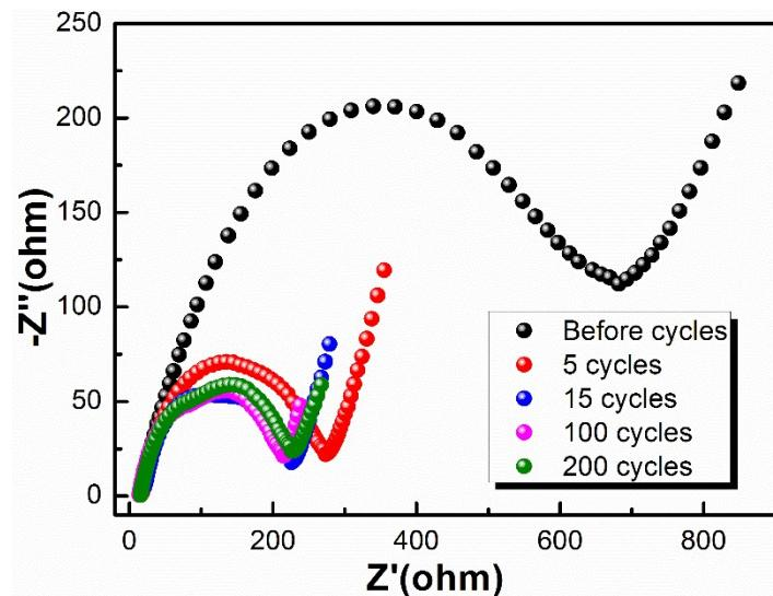
Fig. S8 EIS of the Li/ZIE/LiFePO<sub>4</sub> battery at different cycles
