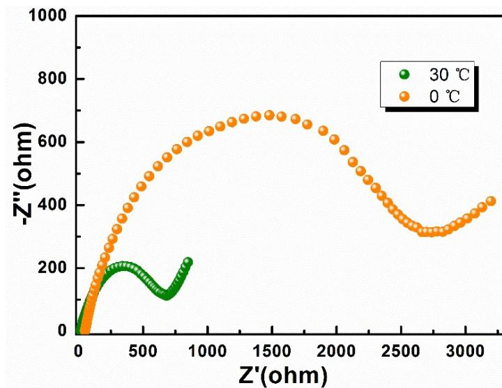
Fig. S6 EIS of the Li/ZIE/LiFePO<sub>4</sub> battery at 0 and 30 °C
