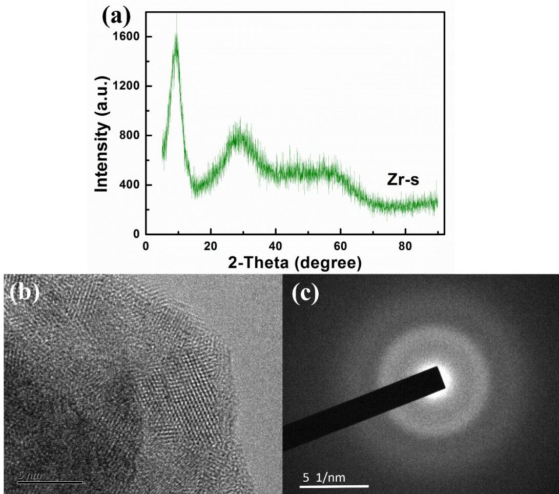
Fig. S3 (a) XRD pattern, (b) high resolution TEM and (c) electron diffraction images of Zr-s.
