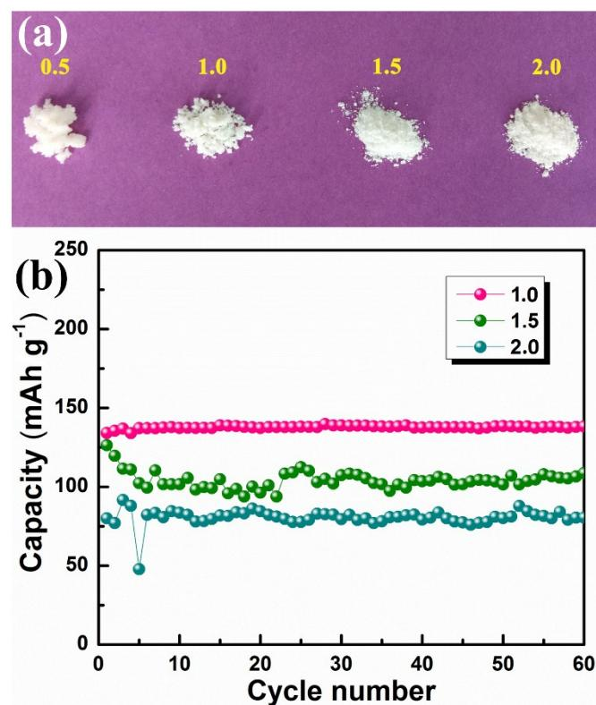
Fig. S2 (a) Digital photograph and (b) cycling performance of ZIEs with four different [EMI][TFSI]/ZrBO molar ratios (The cathodes, ZIE powders that were directly casted onto the cathodes and Li metal anodes were together pressed at 50 MPa to assemble 2025 coin cells. The ZIE with molar ratio of 0.5 can directly cause short circuit).
