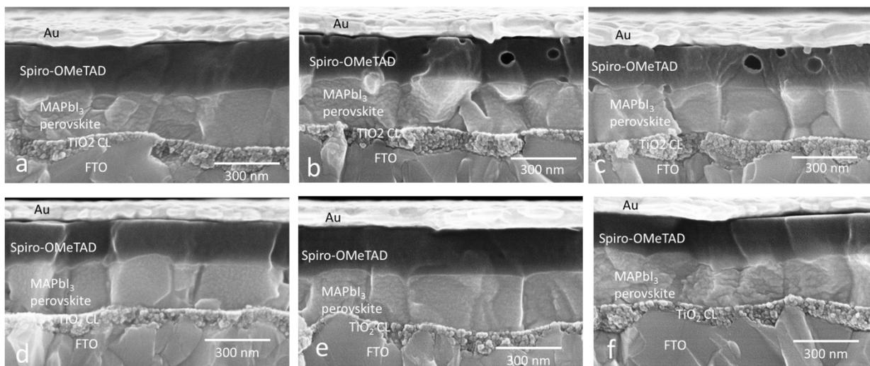
**Figure S5** Cross-sectional SEM micrographs of (a, b, c) planar MAPbI<sub>3</sub> solar cells heated (a-0 °C, b-100 °C and c-120 °C for 1 h) with Au electrode (FTO/c-TiO<sub>2</sub>/MAPbI<sub>3</sub>/Spiro-OMeTAD/Au) and (d, e, f) devices heated (d-0 °C, e-100 °C and f-120 °C for 1 h) before deposition of Au electrode (FTO/c-TiO<sub>2</sub>/MAPbI<sub>3</sub>/Spiro-OMeTAD).
