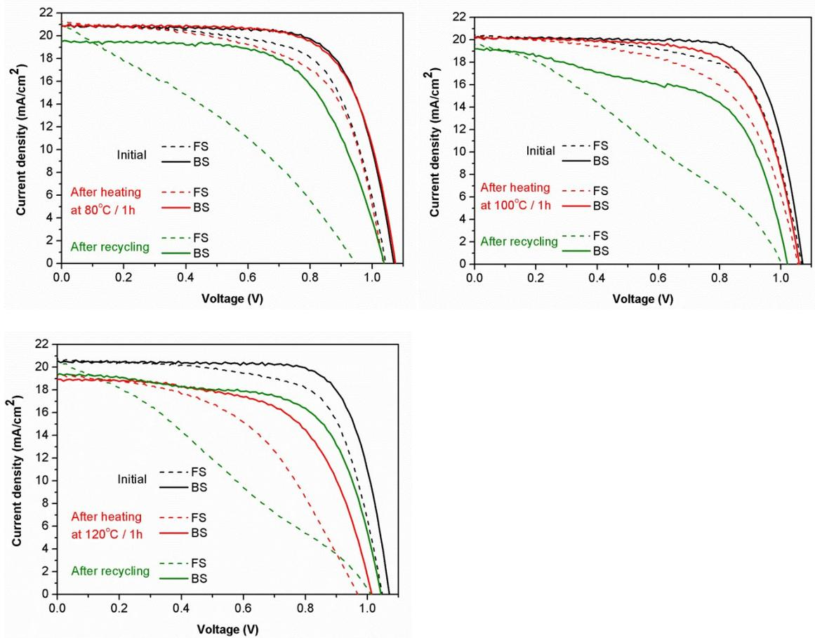
**Figure S8** Forward and backward J-V curves of planar perovskite solar cells before heating at different temperatures and after recycling
