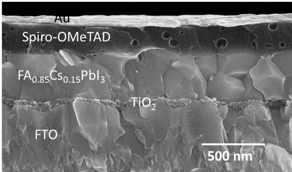
**Figure S10** Cross-sectional SEM micrographs of planar  $\text{FA}_{0.85}\text{Cs}_{0.15}\text{PbI}_3$  perovskite solar cells after heating at 100°C for 1 hour.
