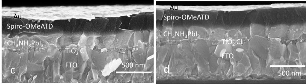
**Figure S9** Cross-sectional SEM micrographs of planar  $\text{MAPbI}_3$  perovskite solar cells recycled (with a fresh spiro-OMeTAD layer) after (a) without heating and heating at (b) 80, (c) 100 and (d) 120°C for 1 hour.
