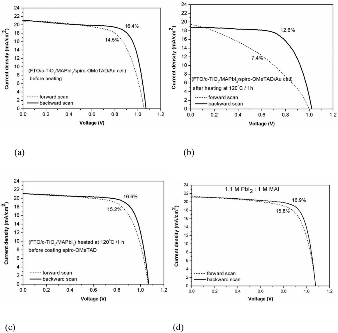
**Figure S4** J-V curves of planar MAPbI<sub>3</sub> perovskite solar cells (a) before (no PbI<sub>2</sub>) and (b) after (slight PbI<sub>2</sub>) heating at 120°C for 1 h, (c) with MAPbI<sub>3</sub> film heated at 120°C for 1 h (slight PbI<sub>2</sub>) before coating spiro-OMeTAD, (d) with slight excess of PbI<sub>2</sub> coming from solution (1.1 M PbI<sub>2</sub> : 1 M MAI)
