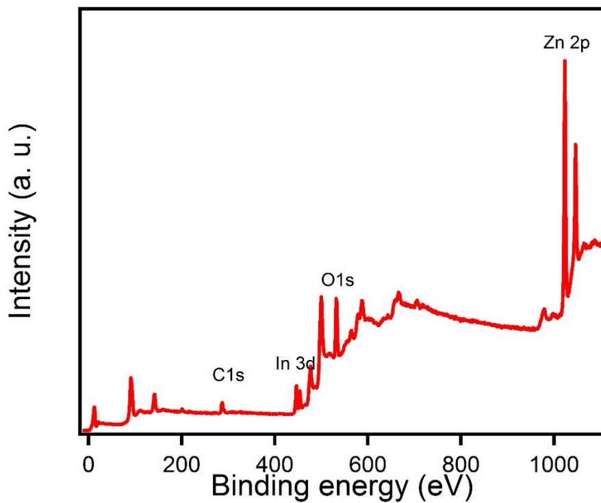
Fig. S1. The X-ray photoemission spectra for 5% IZO powders with full survey scan for binding energy 0-1100 eV.
