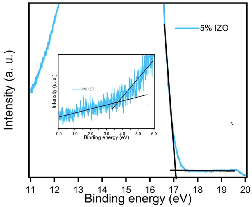
Fig. S2. The ultraviolet photoelectron spectroscopy (UPS) measurement for 5% IZO coated on FTO substrate to measure work function and valence band (inset).
