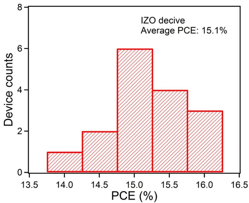
Fig. S6. The statistical data for 6.5 % IZO-based perovskite solar cells.
