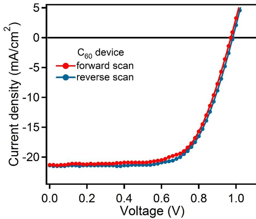
Fig. S9. The  $J$ - $V$  curve for C<sub>60</sub>-based perovskite solar cells with different scan direction from  $J_{sc}$  to  $V_{oc}$  (forward scan) and from  $V_{oc}$  to  $J_{sc}$  (reverse scan).
