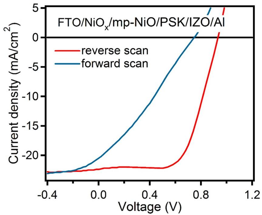
Fig. S8. The hysteresis effect on one of IZO-based perovskite solar cells with  $J$ - $V$  curve for forward scan and reverse scan.
