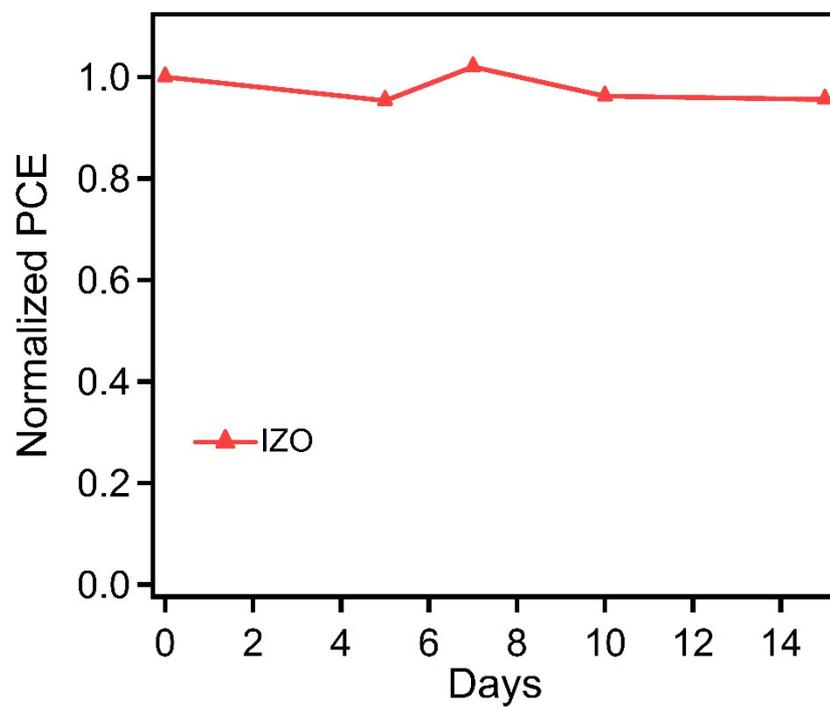
Fig. S10. The stability test with all inorganic interfaces device without encapsulation storage under ambient environment with relative humidity of  $25 \pm 5\%$  for several days.
