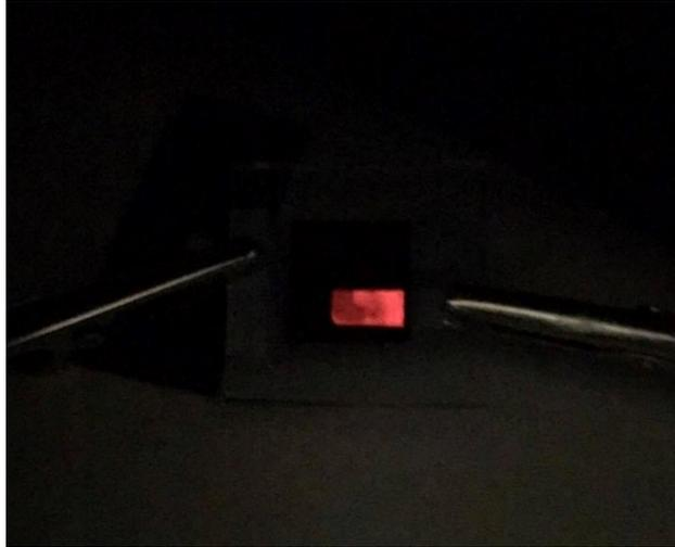
Fig. S11. The electroluminescence photo for IZO-based perovskite solar cell under forward bias in the dark.
