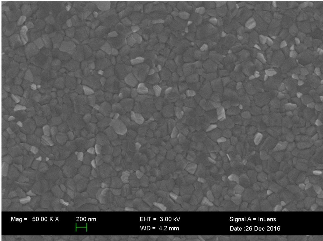
Fig. S4. The top-view SEM image for triple-cation perovskite coated on mesoporous NiO layer/NiO<sub>x</sub> thin.
