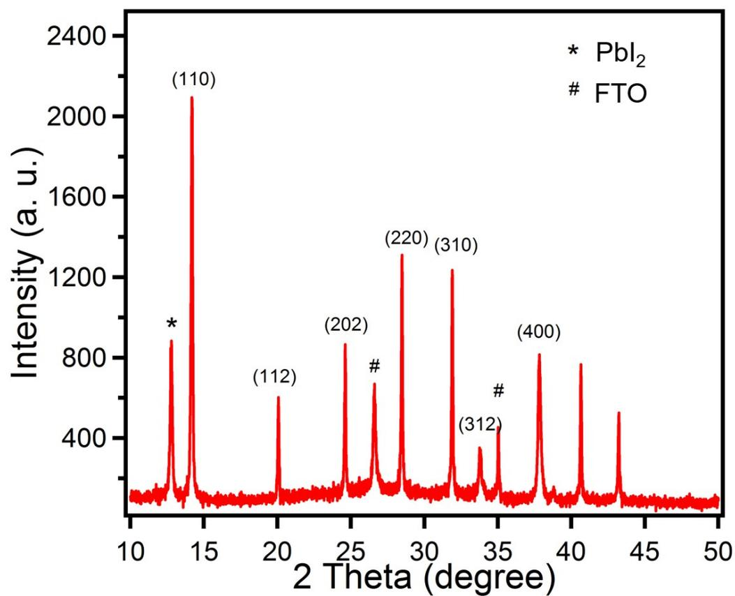
Fig. S5. The XRD pattern of triple-cation perovskite coated on mesoporous NiO layer/ $\text{NiO}_x$  thin.
