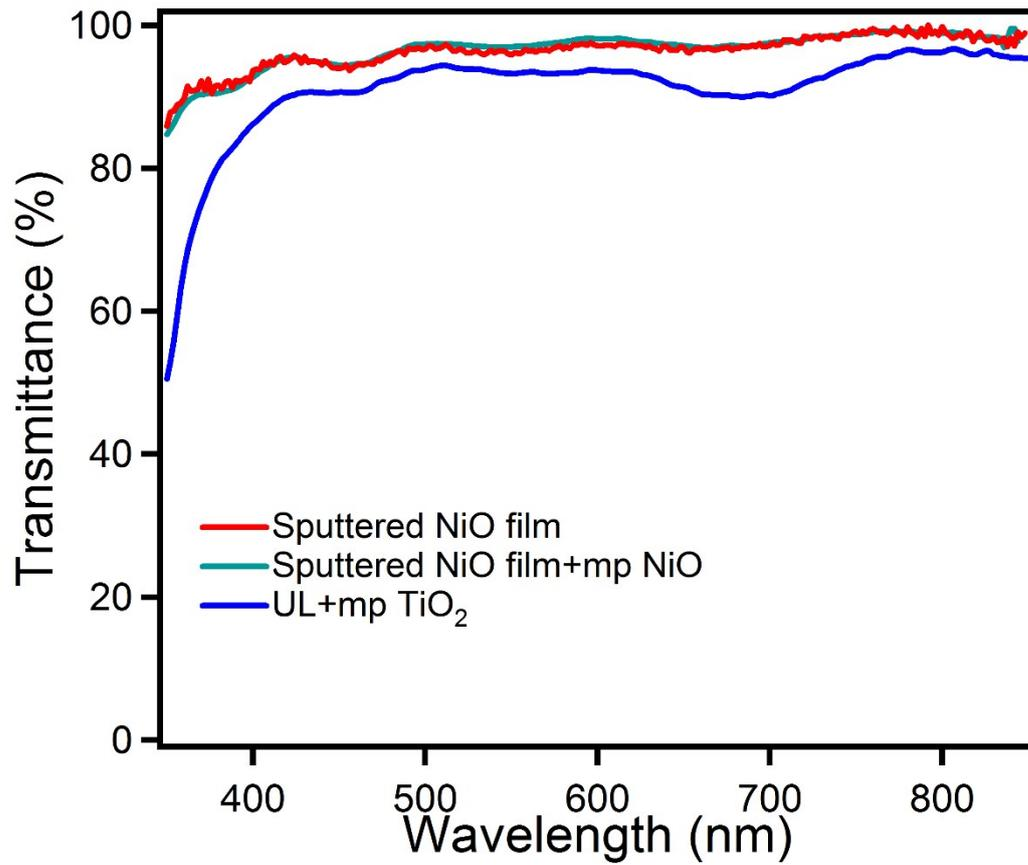
Fig. S3. The transmittance spectra of sputtered NiOx film, sputtered NiOx film + mesoporous NiO layer and mesoporous TiO<sub>2</sub> layer. (We used FTO substrate as baseline.)
