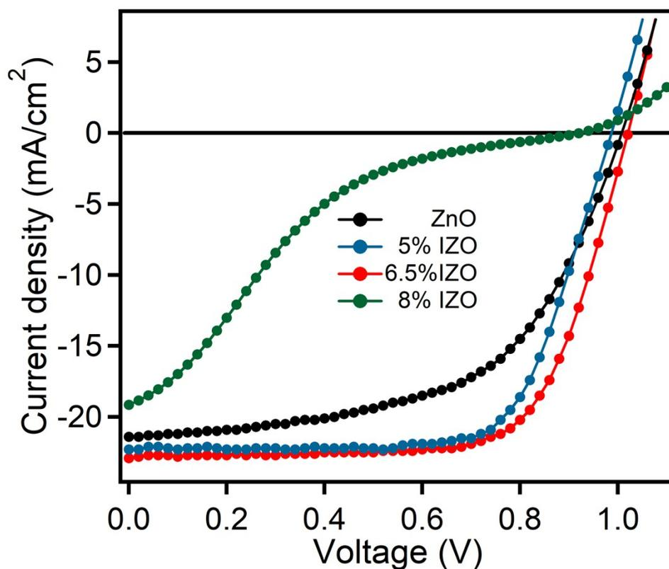
Figure S7. The J-V curve measurement based on different doping ratio of IZO device performance.
