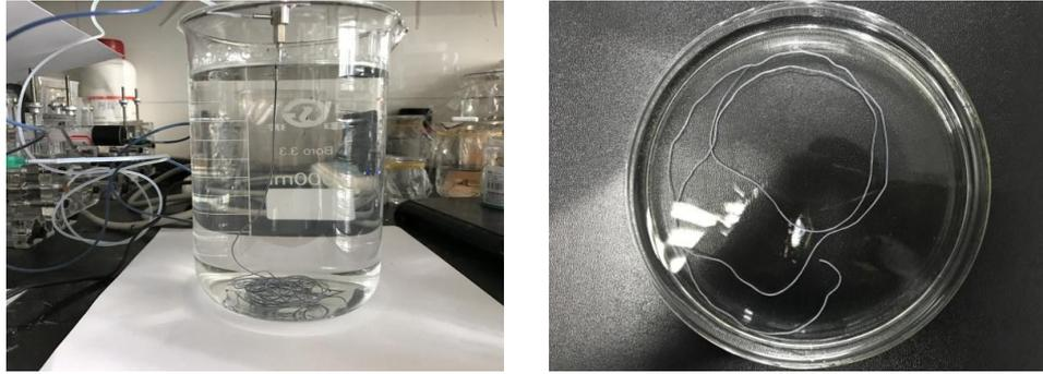
**Fig. S1** optical photos of (a) coaxial wet spinning process and (b) ternary coaxial fibers immersed in coagulation bath.
