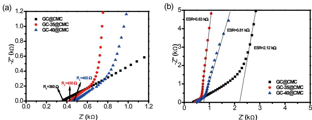
**Fig. S5** (a) EIS curves of GC@CMC, GCP-35@CMC and GCP-40@CMC in high frequency region, in which  $R_s$  is intrinsic ohmic resistance. (b) Equivalent series resistance  $R_{ESR}$  of GC@CMC, GCP-35@CMC and GCP-40@CMC.
