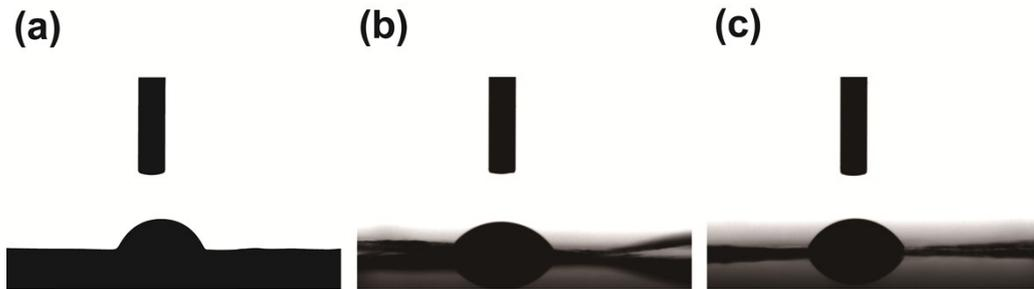
**Fig. S2** Contact angel test of (a) RGO film (b) GP-35 film (c) GCP-35 PEDOT:PSS film prepared by simply blade coating.
