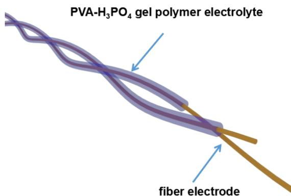
**Fig. S6** Assembly method of all-solid-state FSCs by using two twisted fibers as electrodes and PVA- $H_3PO_4$  gel as electrolytes.
